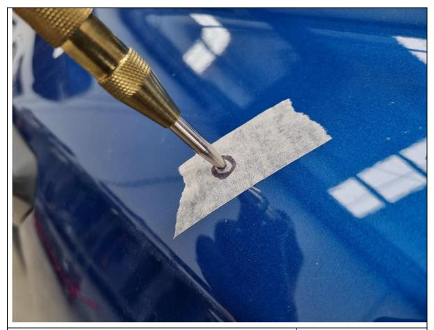
24. Use a centre punch on the centre of the 6x mounting hole locations on the quarter panel.
