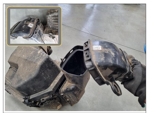
57. Use a flat head screwdriver to pry off the inlet duct off the airbox. Discard the inlet duct.
