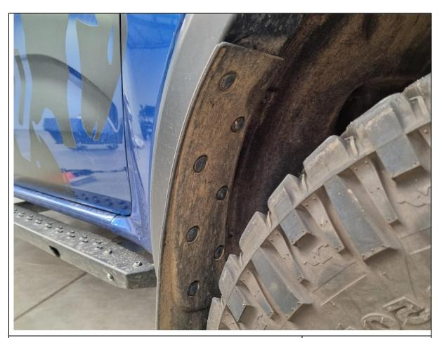
13. Remove the plastic push clips securing the mudflap to the wheel flare. Use a trim tool or flat blade screwdriver. Set the mud flap and clips aside for later.
