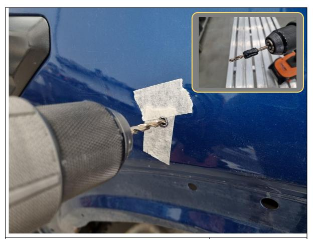
25. Use a 5mm drill bit and drill out a pilot hole on all 6x mounting holes.
