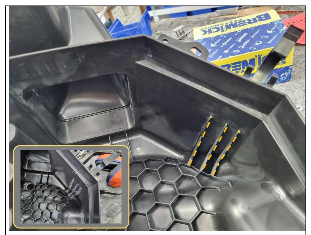
62. Use a die grinder and/or utility knife to remove the 3x internal ribs as shown.
