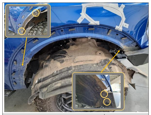
19. Remove/drop the wheel arch liner, by removing any scrivets, T20 Torx screws (towards front bumper), 10mm hex nuts (at back of wheel arch near the driver footwell) and Christmas tree clips holding to the body.
