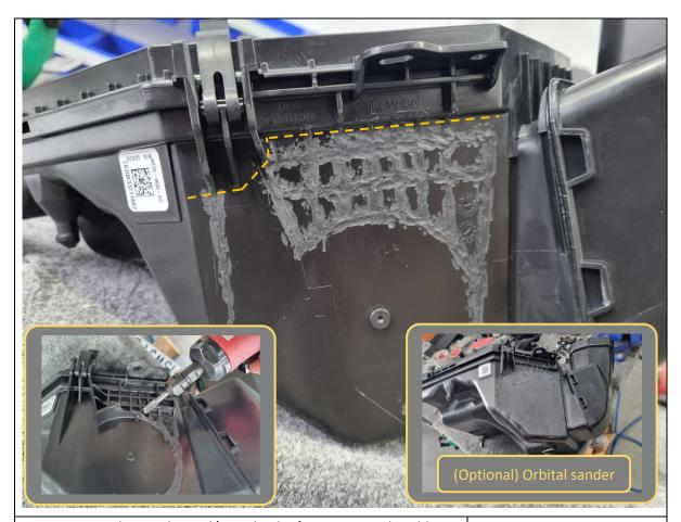
60. Use a die grinder and/or utility knife to remove the ribbing on the outside of the lower airbox, as shown. Remove enough ribbing such that the F-0026 air entry hose can fit onto the airbox.
