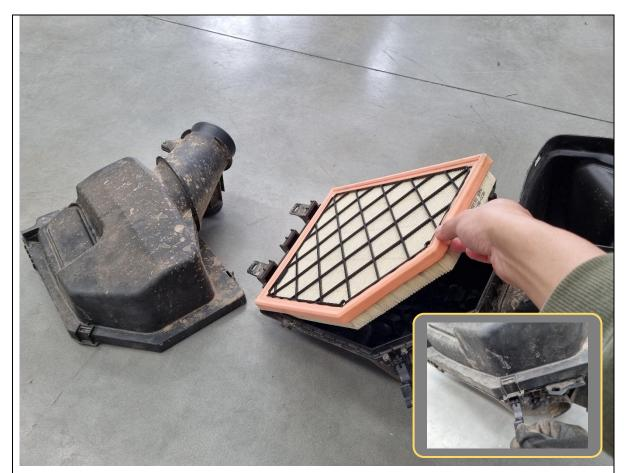
58. Unclip the 2x clips holding the upper airbox to the lower airbox.
