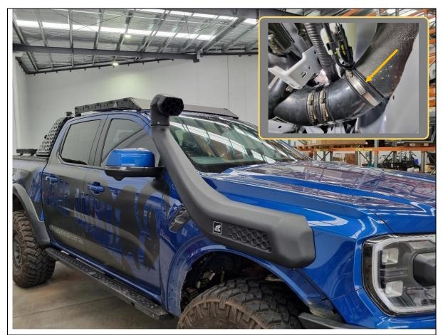
113. Carefully fit the snorkel to the vehicle. Guide the snorkel entry into the F-0027 outlet hose installed on the vehicle. If it is too tight, try adding a tiny bit of lubricant.
