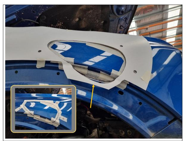
23. Re-fit and align the N-0015 paper card template back in the same position on the quarter panel, then mark out the cut line for the main snorkel intake hole that was previously covered up by the wheel flare (see arrow).
