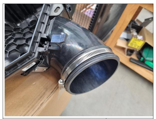
89. Loosely fit 1x hose clamp onto the end of the air entry hose, between the raised edges.
