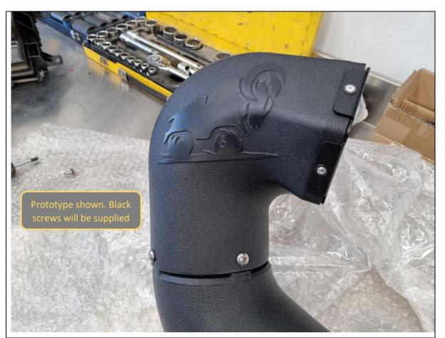
112. Fit the air ram body onto the snorkel main body, and secure with 4x black 14G pan head Phillips screws.
