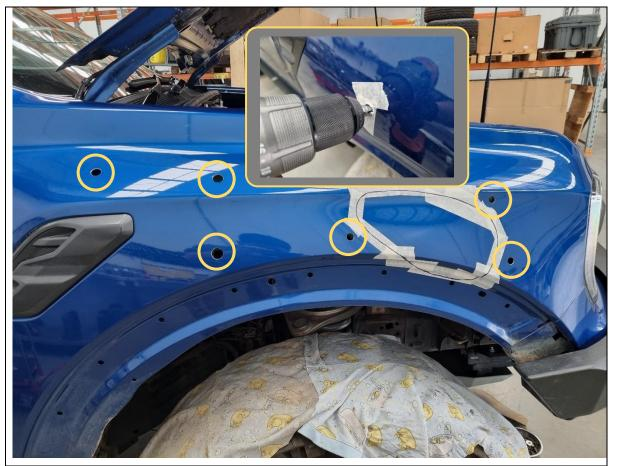
26. Use a step drill and drill out all 6x pilot holes out to 16mm diameter.
