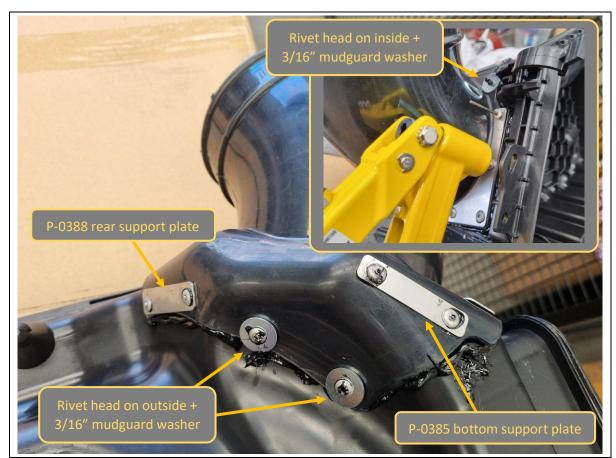
80. Install 2x size 5-6 pop rivets with 3/16" mudguard washers on the bottom.
