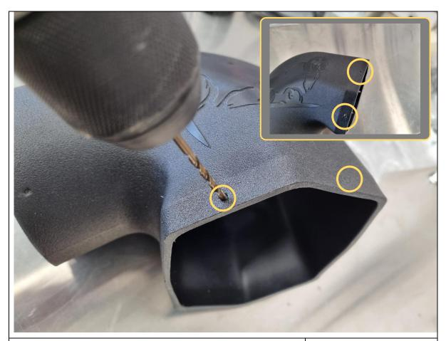
105. Locate the 4x dimples on the front of the F-0029 air ram body and use them as a guide to drill 4x 3.2mm diameter holes, to suit size 4-4 rivets (3.2mm diameter x 10mm length).
