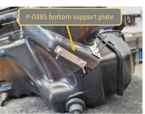
79. Install size 5-6 pop rivets and 4x support plates, as shown above. Total 12x rivets for these plates.
