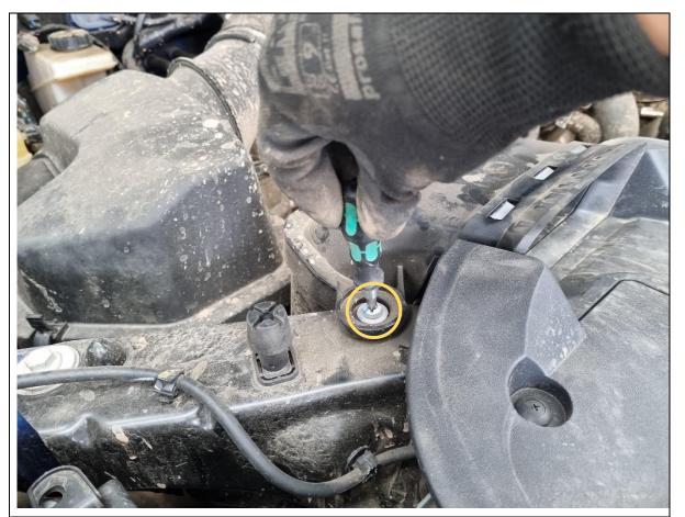
6. Remove 1x T30 Torx screw holding the front of the factory intake scoop to the vehicle body. Retain the T30 bolt for later.
