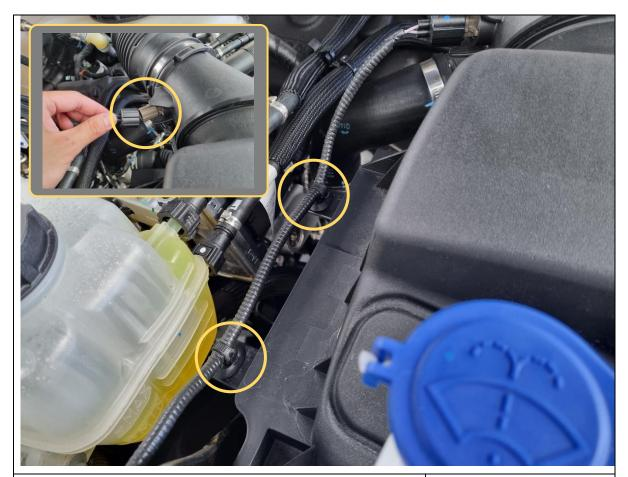
98. Re-connect the MAF sensor and clip the loom back into the airbox.
