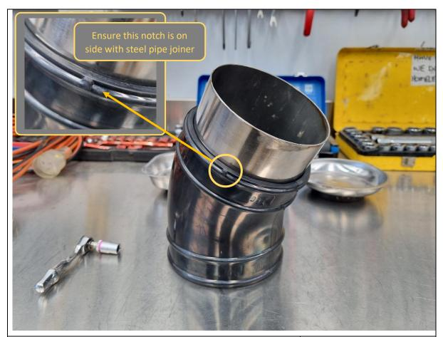
99. Fit the T-0110 pipe joiner to the F-0027 outlet hose. Ensure the pipe joiner is on the same side as the keying notch on the outlet hose as shown.
