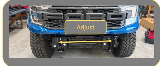
58. Measure Distance between outside edges uprights on bar using tape measure. Write distance below for reference if required.
