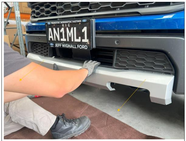
14. Remove the center silver trim on the bumper, by pulling firmly to release clips.
