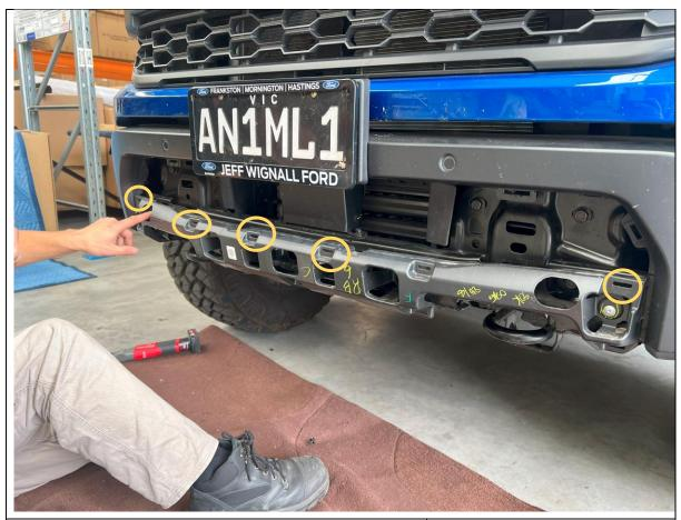
15. This will reveal the impact beam. The above photo shows the location of the clips securing the silver trim.
