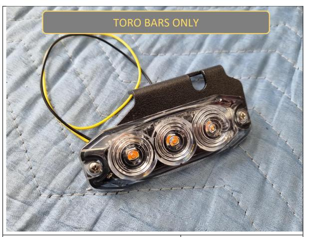
63. Fit the indicator repeater lamps to the indicator brackets, using M3 Phillips head Screws and the adhesive backing included with the lamp module.
