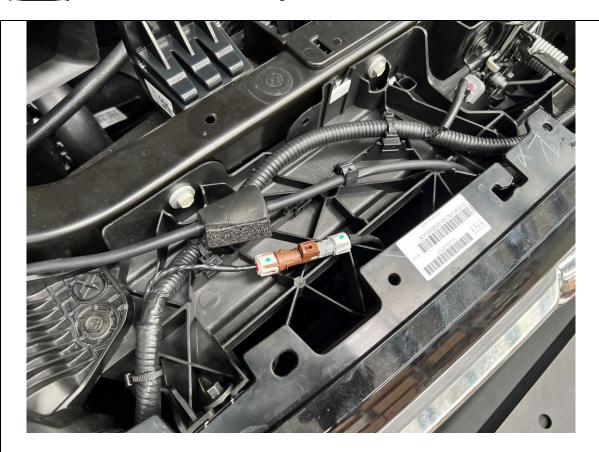
119. Re Connect Electrical Harness, camera plug and camera washer hose.
