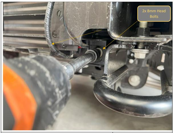
38. Remove the fasteners securing the Louvres to the lower tow point mounting bracket.
