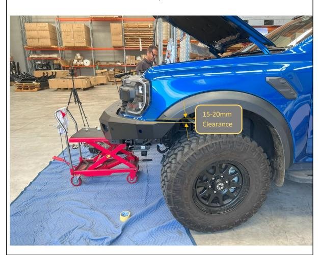
102. With assistance, from another person, Align the bar with the edges of the vehicle. Adjust such that the clearances are neat and even side to side.
