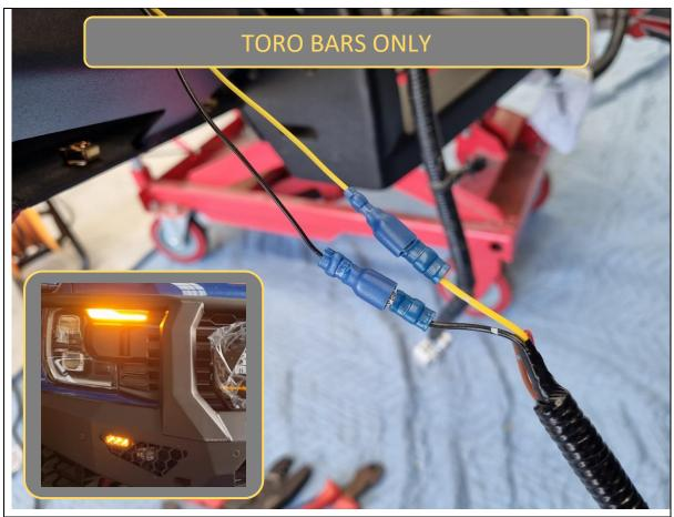
121. Connect the indicator wiring connectors fitted earlier.
