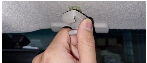
23. Grab onto the sun visor retaining clip and twist to release from the roof. (Twist anti-clockwise for the RH driver side, clockwise for LH passenger side)
