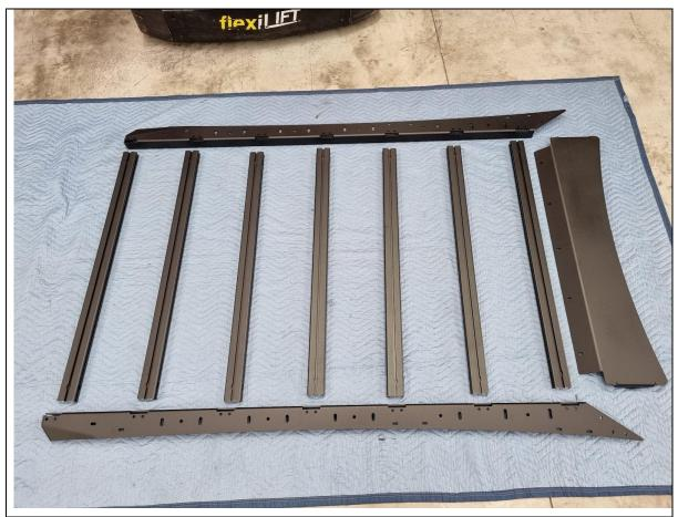
1. Find a large table space or floor area and lay out all the extrusion cross bars, rack sides and wind deflector of choice.
