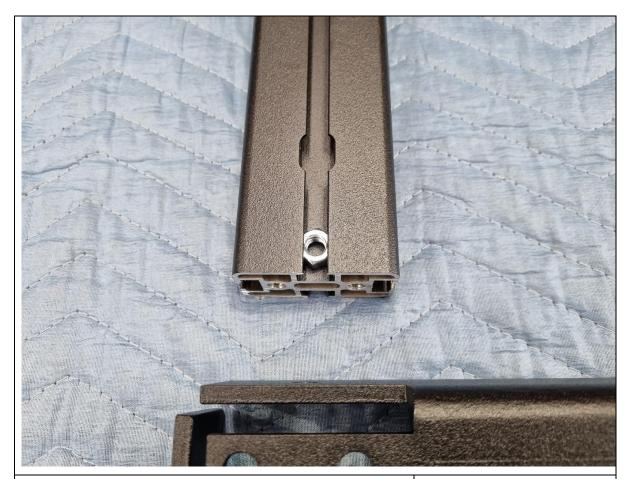
2. Insert 1x M8 nut into the top T-slot of the extrusion end.
