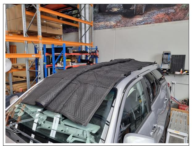
79. Place a soft blanket on the roof in between the roof channels to protect the paintwork while the roof rack is installed.
