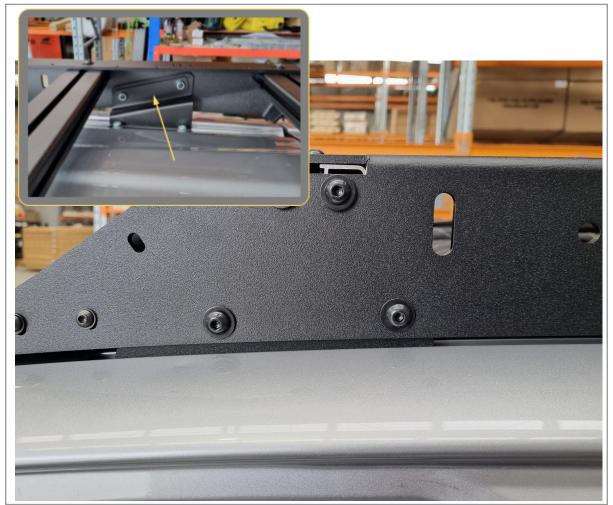
69. Start securing the roof rack to the mount brackets using M8x20 button head bolts, black washers, and 100mm M8 nut plates.
