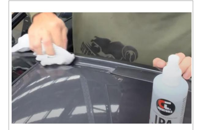
57. Using a cleaning solvent like isopropyl alcohol, give the roof channel a good clean. Make sure there is no dirt or oils left in the channel.
