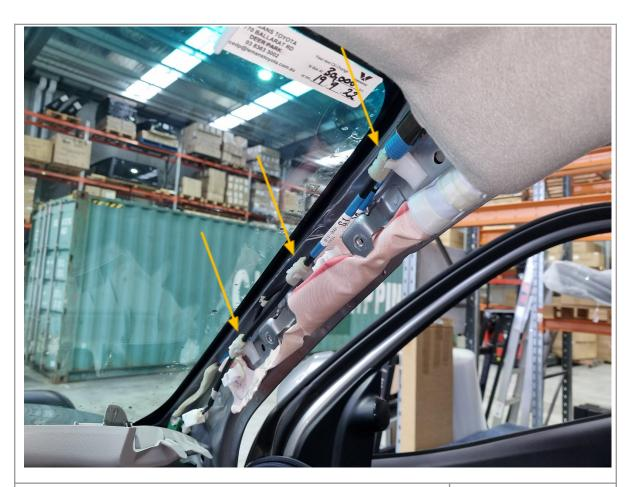
20. Carefully unclip the exposed curtain SRS airbag wire from its plastic clips as indicated.
