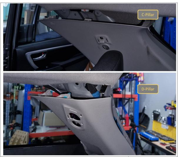
42. Starting from the top, pull and release the clips holding the C-pillar trim. Set aside the trim.
