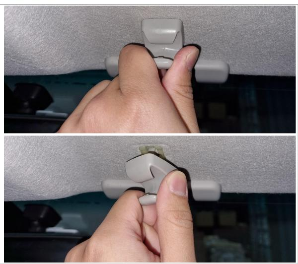
23. Grab onto the sun visor retaining clip and twist to release from the roof. (Twist anti-clockwise for the RH driver side, clockwise for LH passenger side)
