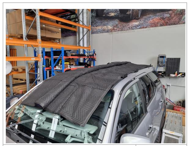
66. Place a soft blanket on the roof in between the roof channels to protect the paintwork while the roof rack is installed.
