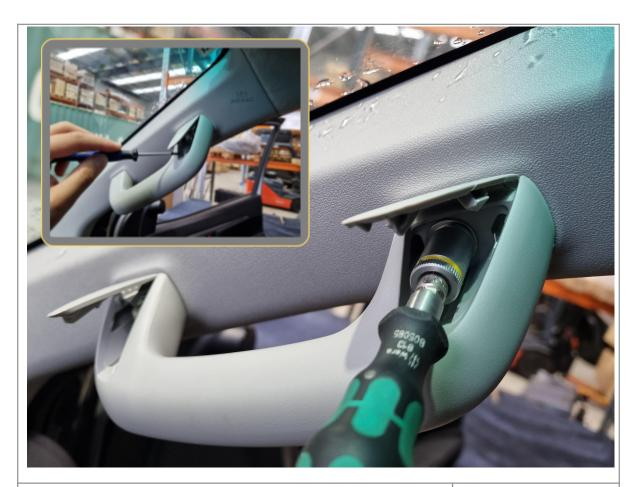
15. Headliner removal is required for fitting the roof rack. Start from the front and work your way backwards.
