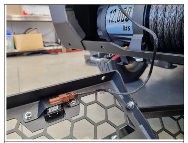
169. Present the mesh fairlead up to the bar and connect the camera to the previously installed camera extension harness.
