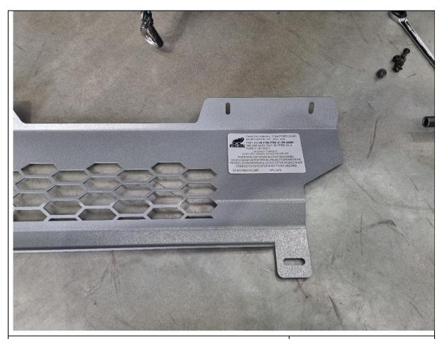
174. Fit the supplied compliance plate to the inside of the centre bash plate as shown. Peel the backing film off and adhere to the bash plate surface.
