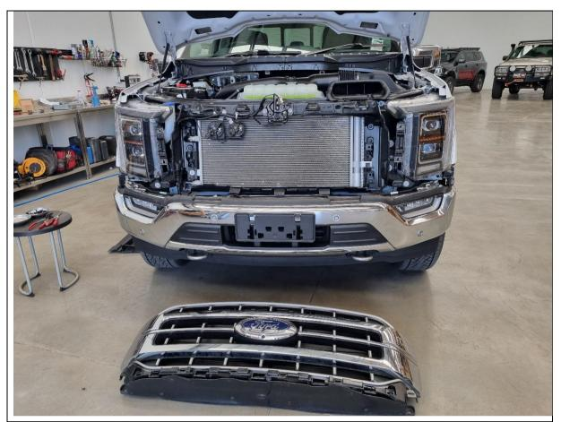
10. Pull outwards and remove the grille. Set aside for later.
