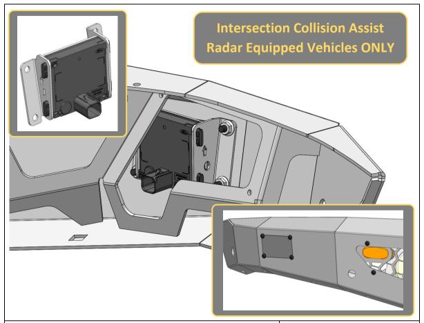
124. Take the ICA radar units from Step 20 and fit it to the inner and outer ICA radar clamp brackets.
