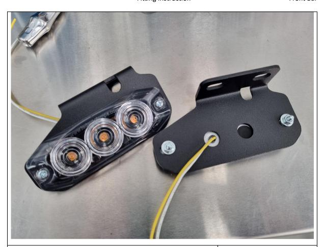
114. Fit the indicator repeater lamps to the indicator brackets, using M3x12 pan head screws, washers, nuts and the adhesive backing included with the lamp module.
