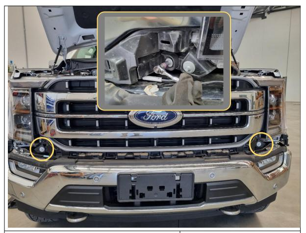
6. Remove 1x 8mm hex bolt securing the outer corner of the grille to the body, on each side.
