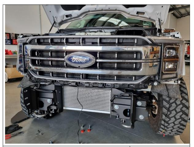
73. Re-fit the grille to the vehicle and secure using fasteners removed in Step 6 and 7.
