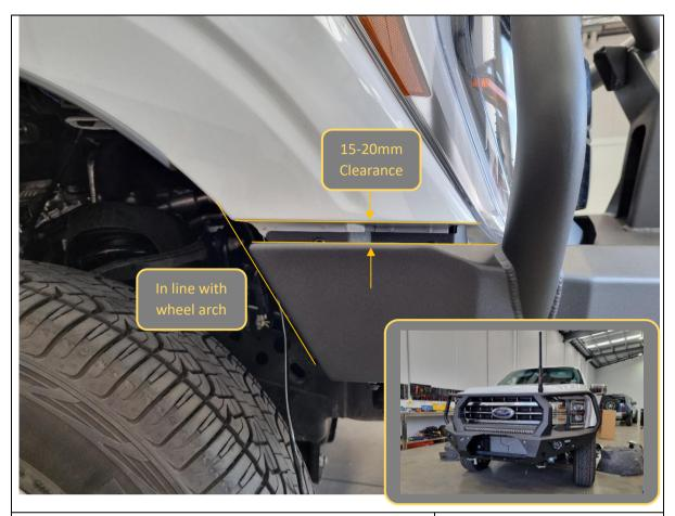
158. With assistance, from another person, align the bar with the edges of the vehicle.
