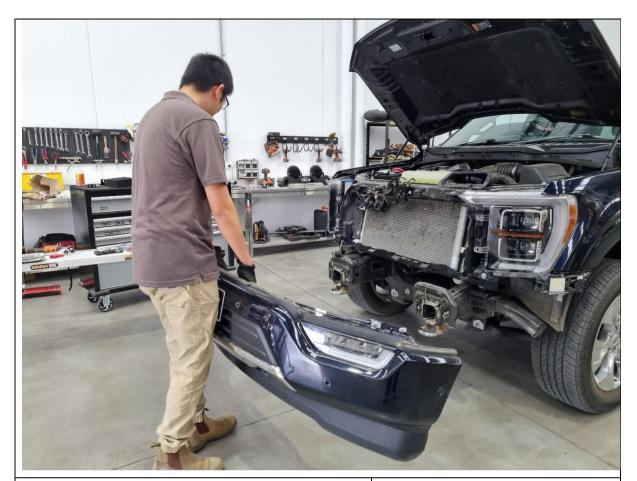
17. Pull the bumper off the vehicle and set aside in a safe place.
