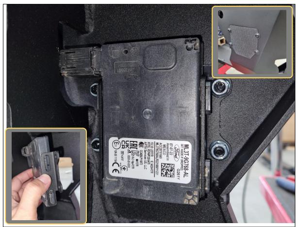
120. Fit the 2x B-1100 radar brackets onto the ACC radar unit, then hold it up against the inside of the bullbar, on the LH front face.
