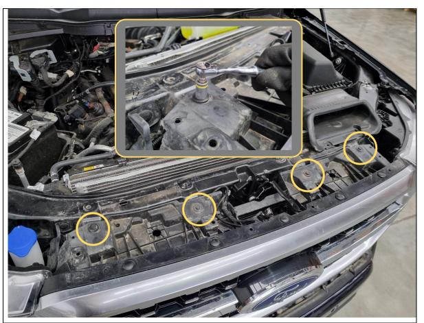
7. Remove 4x 10mm hex bolts securing the top of the grille to the body.
