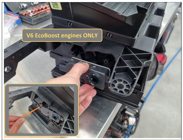
35. Remove the shutter motor by removing the 2x T20 Torx screws securing it to the shroud. Set it aside.
