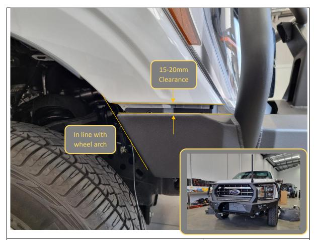
158. With assistance, from another person, align the bar with the edges of the vehicle.
