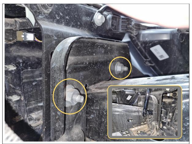
16. Remove the 3x 21mm hex nuts holding the bumper onto the chassis frame end, on each side.
