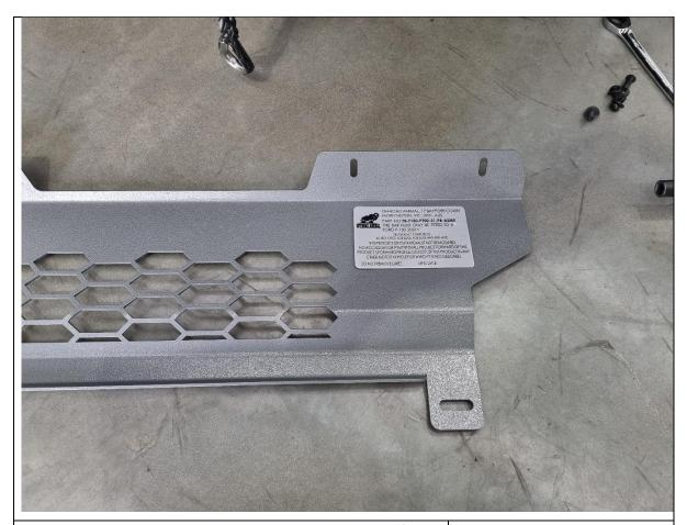
174. Fit the supplied compliance plate to the inside of the centre bash plate as shown. Peel the backing film off and adhere to the bash plate surface.
