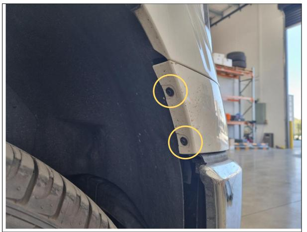
4. Remove 2x 7mm hex bolts securing the plastic bumper trim to the inner wheel guard, on each side.
