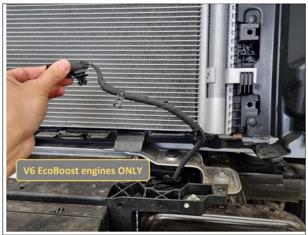
27. Unclip the remainder of the harness on top of the intercooler shroud.
