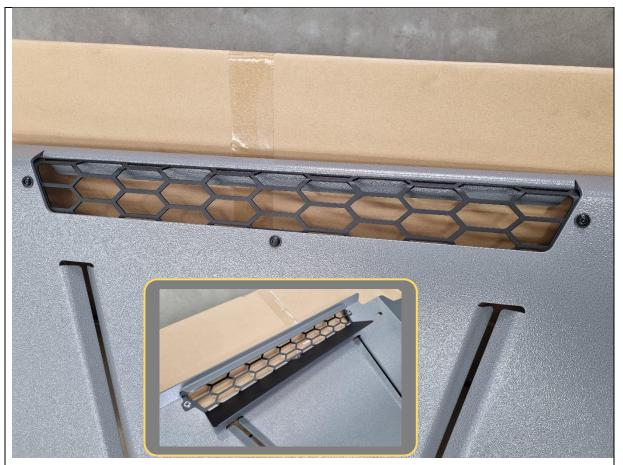
177. Bolt the air guide to the lower bash plate and secure using 3x M6x16 black button head bolts, black washers and flange nuts.
