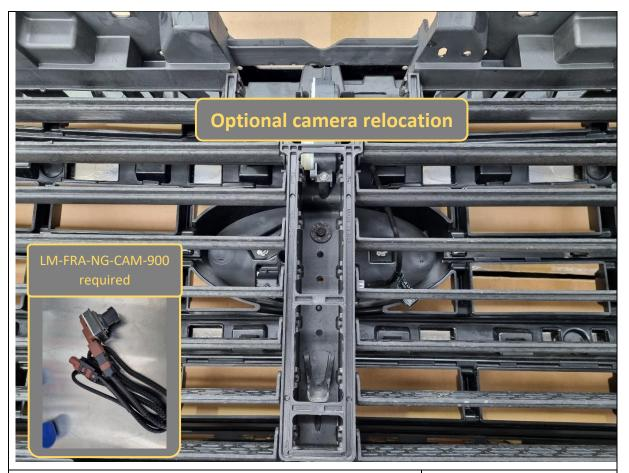
64. Front 360 degree camera relocation is optional but recommended when fitting with driving lights or Offroad Animal top tube accessories (eg. Stealth Hoop or Rally Hoop).
