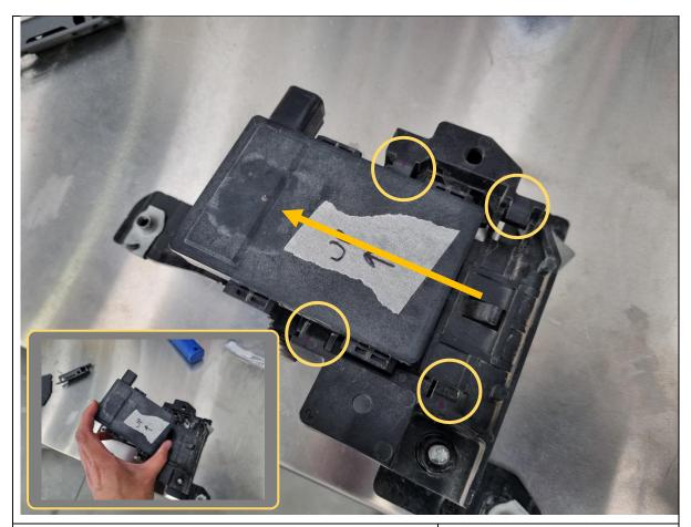
119. Release 4x tabs on the ACC radar mount and slide the ACC radar unit up and away.
