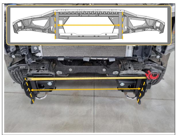
61. Measure the distance between the outside faces of uprights on bar using tape measure. Write distance below for reference if required.
