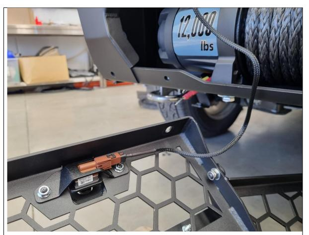
169. Present the mesh fairlead up to the bar and connect the camera to the previously installed camera extension harness.
