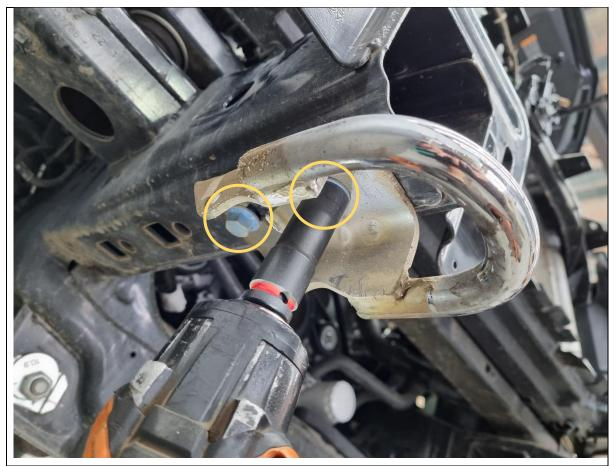
32. Remove the 2x 15mm hex bolts and nutplates securing the tow hook to the chassis, on each side. Set aside for re-fitment.
