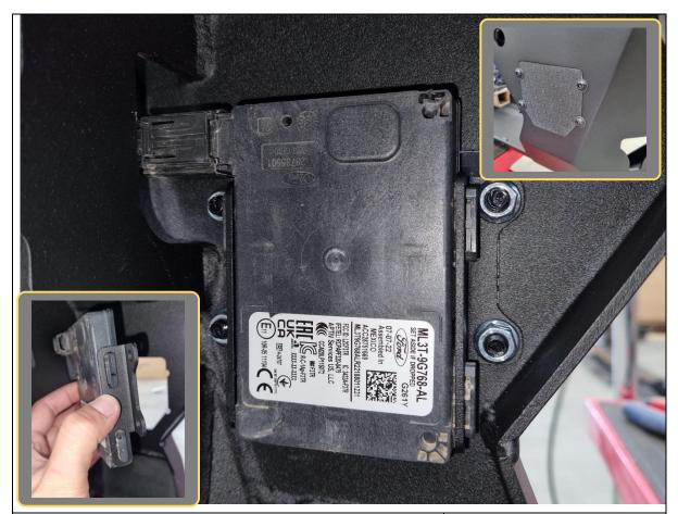
120. Fit the 2x B-1100 radar brackets onto the ACC radar unit, then hold it up against the inside of the bullbar, on the LH front face.
