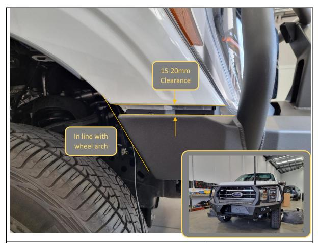
157. With assistance, from another person, align the bar with the edges of the vehicle.
