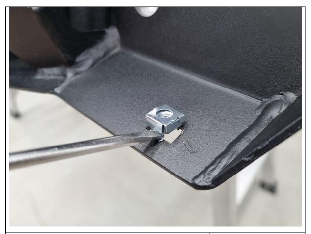
111. Fit 10x M6 cage nuts into the rectangular slots on the bottom of the bar wing (5x per side).
