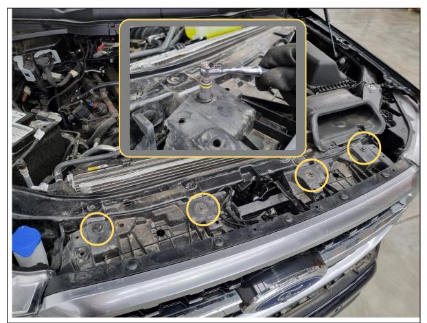
7. Remove 4x 10mm hex bolts securing the top of the grille to the body.
