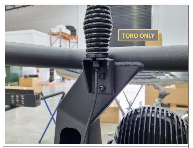
150. If fitting antennas or other accessories on the Toro bar, fit the antenna mount bracket to the back of the Toro uprights using 2x M8x20 black button head bolts and black flat washers.
