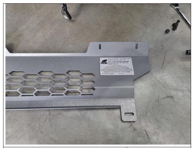
173. Fit the supplied compliance plate to the inside of the centre bash plate as shown. Peel the backing film off and adhere to the bash plate surface.
