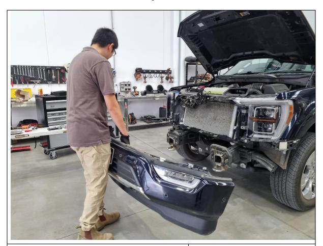
17. Pull the bumper off the vehicle and set aside in a safe place.
