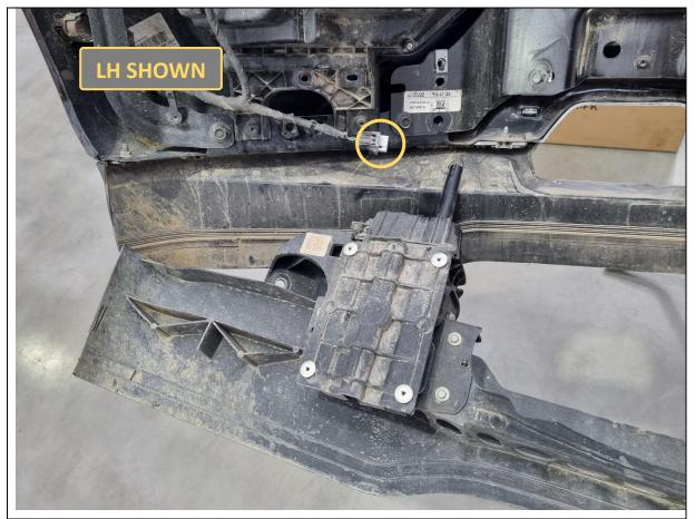
99. Disconnect the wiring harness plug to each spoiler actuator.
