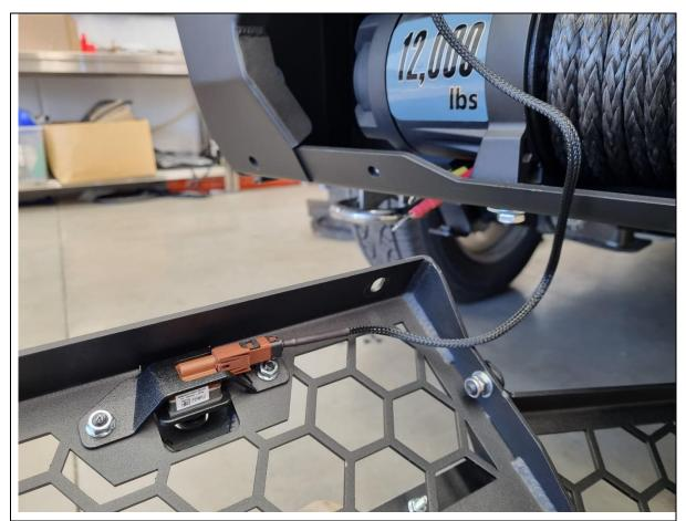
168. Present the mesh fairlead up to the bar and connect the camera to the previously installed camera extension harness.
