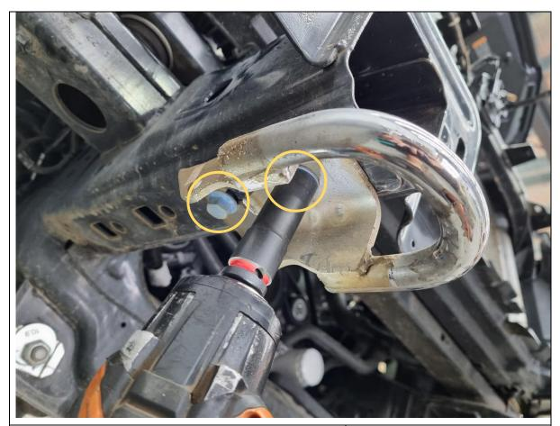
32. Remove the 2x 15mm hex bolts and nutplates securing the tow hook to the chassis, on each side. Set aside for re-fitment.
