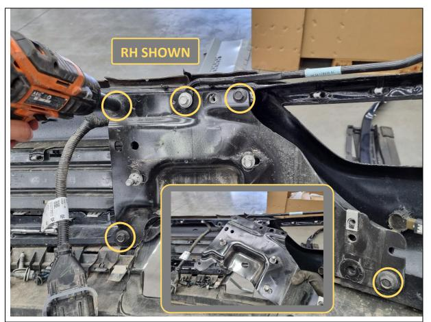
105. Remove 5x 13mm hex bolts securing the inner steel bumper bracket to the main bumper. Do this for both sides.
