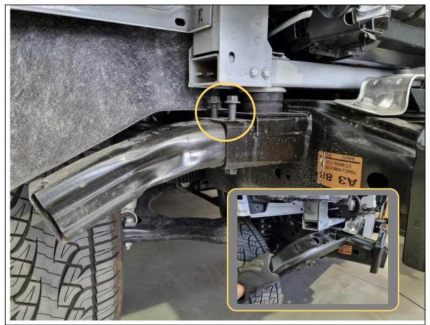
30. Remove the 2x 15mm hex bolts securing the chassis horns on each side of the chassis.
