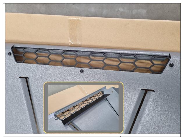
176. Bolt the air guide to the lower bash plate and secure using 3x M6x16 black button head bolts, black washers and flange nuts.
