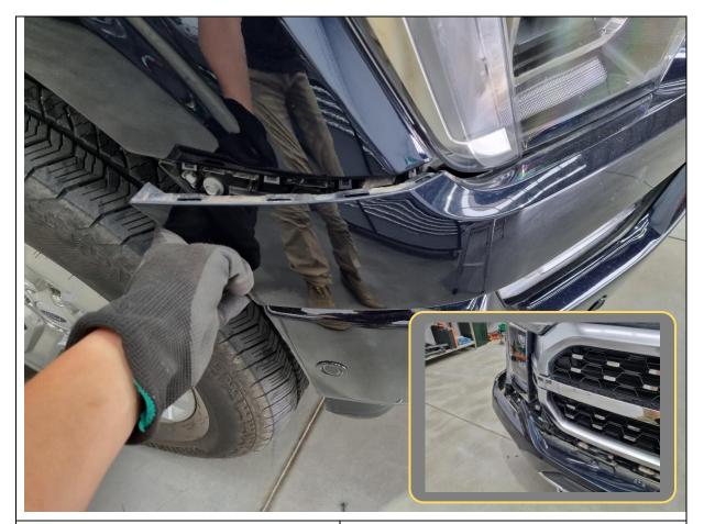
5. Pull and release the clips holding the plastic bumper trim. Set aside for later.
