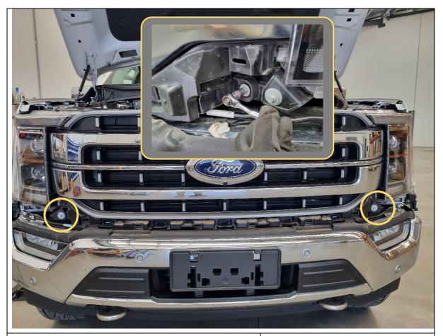
6. Remove 1x 8mm hex bolt securing the outer corner of the grille to the body, on each side.
