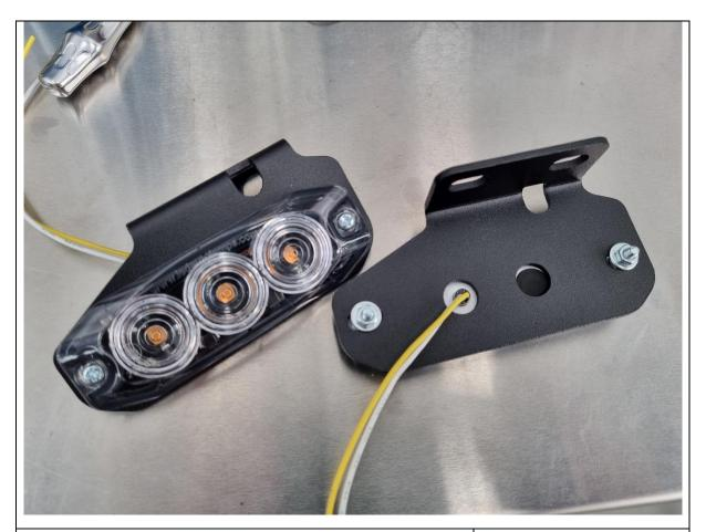
114. Fit the indicator repeater lamps to the indicator brackets, using M3x12 pan head screws, washers, nuts and the adhesive backing included with the lamp module.
