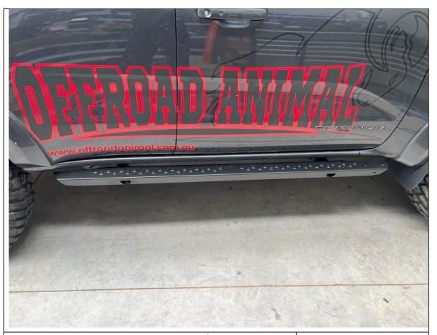
20. Check that step is sitting level to body / chassis. If the step is not level, it is likely that bolts were tightened out of sequence and mounts are not sitting flat against the chassis. To remedy loosen bolts and Repeat Steps 18 and 19.
