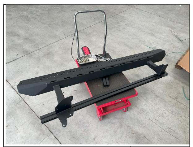
13. Unpack welded slider assembly and position on lifting trolley such that mounts sit approximately level.
