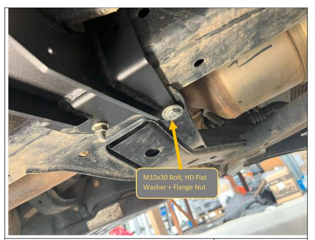
17. Once secure, finish front mount installation securing final mounting point with M10x30 Bolt, HD Flat Washer, and Flange Nut.
