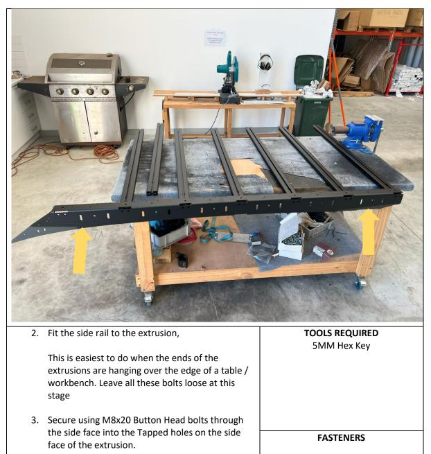
4. Complete steps 3 through 5 for the other side of the rack assembly to fit the other side rail.
