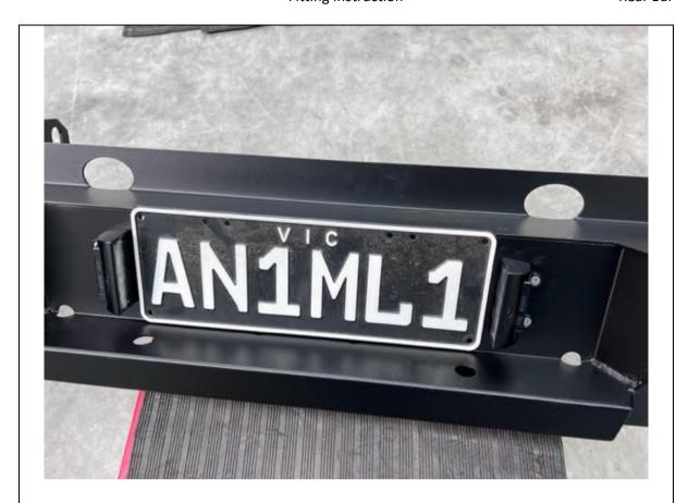
8. Fit number plate lights and number plate as shown with M5 pan screws and flange nuts. Use supplied hardware with lights to fit them
