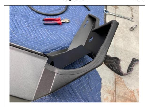
9. Fit pinch weld over edges of each wing as shown. This protects the vehicle during installation of the bar
