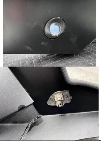
10. Use an industrial grade adhesive silicone or double-sided tape to secure sensor housings to bar. Before gluing in, ensure you can get sensor wiring to each sensor. Ensure area is clean of all dirt and grime before fitting housing to bar.
