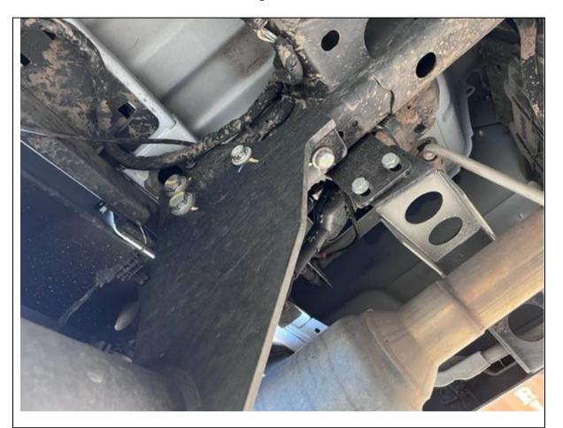
15. Lift bar on to vehicle with a friend or aid of a lifting trolley, and secure new bumper to tow bar with large M16 x 110 bolts and nuts Torque these bolts
