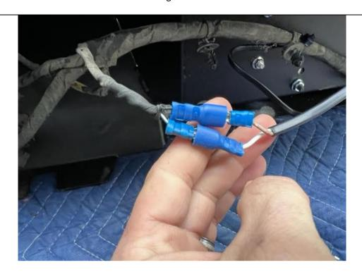
14. Wire in new number plate lights to existing wires and link together with terminals
