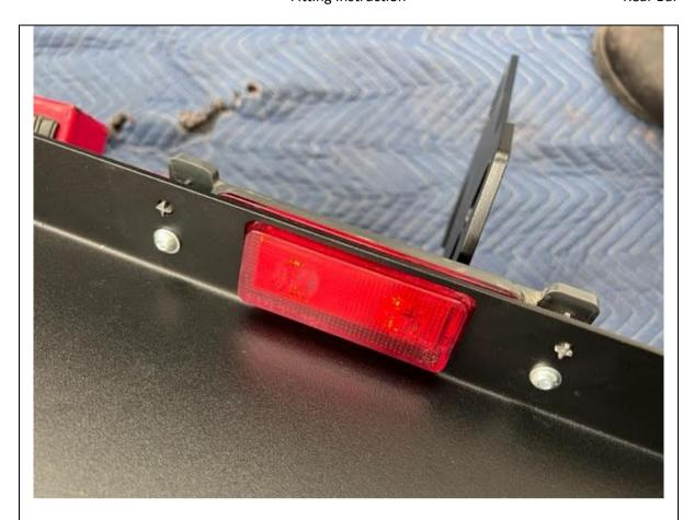
7. Refit rectangular stop lamp and reverse lamp into the new bumper with M6x 35 button head cap screws and nyloc nuts
