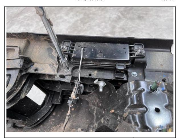
2. Remove factory reverse and brake lamp from factory bumper
