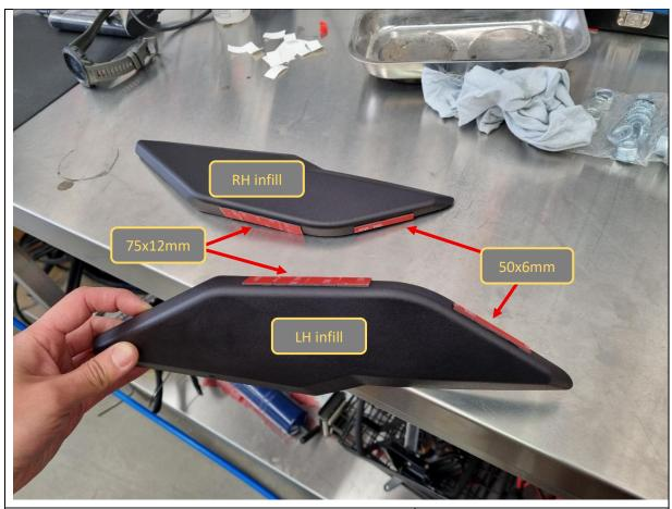
64. Apply supplied 3M VHB tape strips to the 2x grille infills as shown.
