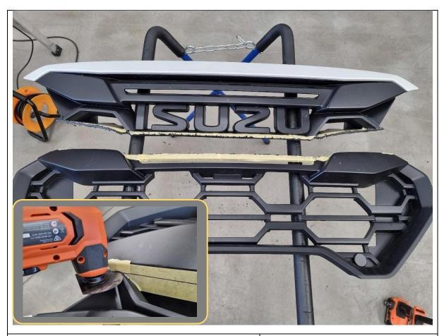
50. Trim the grille along the cut line using an oscillating multi-tool or similar device.
