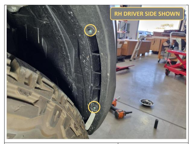
16. In the front wheel well area, remove 2x 8mm hex screws holding the flare to the bumper. Do this for both sides.
