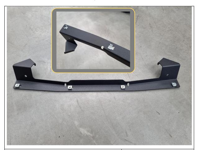
53. Fit 4x M6 cage nuts to the rectangular cutouts in the B-1575 grille mount. Use a flat blade screwdriver to assist.
