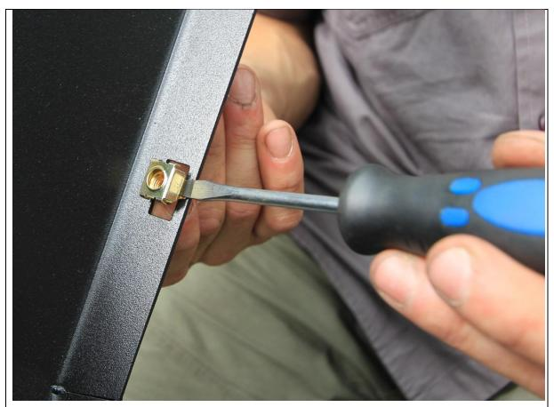
120. Fit 10x M6 cage nuts into the rectangular slots in bottom of wing (5x per side)
