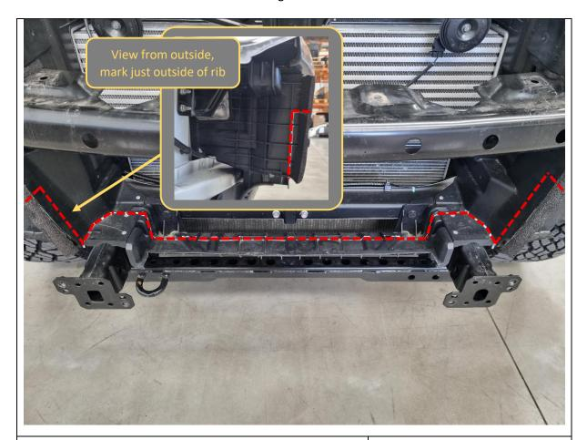
38. The plastic air guide needs to be trimmed. Use a marker pen and mark the air guide using the above images as reference.
