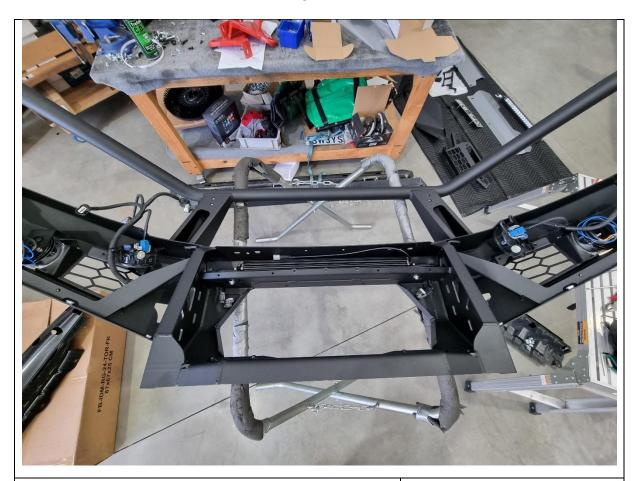
123. Route the fog light bumper wiring harness through the inside of the bullbar.
