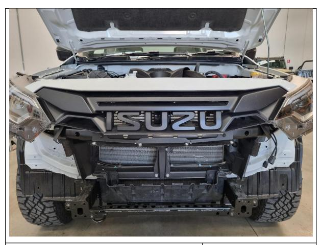
59. Re-fit the grille, radiator grille cover and factory air intake scoop to the vehicle. Secure using original plastic push clips.
