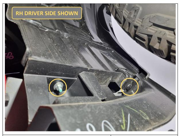
15. In the front wheel well area, remove 1x 10mm flange nut and 1x plastic push clip holding the bottom of the bumper to the wheel arch liner and outer support bracket. Do this for both sides.
