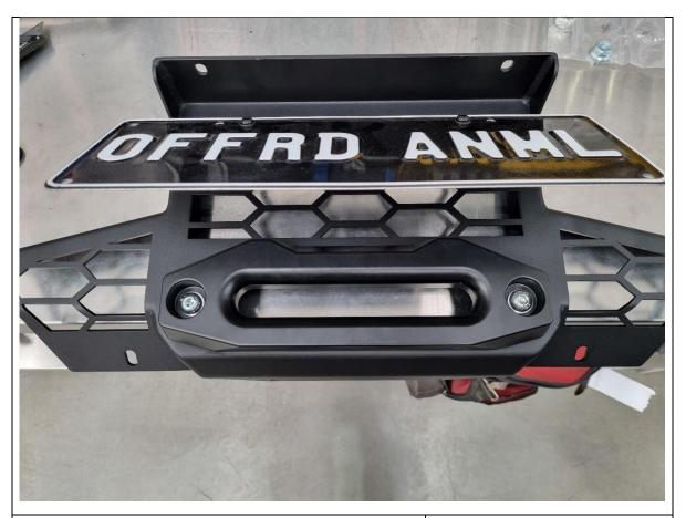
146. If required, fit the winch fairlead to the mesh fairlead mount using M10 or 3/8" fasteners supplied with the winch. This bar is only compatible with hawse type fairleads.
