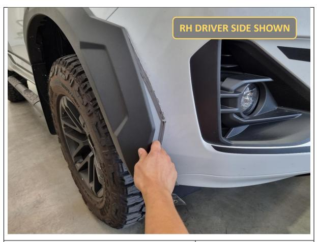
20. Starting from the bottom, pull on the front of the flare and separate it from the bumper.
