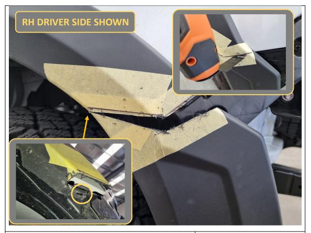
72. Using an oscillating multi-tool or similar, cut the flare along the marked cut line. Take care not to touch the quarter panel underneath.
