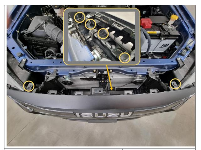
12. Remove 6x plastic push clips holding the grille.
