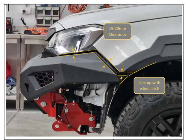
139. With assistance, from another person, align the bar with the edges of the vehicle. Adjust such that the clearances are neat, and the bar is symmetric left/right on the vehicle.
