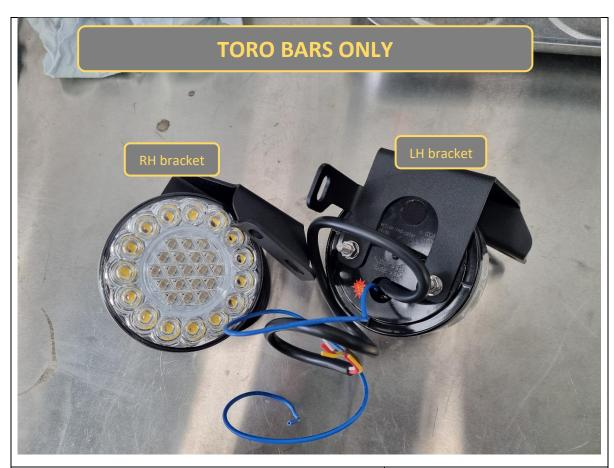
116. **Toro only.** Fit indicator units to the indicator mounting bracket, using fasteners supplied with the indicator.
