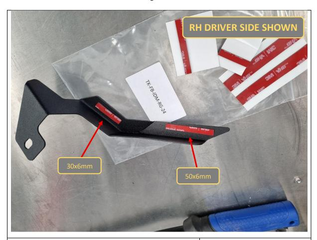
84. Apply supplied 3M VHB tape strips to the inside of the B-1576 flare endcap as shown. Do this for both LH and RH endcaps.
