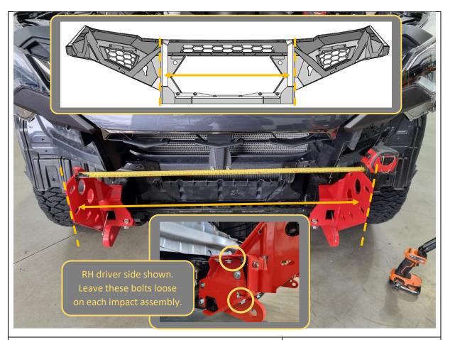
109. Measure the distance between the outside faces of uprights on bar using tape measure. Write distance below for reference if required.
