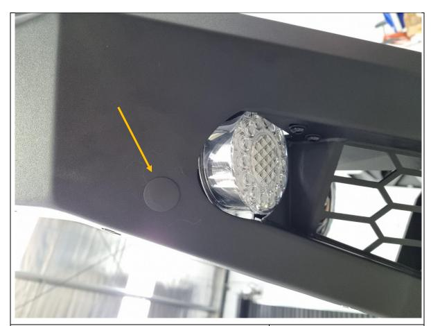
130. Insert the supplied plastic round blanking plugs into all 4x parking sensor holes in the bullbar.
