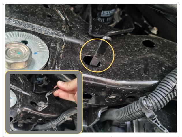
37. Remove any leftover nutplates, flange nuts and/or spacers from the chassis where the tow point assembly was bolted to.
