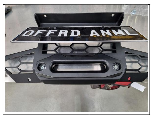
120. If required, fit the winch fairlead to the mesh fairlead mount using M10 or 3/8" fasteners supplied with the winch. This bar is only compatible with hawse type fairleads.
