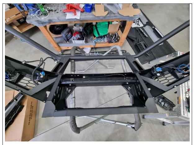
87. Route the bumper wiring harness through the inside of the bullbar.
