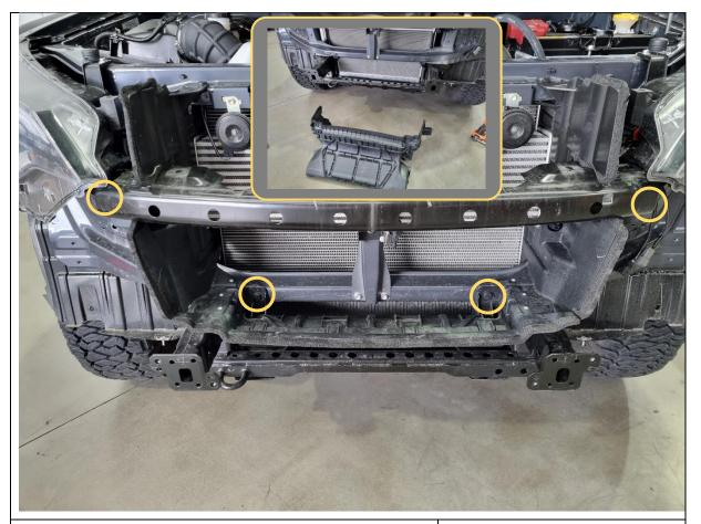
21. Remove the 4x plastic push clips holding the lower plastic air guide.
