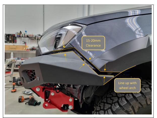
113. With assistance, from another person, align the bar with the edges of the vehicle. Adjust such that the clearances are neat, and the bar is symmetric left/right on the vehicle.
