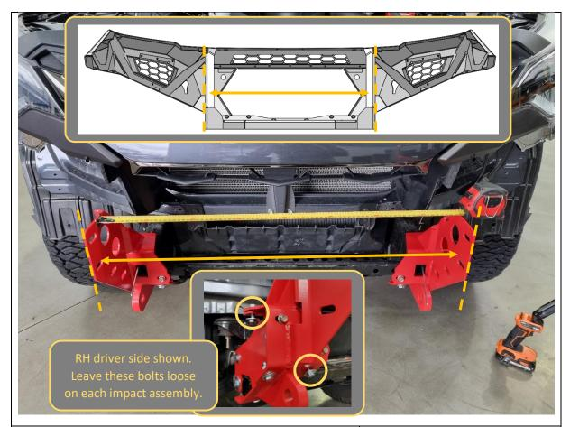
73. Measure the distance between the outside faces of uprights on bar using tape measure. Write distance below for reference if required.
