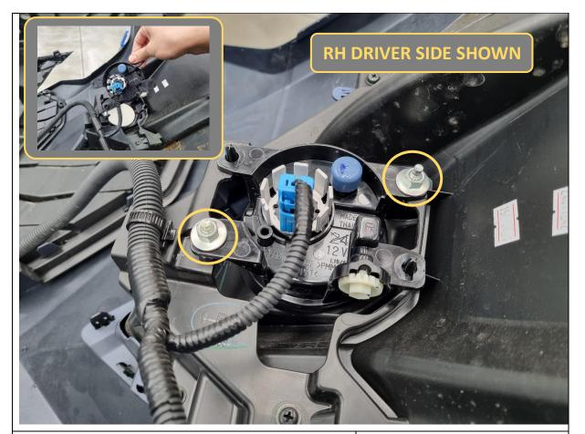
26. If equipped, remove 2x 10mm flange nuts securing each fog light on the back of the bumper.
