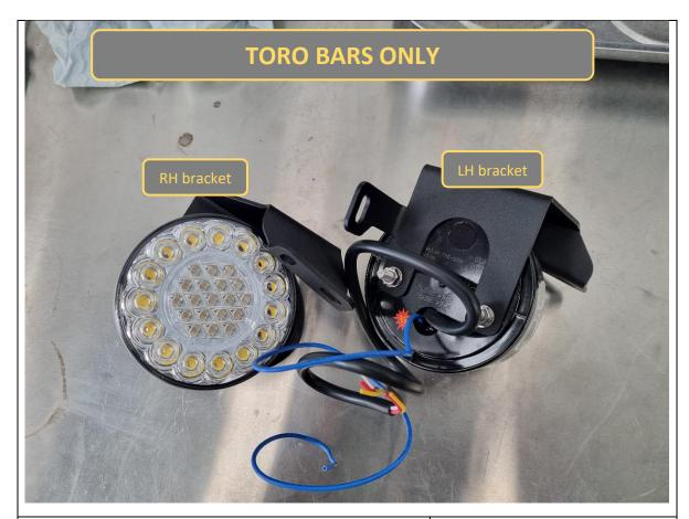
80. **Toro only.** Fit indicator units to the indicator mounting bracket, using fasteners supplied with the indicator.
