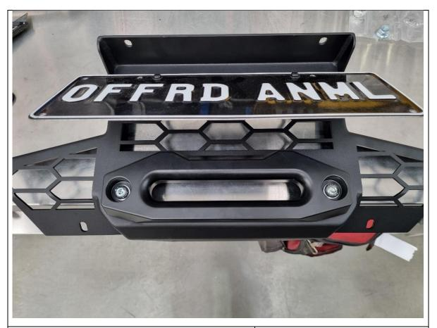
117. If required, fit the winch fairlead to the mesh fairlead mount using M10 or 3/8" fasteners supplied with the winch. This bar is only compatible with hawse type fairleads.
