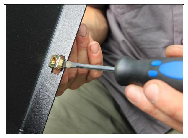
84. Fit 10x M6 cage nuts into the rectangular slots in bottom of wing (5x per side)
