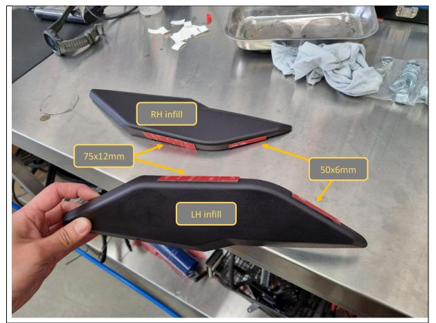
48. Apply supplied 3M VHB tape strips to the 2x grille infills as shown.
