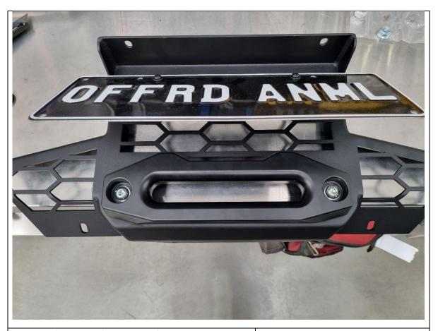
116. If required, fit the winch fairlead to the mesh fairlead mount using M10 or 3/8" fasteners supplied with the winch. This bar is only compatible with hawse type fairleads.
