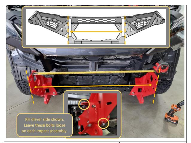
72. Measure the distance between the outside faces of uprights on bar using tape measure. Write distance below for reference if required.
