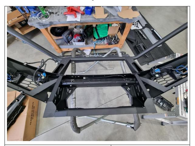
86. Route the bumper wiring harness through the inside of the bullbar.
