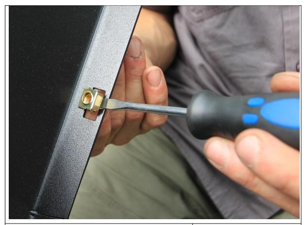
83. Fit 10x M6 cage nuts into the rectangular slots in bottom of wing (5x per side)
