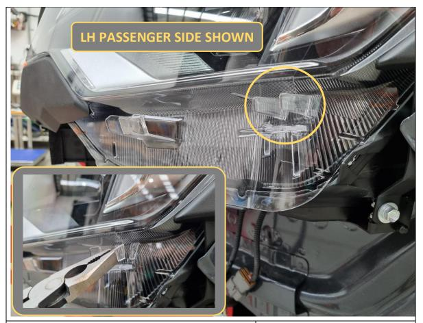
63. Use a pair of pliers to cleanly snap/bend off the 2x outermost plastic tabs under each headlight.
