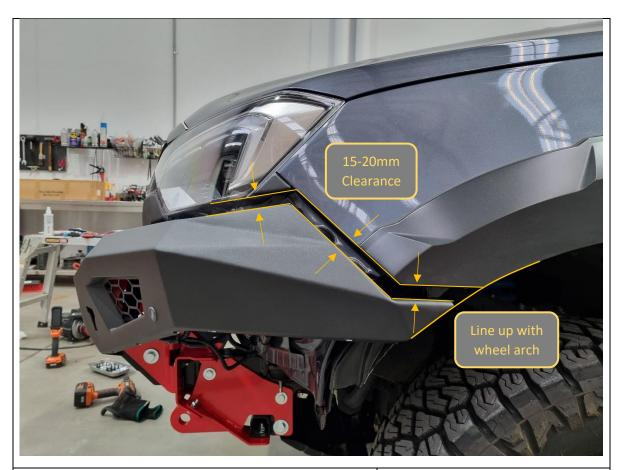
109. With assistance, from another person, align the bar with the edges of the vehicle. Adjust such that the clearances are neat, and the bar is symmetric left/right on the vehicle.
