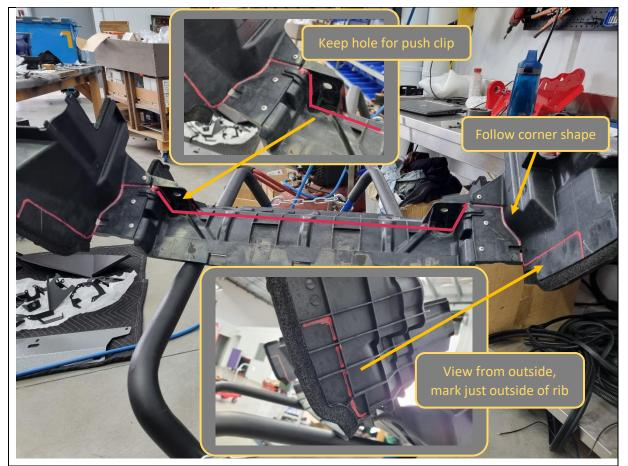
23. Use a marker pen and mark a cut line on the air guide, as shown.
