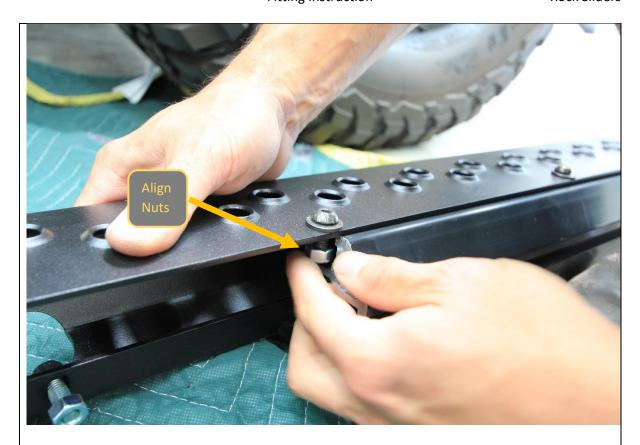
26. Slide the step plate onto the main slider structural extrusion. Align the nuts as they enter the T Slots on the extrusion.
