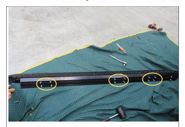
32. Slide the 12x M10x25 Hex bolts into the T slots on back side of extrusion. 6 bolts per slot.
