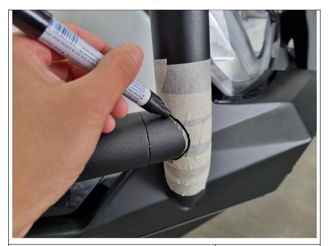
58. Using a marker pen, trace the outline of the spigot in position onto the Toro bar tube.
