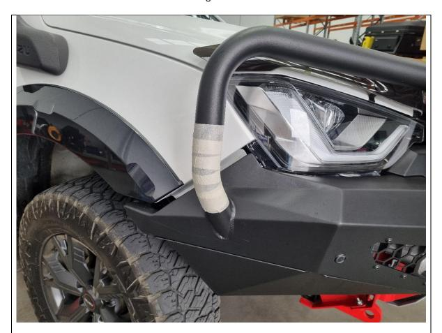
49. Apply masking tape around the outer bend of the Toro bar tube where the scrub rail will attach to.
