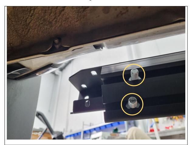
50. Slide in 2x M10x25 hex bolts into the front open end of the extrusion as shown.
