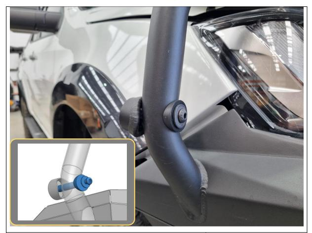
67. Loosely position the spigot with the Toro bar and hold in place with 1x M10x100 black button head, flat washer, nylon saddle washer and crush tube, through the 18mm drilled hole in the bar.
