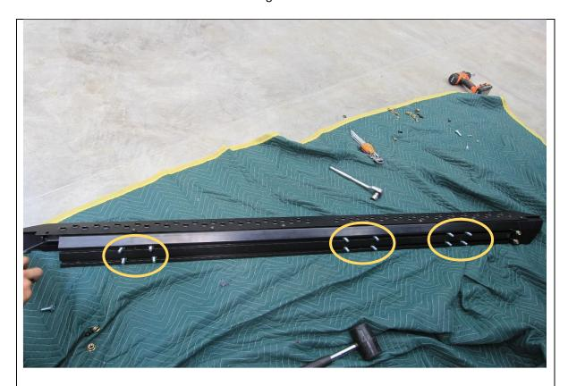
44. Slide the 12x M10x25 hex bolts into the T-slots on the back side of the extrusion. 6 bolts per slot.
