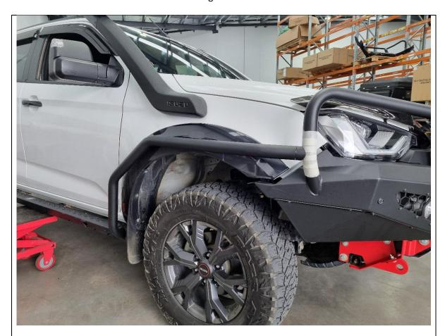
51. Perform a dry test fit of the scrub rail by sliding it into the open end of the slider step.
