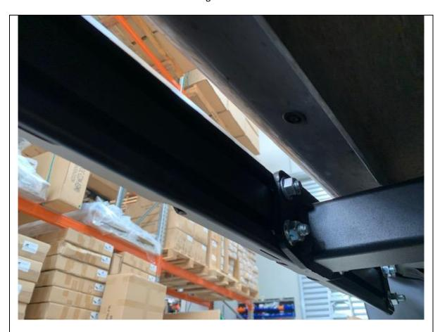
46. With the help of a friend or mate, lift step and extrusion up to brackets. Align all the bolts so they fit through the corresponding holes in the brackets.
