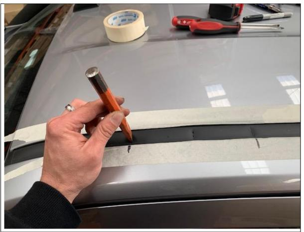
6. Using a cold chisel, carefully strike the roof rubbers at the front and rear points measured earlier. These initial strikes should be reasonably gentle such that they cut the rubber and score the metal strip embedded within.
