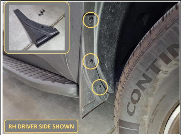
6. The front half of the flares need to be unclipped to remove the bumper, and will need to also be trimmed prior to fitting the bull bar.
