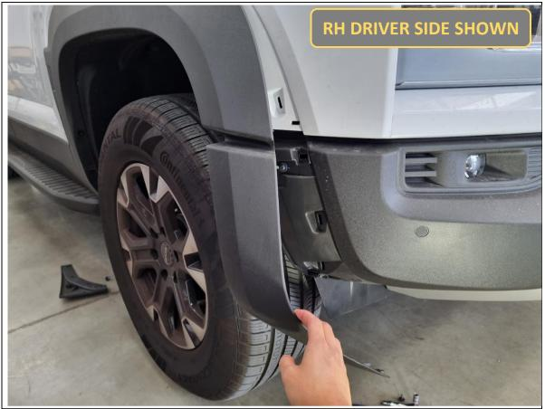
10. Starting at the front, carefully pull outwards and unclip the flare.
