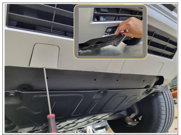
15. Use a small flat blade screwdriver to remove the 3x cover panels on the bottom of the bumper.
