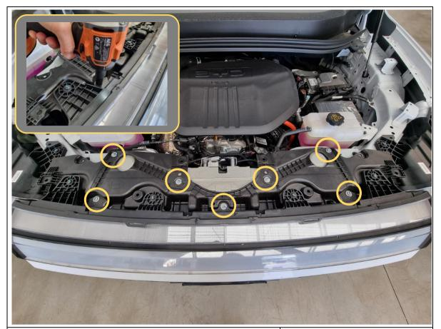
5. Remove 7x 10mm silver coloured hex bolts holding the top of the grille to the vehicle.
