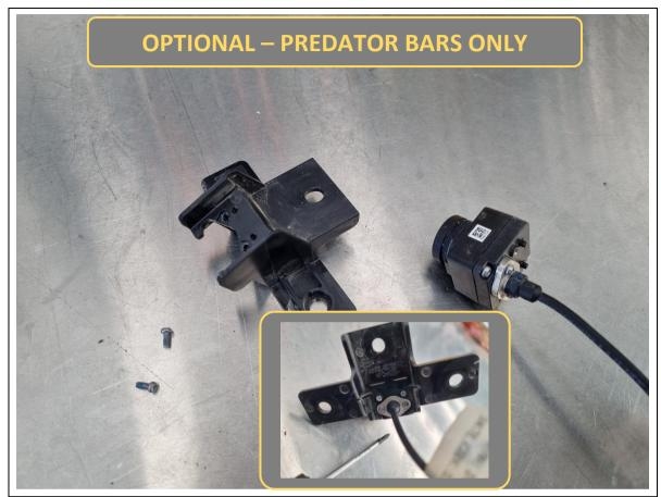
127. **Predator only (optional)** Remove 2x small Phillips head screws holding the camera to its mounting bracket. Retain these screws.
