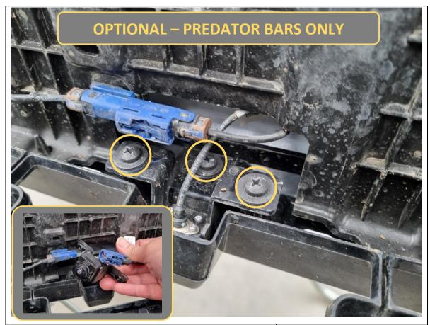
65. **Predator only.** For Predator bars, there is the option to relocate the front 360 degree camera if fitting with a Stealth Hoop or Rally Hoop bolt-on top tube.
