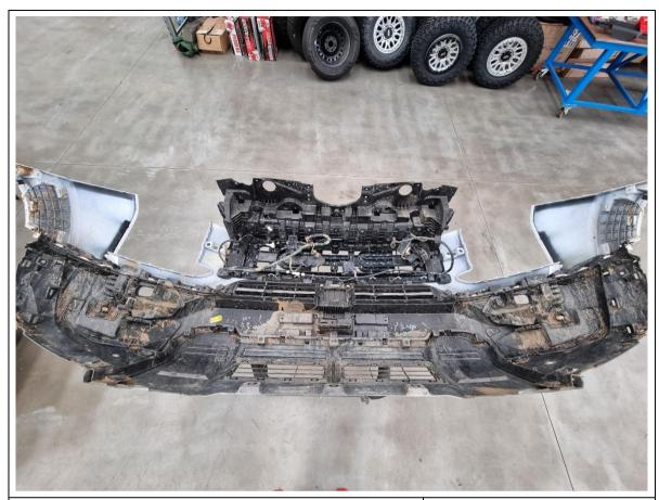
19. Pull outwards and unclip the remainder of the front bumper. Set aside in a safe place.
