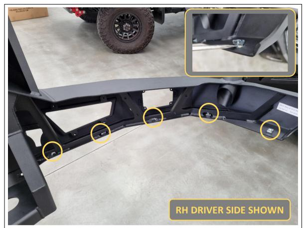
98. Fit 10x M6 cage nuts into the rectangular slots in bottom of bull bar wing (5x per side).
