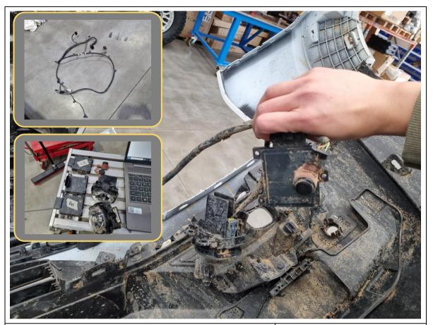
64. Release the loom from the bumper by either unclipping or cutting the retaining clips and set aside.
