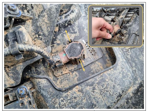
62. Unclip the 2x parking sensors. Spread the tabs on the bumper apart and push the sensor out the back.
