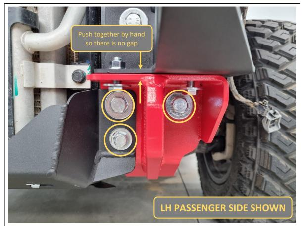
57. Next tighten the tow point front bolts and bash plate reinforcement to the chassis.
