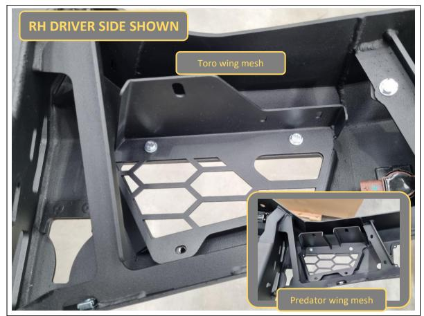
110. Fit the wing meshes to the inside of the bar. Secure each one only at the top with 2x M6x12 hex bolts and flat washers.
