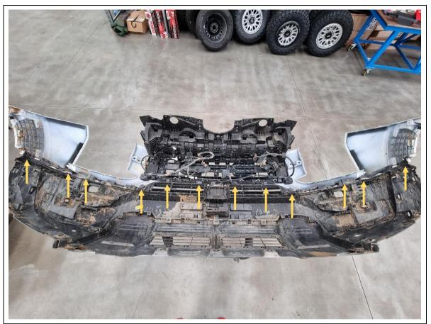
66. Remove 12x Phillips head screws holding lower section of bumper to grille top section.
