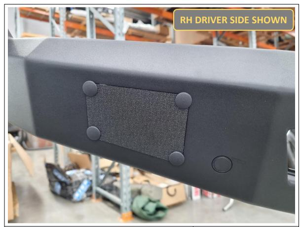
108. Fit the N-0021 plastic radar covers to the open windows in each bull bar wing, textured face on the outside.
