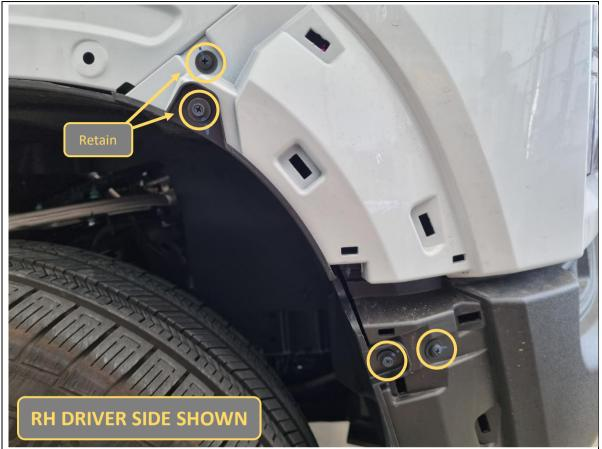
11. Remove 4x screws on each side of the bumper with a Phillips head screwdriver and/or 8mm socket/spanner.
