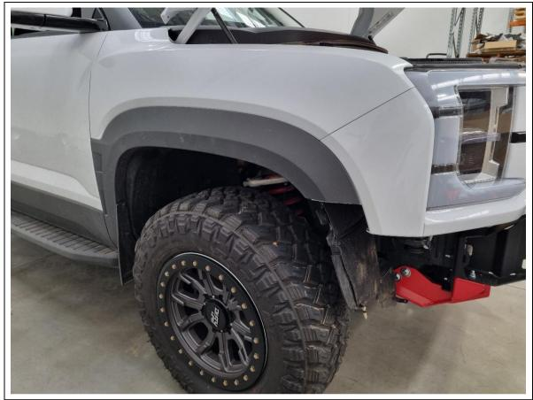
85. Re-fit the trimmed flares and mudflaps (if removed). Re-use the 10mm factory fasteners from Step 7 + 9.
