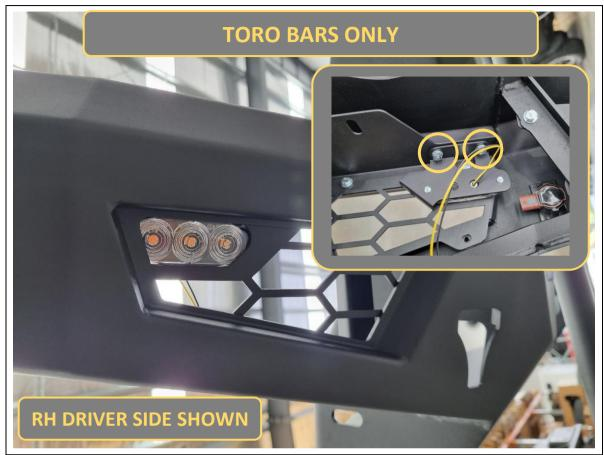
112. **Toro only.** Fit the indicators and brackets to the back of the wing mesh. Secure each one with 2x M6x12 hex bolts, flat washers and flange nuts.
