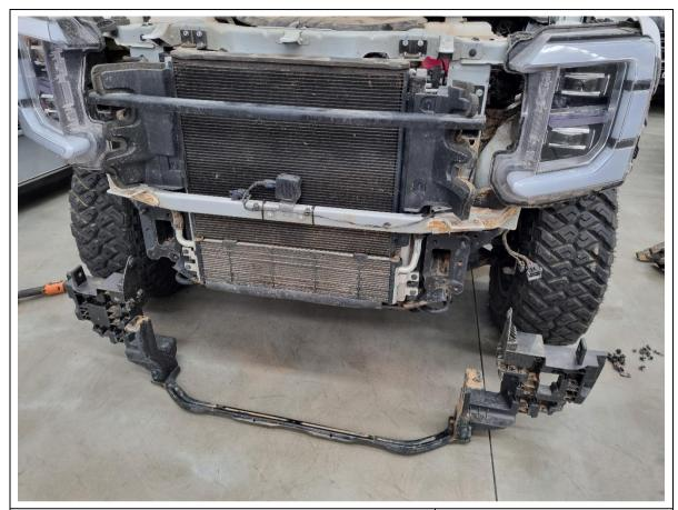
30. Fully remove and discard the bumper support structure.
