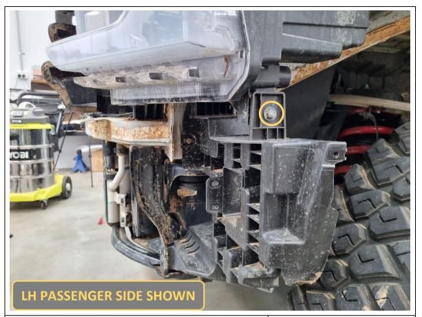
29. Also remove 1x 10mm hex bolt holding the bumper support to the bottom outside corner of each headlight.
