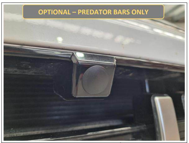
126. **Predator only (optional).** Fit the supplied plastic blanking plug in the hole in the grille where the camera was.
