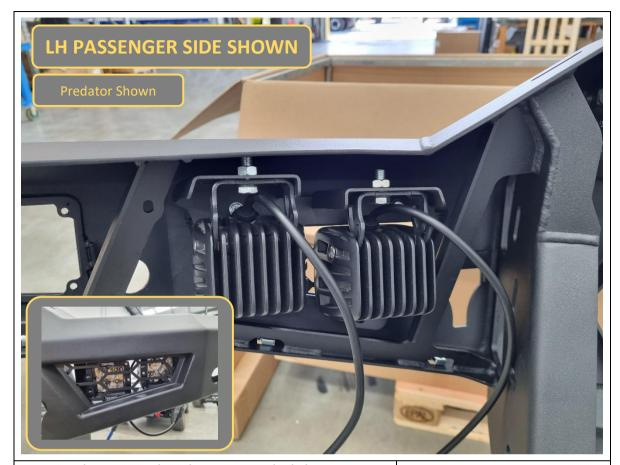
115. The wing meshes also support cube lights in addition to, or to replace the fog lights.
