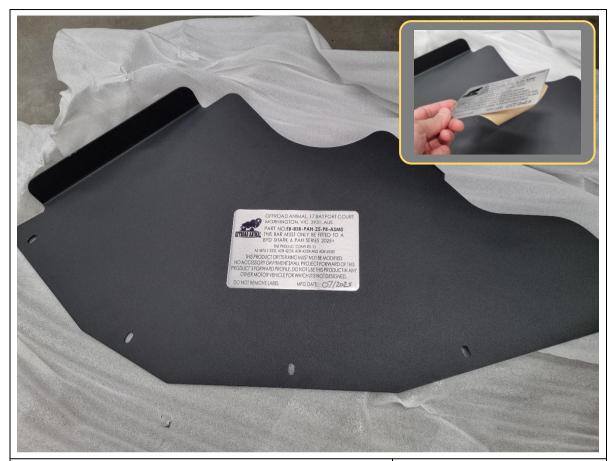
167. Peel off the backing film and affix the ADR compliance plate to the inside of the one of the side underpanel.
