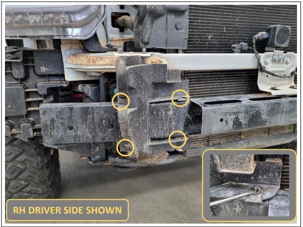
20. Remove 4x plastic push clips holding each lower air dam to the front impact beam. Use a flat blade screwdriver or trim tool to assist.
