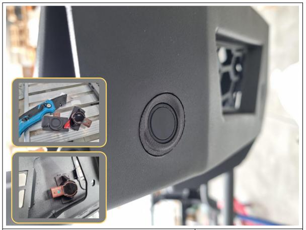
104. Remove backing film on VHB tape (easier with knife to peel off) and adhere parking sensors in position in bar. Apply pressure for at least 10 seconds after positioning for best adhesion.
