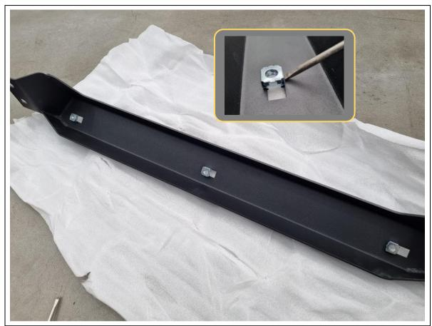
46. Fit 3x M8 cage nuts to the inside of the B-1601 bash plate reinforcement bracket as shown. Use a flat blade screwdriver to assist.
