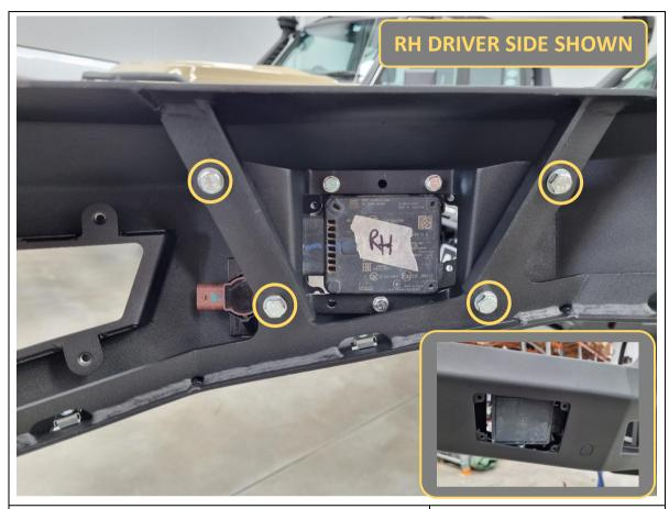
107. Install the side radar and bracket into the bull bar wing. Secure the bracket to the bracing inside the bar with 4x M6x12 hex bolts, flat washers and flange nuts.
