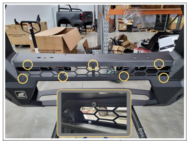
96. Time to dress the bar. Fit the light bar mesh plate to the inside of the central cutout, and secure using 7x M6x12 black countersunk bolts and flange nuts.
