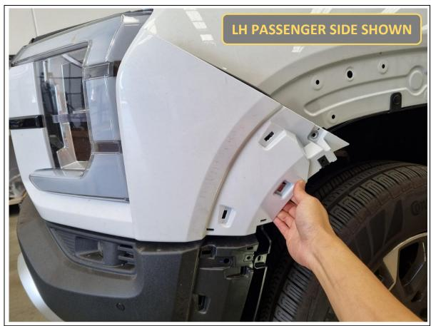
17. Pull outwards and unclip the bumper from the LH corner.
