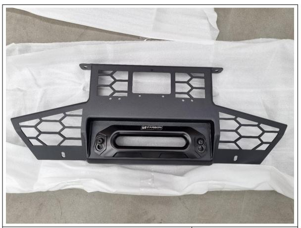
148. If required, fit the winch fairlead to the mesh fairlead mount using M10 or 3/8" fasteners supplied with the winch. This bar is only compatible with hawse type fairleads.
