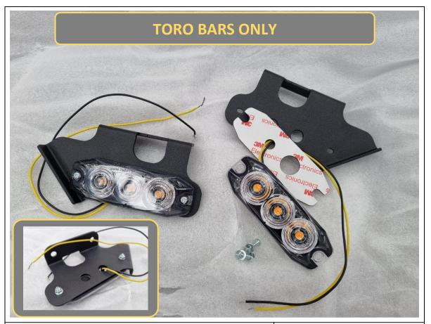
111. **Toro only.** Fit the supplied indicator repeaters to the mounting bracekts. Secure each indicator with 2x M3x12 pan head screws, flat washers and hex nuts.
