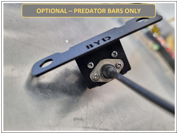
128. **Predator only (optional).** Fit the camera to the relocation bracket in the optional camera relocation kit using the original small Phillips head screws.
