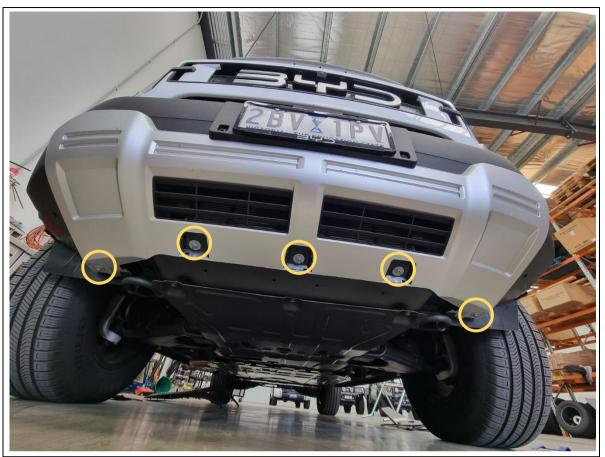
16. Remove 5x 10mm hex bolts along the bottom of the bumper.
