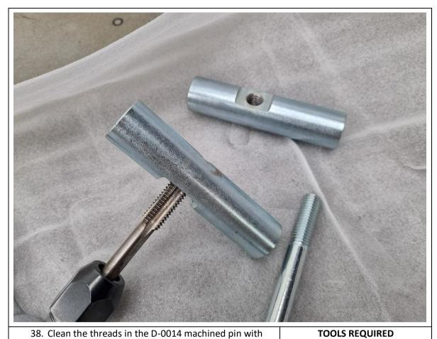
38. Clean the threads in the D-0014 machined pin with M12x1.75 coarse pitch tap if necessary.
