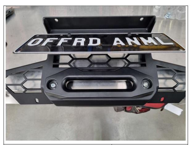
128. If required, fit the winch fairlead to the mesh fairlead mount using M10 or 3/8" fasteners supplied with the winch. This bar is only compatible with hawse type fairleads.
