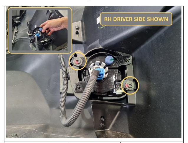
30. Time to strip the bumper. If equipped, remove 2x 10mm hex head screws securing each fog light on the back of the bumper.
