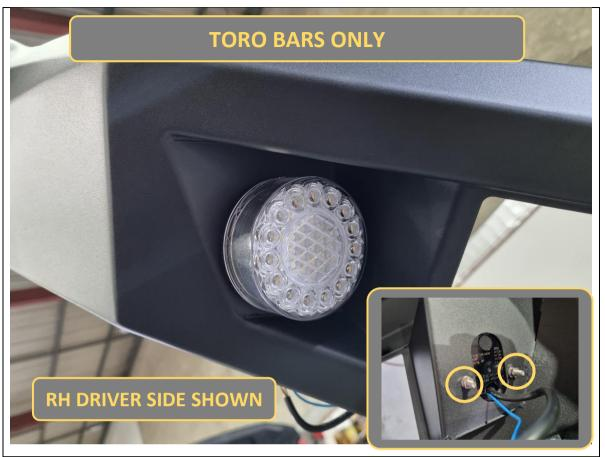
88. **Toro only.** Fit indicator units to the bar, using fasteners supplied with the indicator.
