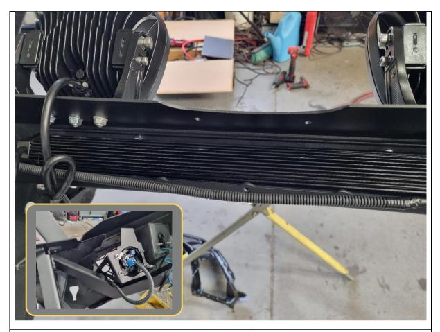
98. Route the bumper wiring harness through the inside of the bullbar.
