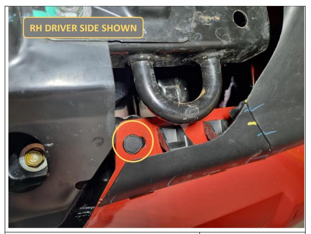
15. On the underside of the bumper, remove 2x plastic push clips holding the bumper to the inner bumper support brackets. These are located near where the factory tie down hooks are.
