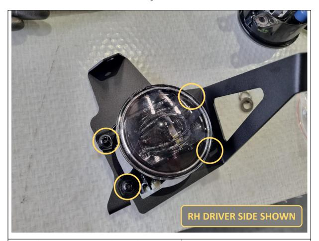
91. If equipped, unplug each fog light from the loom and then fit to the supplied mounting bracket and secure with 4x M6x16 black button head bolts, black washers and flange nuts.
