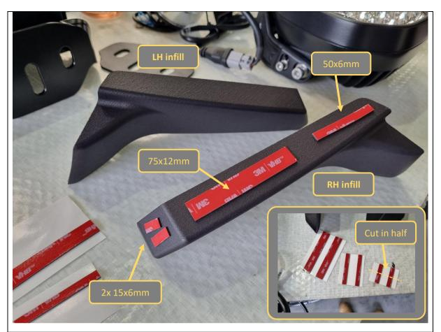
60. Apply supplied 3M VHB tape strips to the 2x headlight infills as shown. Cut the 30x6mm strips of tape in half to form 15x6mm strips.
