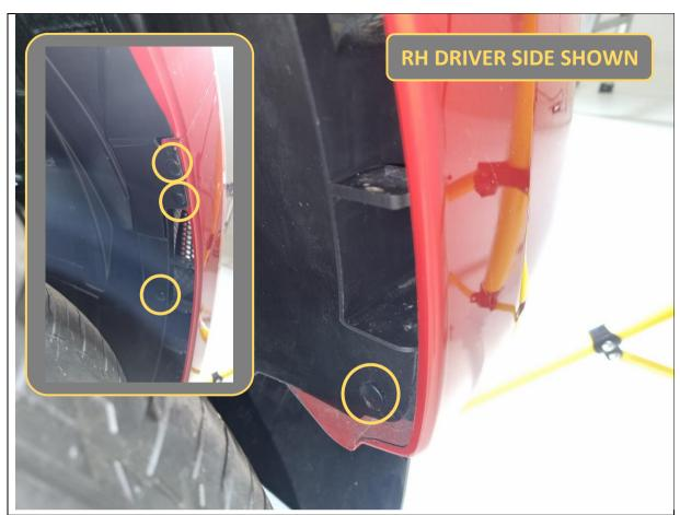
13. Remove 4x plastic push clips holding the wheel arch liner to the bumper, per side.
