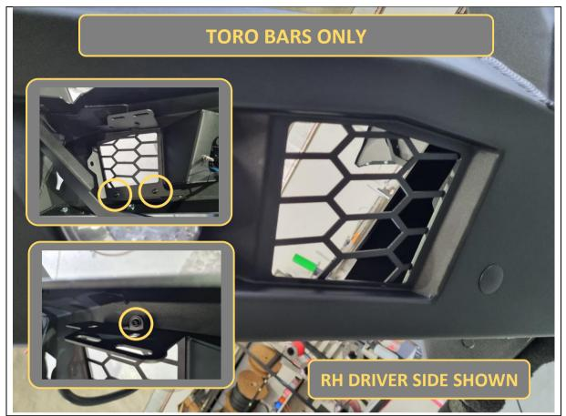
89. **Toro only.** Fit the M-0062 wing light meshes to the inside of each bull bar wing and secure with 3x M6x16 black button head bolts and black flat washers.
