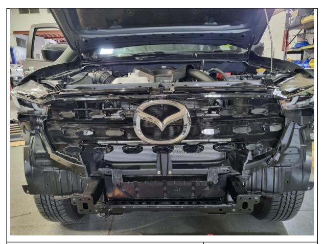
57. Re-fit the grille to the vehicle. Secure with the 7x plastic push clips and 1x Phillips head screw in Mazda badge removed previously.
