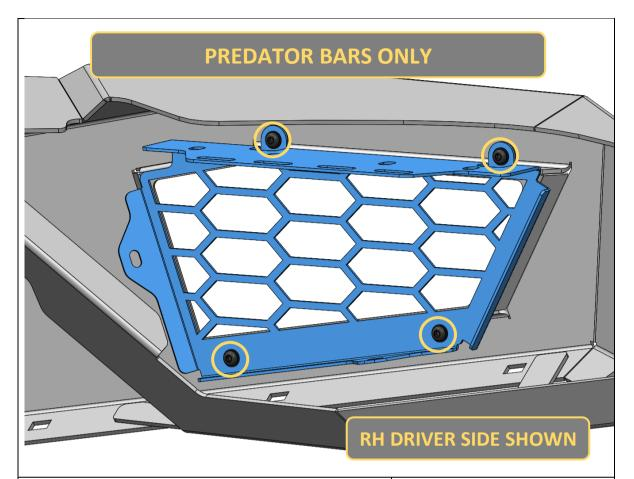
90. **Predator only.** Fit the M-0061 wing light meshes to the inside of each bull bar wing and secure with 4x M6x16 black button head bolts and black flat washers.
