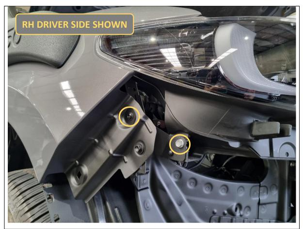
48. **Optional.** The metal guard underneath the headlight and quarter panel can be painted black. This is recommended on light-coloured vehicles, as the will be a gap between bull bar and headlight once fitted.
