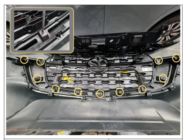
36. From the inside of the bumper, remove 11x Phillips head screws securing the black plastic grille inserts, as highlighted.
