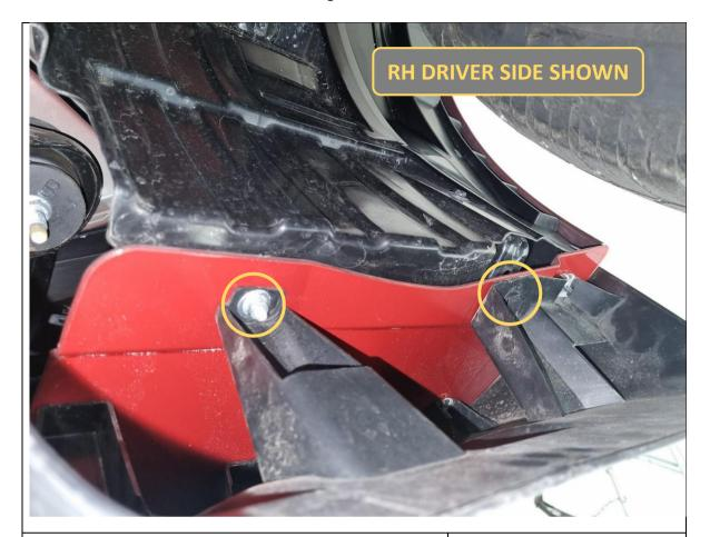
14. From below, remove 1x 10mm hex nut and 1x plastic push clip holding the bottom of the bumper to the wheel arch liner and outer bumper support bracket. Do this on both sides.
