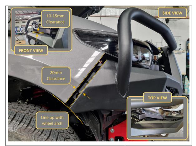
121. With assistance, from another person, align the bar with the edges of the vehicle. Adjust such that the clearances are neat, and the bar is symmetric left/right on the vehicle.
