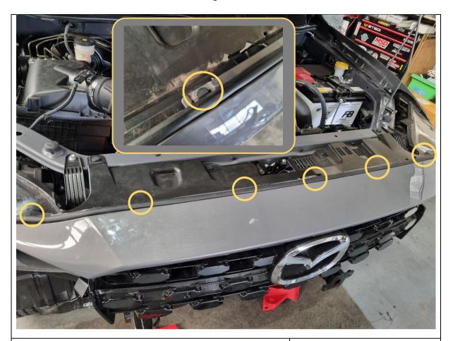
5. Remove 6x plastic push clips holding the upper grille lip. Move rubber seal aside to access.
