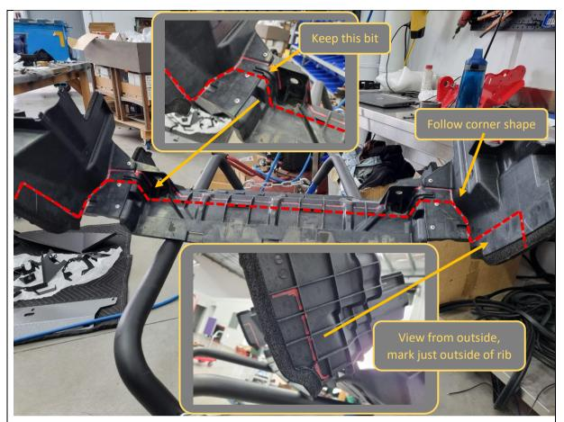
27. Use a marker pen and mark a cut line on the air guide, as shown.
