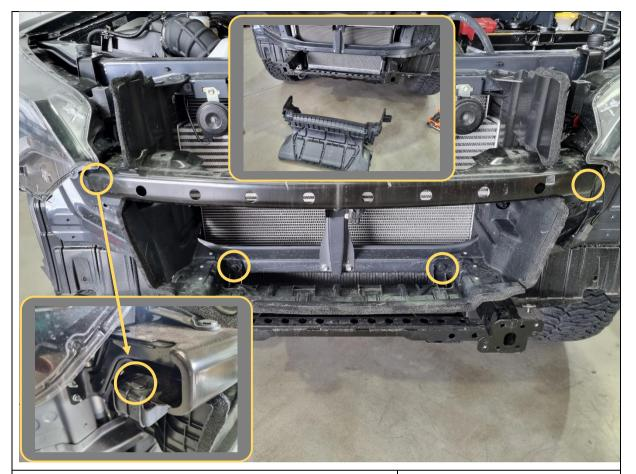
25. Remove the 4x plastic push clips holding the lower plastic air guide.
