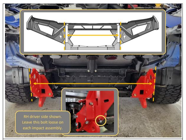
75. Measure the distance between the outside faces of uprights on bar using tape measure. Write distance below for reference if required.
