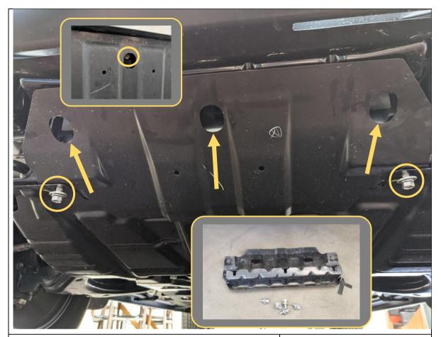
19. Remove the front skid plate by removing the 5x 14mm hex bolts securing it to the chassis. Retain the bolts for use later.
