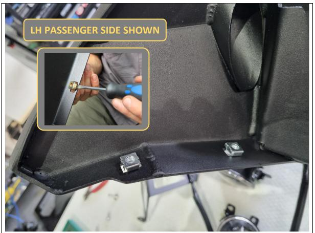
83. Fit 12x M6 cage nuts into the rectangular slots in bottom of wing (6x per side).
