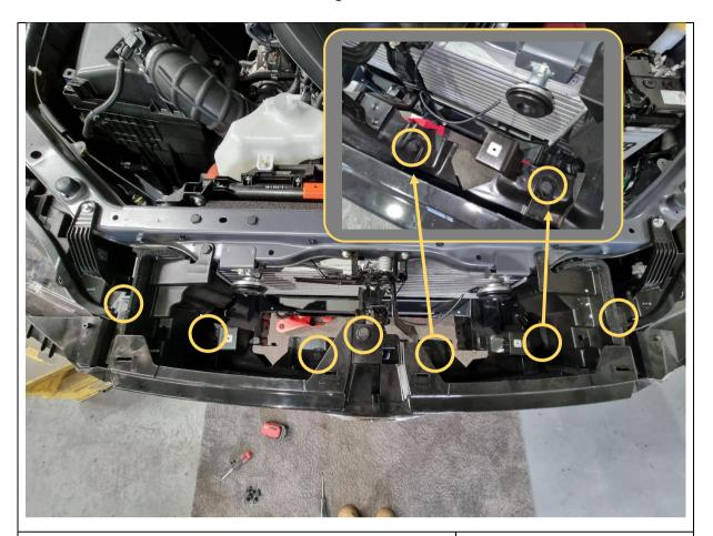
11. Remove 7x plastic push clips holding the grille. There are 3x clips on the top edge, and 4x clips on the cross member on the inside of the grille (see insert photo).
