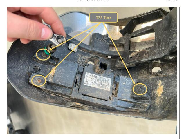
18. Before removing the Radar it is helpful to mark L&R sides to aid in re-fitment to bar
