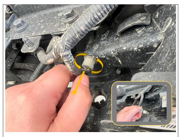
9. Disconnect the Number plate lamp connectors. Twist to unlock then remove.
