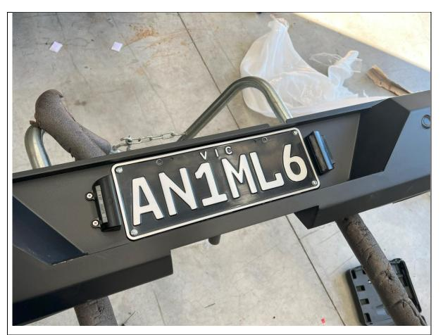
55. Re-Fit number plate to the bar, using supplied M5 Fasteners.
