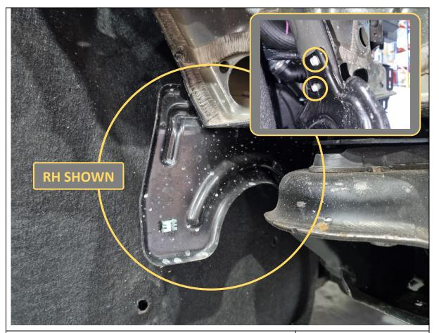
40. Unbolt and remove the 2x inner wheel guard support brackets using a 10mm socket/spanner.
