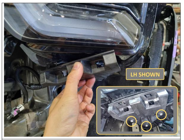
41. Unbolt and remove the plastic bumper clip under each headlight using a **T20** Torx driver.
