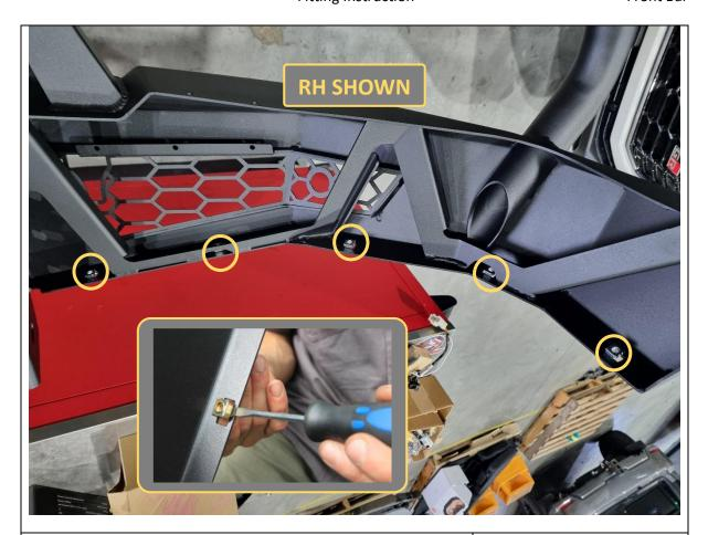
88. Fit 5x M6 cage nuts into the rectangular slots on the bottom of the bar wing.
