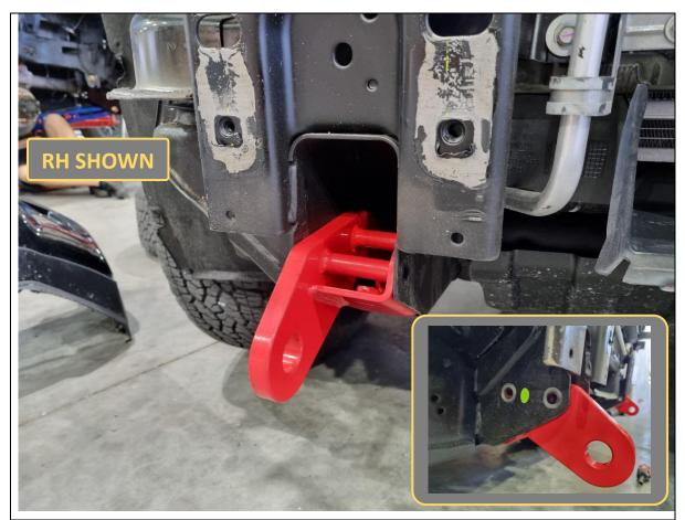
24. Firmly insert the supplied red tow points into the chassis rail ends. Align the 2x bolt holes on the side with the holes in the chassis rail.
