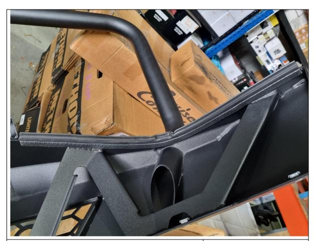
92. Fit the 2x supplied 500mm lengths of top bulb pinch weld to the top edge of each bullbar wing.
