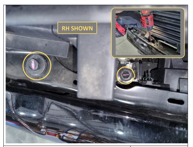
18. Looking down on the top lip of the bumper, remove 4x 18mm hex bolts securing the top bumper support brackets.
