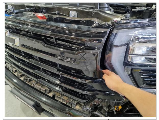
14. Pull outwards and release the clips securing the grille to the vehicle. Set aside in a safe place for later.
