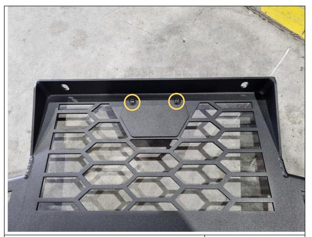
97. If not relocating the front camera, bolt the blanking plate onto the front of the mesh fairlead, and secure with 2x M5x20 black button head bolts, flat washers and flange nuts.
