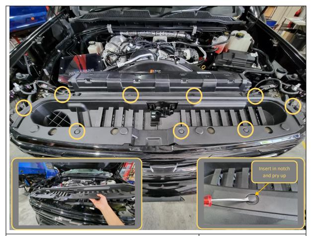
5. Remove the radiator grille cover by removing 9x plastic push rivets. To remove each push rivet, lever the centre section upwards using a flat blade screwdriver or trim tool, as shown.
