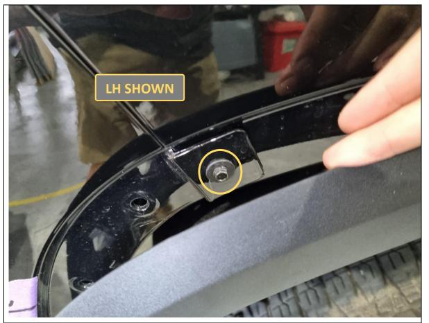
8. Remove 1x 7mm hex bolt hiding under the flare which is securing the plastic bumper to the metal fender guard. Do this for both sides.
