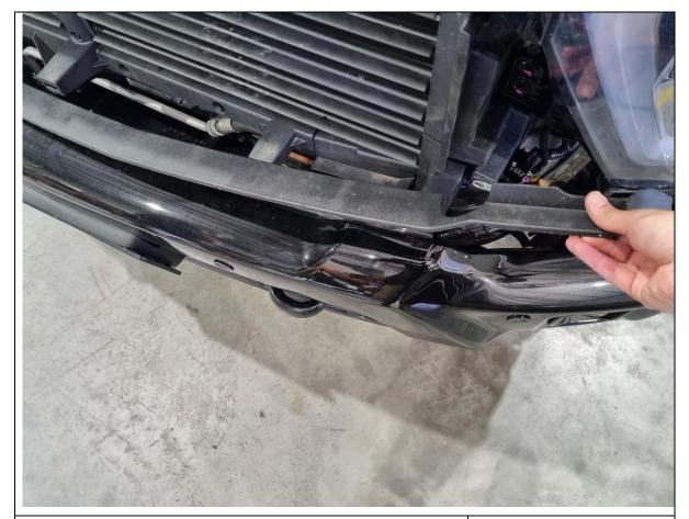
15. Unclip the plastic spoiler running along the top lip of the steel bumper.
