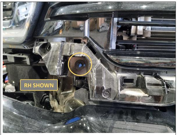
11. Remove 2x 10mm hex bolts (1x per corner) securing the bottom of the grille.
