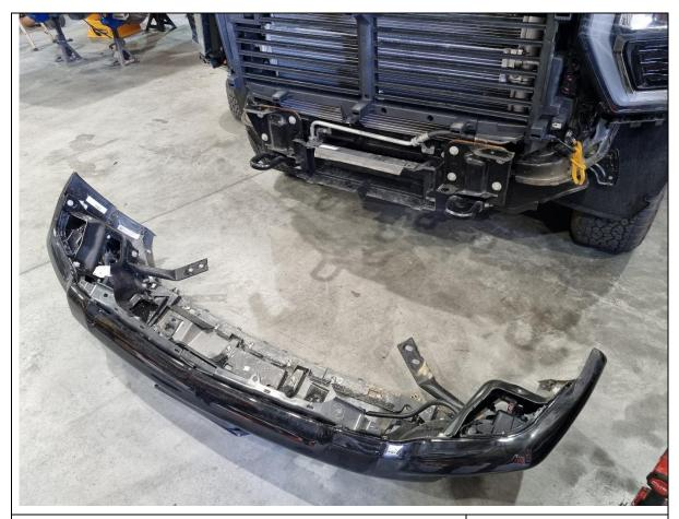
19. With assistance, either from another person or mechanical lifting device, remove the steel bumper and set aside in a safe place.
