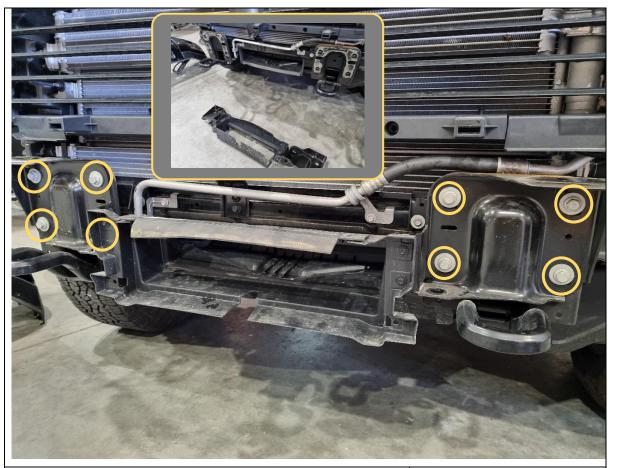
20. Remove 8x 15mm hex bolts (4x per side) securing the bumper brackets and intercooler shroud to the chassis. Retain fasteners for re-use.
