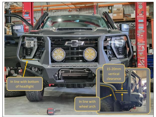
98. With assistance, from another person, align the bar with the edges of the vehicle. Adjust such that the clearances are neat, and the bar is symmetric left/right on the vehicle.
