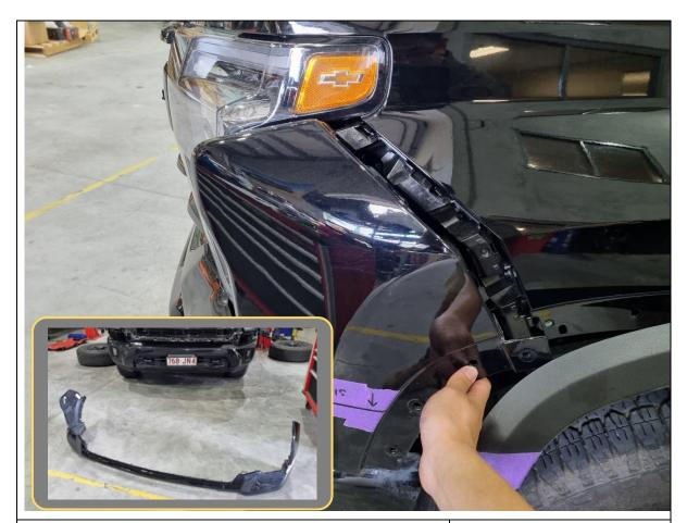
9. Starting from the outer tips, pull outwards and release the clips holding the plastic bumper to the vehicle.
