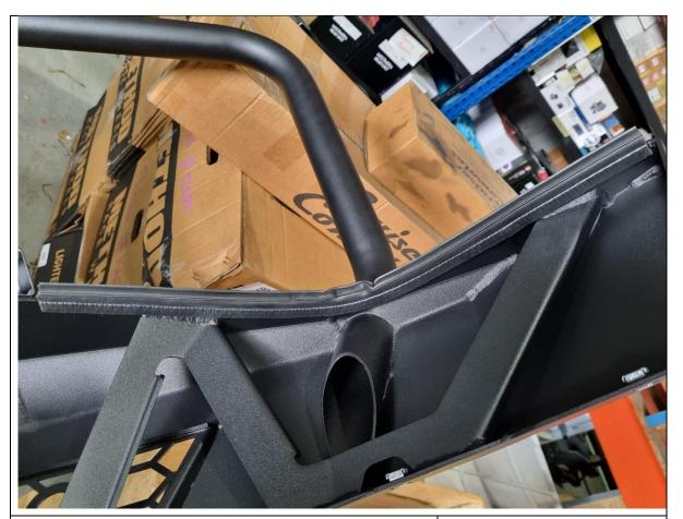
85. Fit the 2x supplied 500mm lengths of top bulb pinch weld to the top edge of each bullbar wing.
