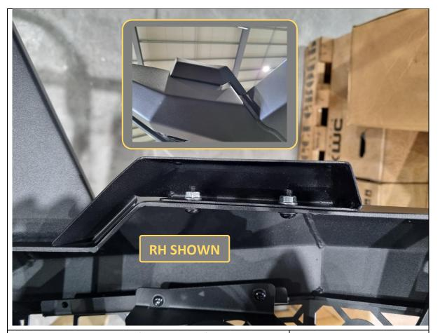
83. Fit the B-1192 grille infills to the top of the bullbar.
