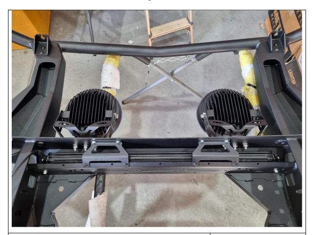
80. If fitting driving lights or top hoop to this bar, this is also the most convenient time to do so. It is still possible later but is more difficult.
