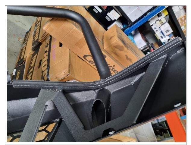
83. Fit the 2x supplied 500mm lengths of top bulb pinch weld to the top edge of each bullbar wing.
