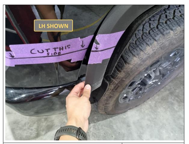
7. Starting from the front bottom corner, pull outwards and release the clips holding the front half of the fender flare. Let it hang off the side of the vehicle. Do this for both sides.
