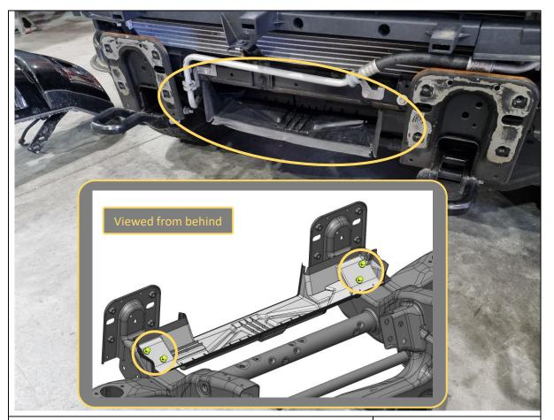
23. Remove the 4x plastic push rivets (2x per side) securing the air dam to the chassis.
