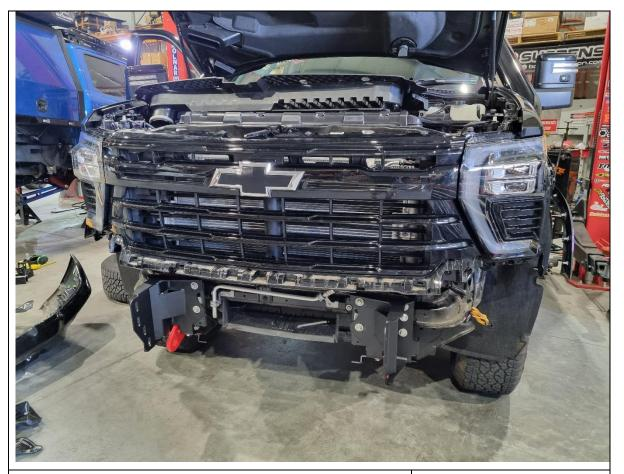
45. Refit the grille, radiator grille cover, and bonnet release handle to the vehicle in reverse order. Also re-connect the camera harness if the camera is remaining in the grille.
