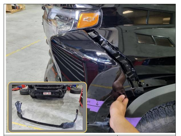
9. Starting from the outer tips, pull outwards and release the clips holding the plastic bumper to the vehicle.
