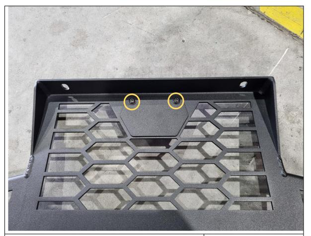
97. If not relocating the front camera, bolt the blanking plate onto the front of the mesh fairlead, and secure with 2x M5x20 black button head bolts, flat washers and flange nuts.
