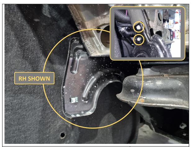
40. Unbolt and remove the 2x inner wheel guard support brackets using a 10mm socket/spanner.
