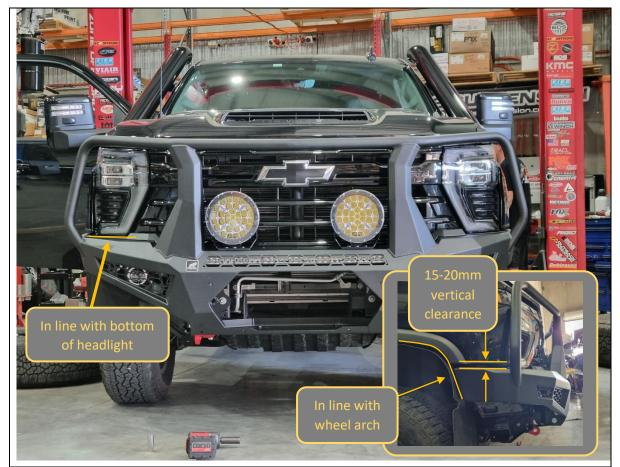
89. With assistance, from another person, align the bar with the edges of the vehicle. Adjust such that the clearances are neat, and the bar is symmetric left/right on the vehicle.
