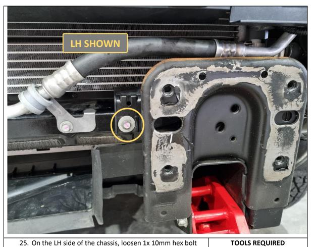
25. On the LH side of the chassis, loosen 1x 10mm hex bolt securing the plastic bracket. Manipulate it out of the way in preparation for fitting the chassis brace in the next step.
