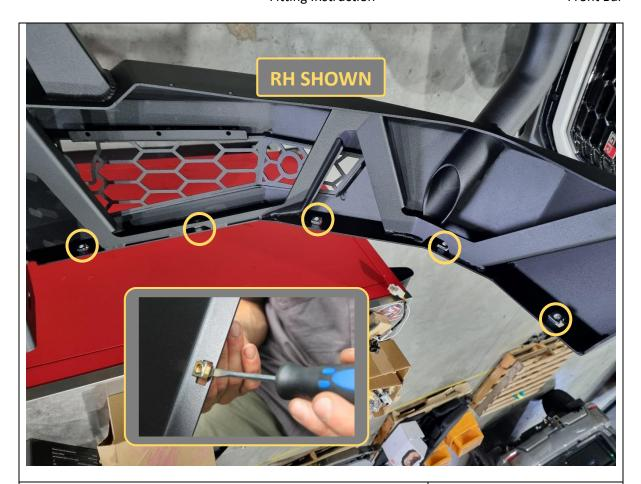
79. Fit 5x M6 cage nuts into the rectangular slots on the bottom of the bar wing.
