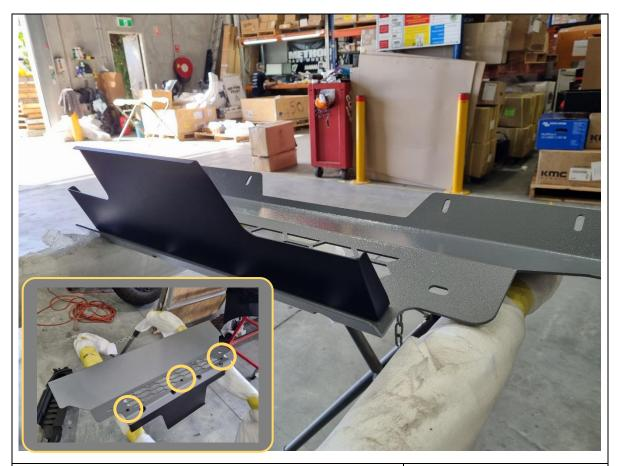
108. Bolt the air guide to the bash plate and secure using 3x M6x16 black button head bolts, black washers and flange nuts.
