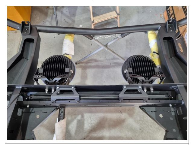
78. If fitting driving lights or top hoop to this bar, this is also the most convenient time to do so. It is still possible later but is more difficult.
