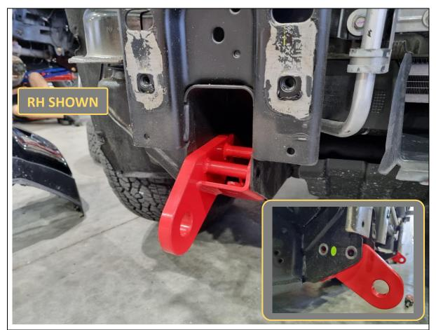
24. Firmly insert the supplied red tow points into the chassis rail ends. Align the 2x bolt holes on the side with the holes in the chassis rail.
