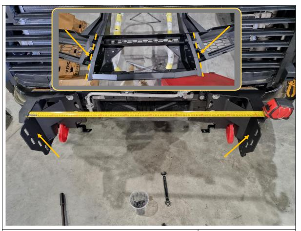
37. Measure the horizontal distance between the outside faces of uprights on bar using tape measure. Write distance below for reference if required.
