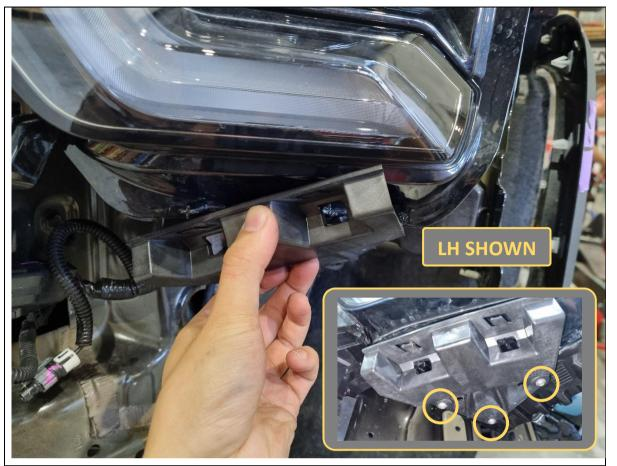
41. Unbolt and remove the plastic bumper clip under each headlight using a **T20** Torx driver.
