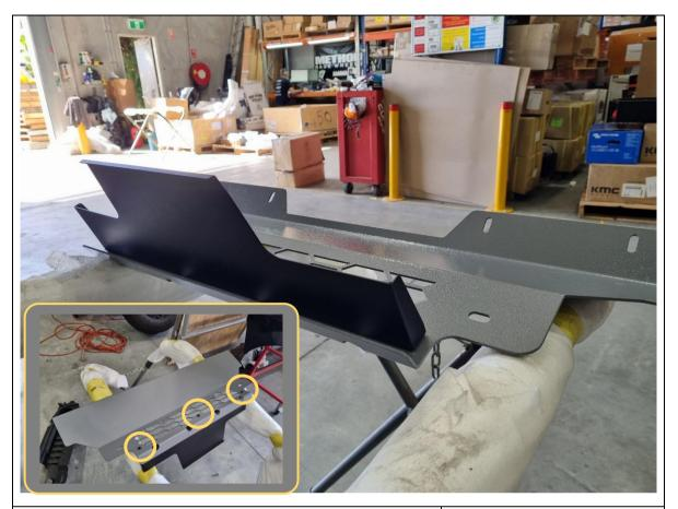
127. Bolt the air guide to the bash plate and secure using 3x M6x16 black button head bolts, black washers and flange nuts.
