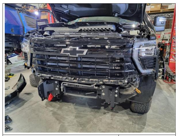
45. Refit the grille, radiator grille cover, and bonnet release handle to the vehicle in reverse order. Also re-connect the camera harness if the camera is remaining in the grille.
