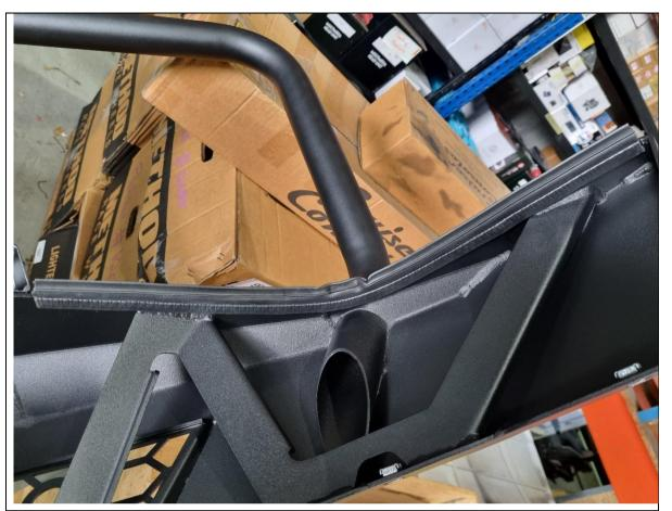
102. Fit the 2x supplied 500mm lengths of top bulb pinch weld to the top edge of each bullbar wing.
