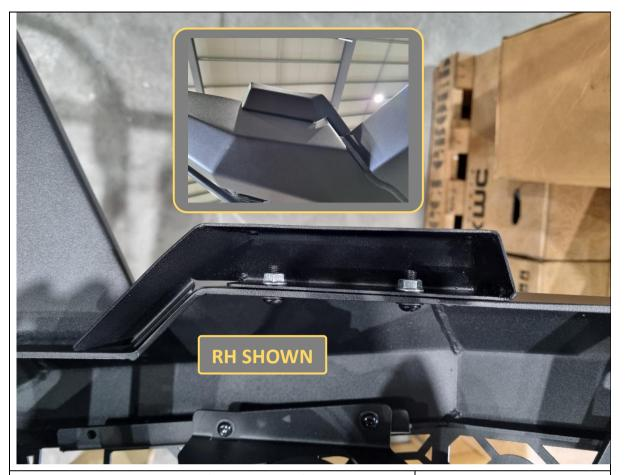
100. Fit the B-1192 grille infills to the top of the bullbar.
