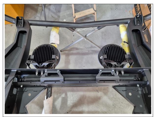
97. If fitting driving lights or top hoop to this bar, this is also the most convenient time to do so. It is still possible later but is more difficult.
