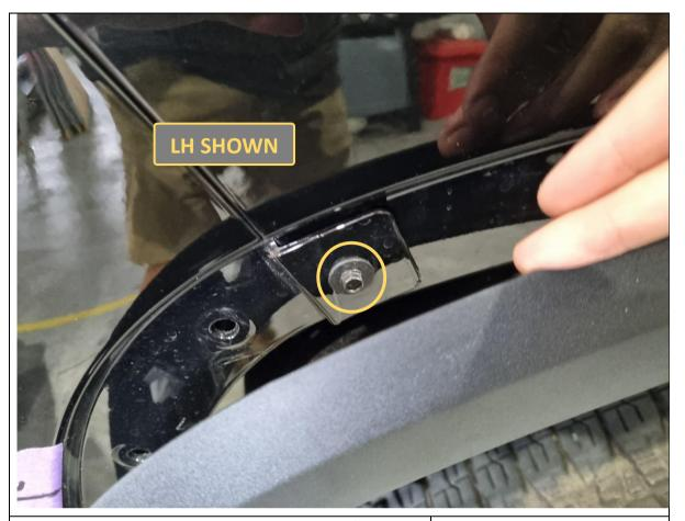
8. Remove 1x 7mm hex bolt hiding under the flare which is securing the plastic bumper to the metal fender guard. Do this for both sides.
