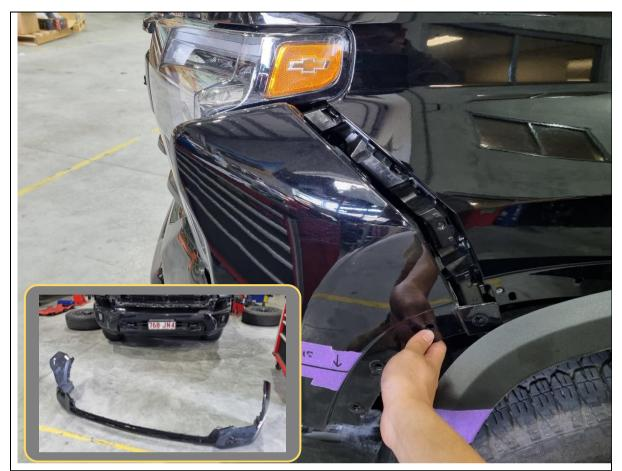
9. Starting from the outer tips, carefully pull outwards and release the clips holding the plastic bumper to the vehicle.
