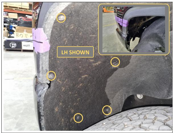
6. Remove multiple plastic push rivets and T15 Torx screws to remove and pull away the front half of the inner wheel arch liner. Do this for both sides.
