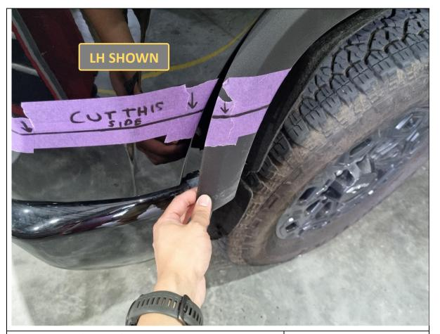
7. Starting from the front bottom corner, pull outwards and release the clips holding the front half of the fender flare. Let it hang off the side of the vehicle. Do this for both sides.
