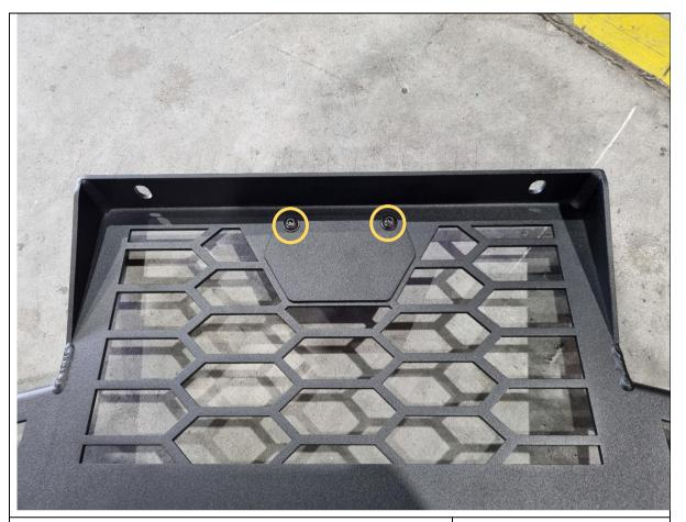
116. If not relocating the front camera, bolt the blanking plate onto the outside of the mesh fairlead, and secure with 2x M5x20 black button head bolts, flat washers and flange nuts.
