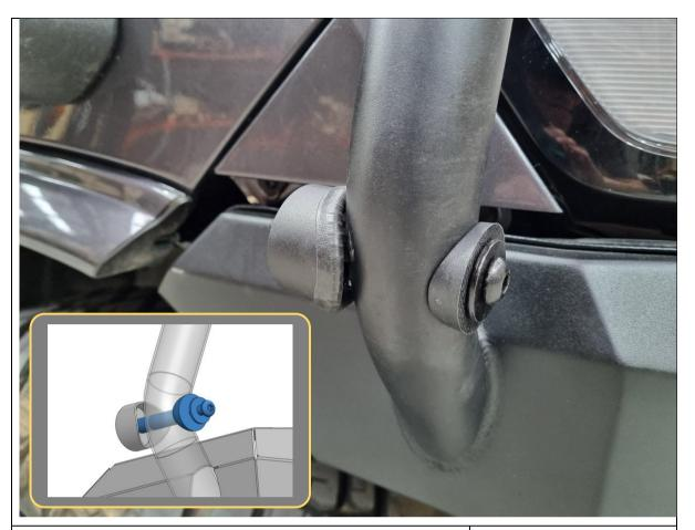
17. Loosely position the spigot with the Toro bar and hold in place with 1x M10x100 black button head, flat washer, nylon saddle washer and crush tube, through the 18mm drilled hole in the bar.
