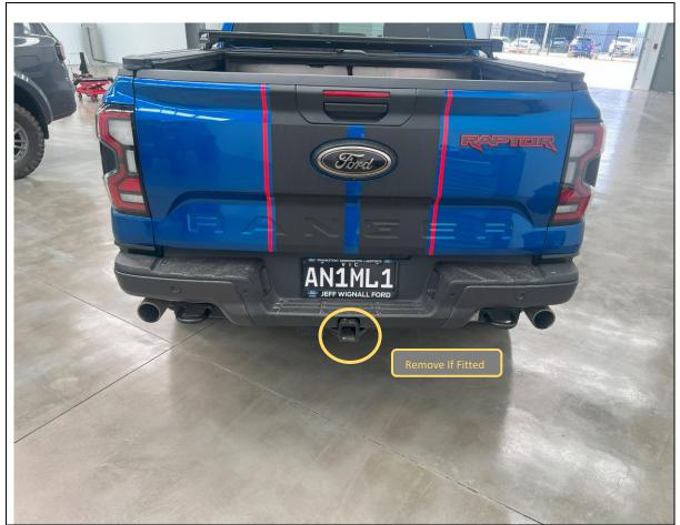
1. Before beginning work, remove factory TBM if fitted for easier access. 17mm spanner may be required to loosen anti rattle bolt on bottom of hitch.
