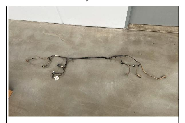
15. Unclip and remove wiring loom from original rear bar. Place aside in safe location for refitment to Offroad Animal Bar.
