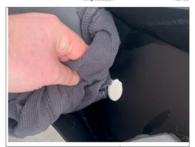
16. Clean areas adjacent to parking sensor locations on inside of bar with isopropyl alcohol.
