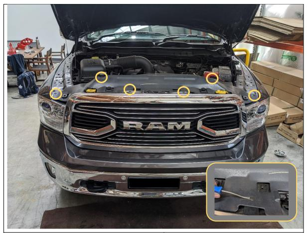
**NOTE:** The following steps show the removal of the split chrome type bumper as fitted to Laramie Models.
