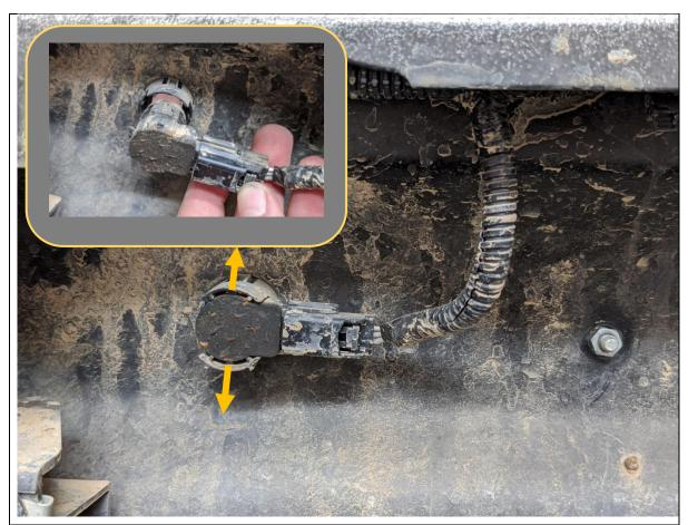
34. Remove parking sensors from housings. Gently pry apart housing, using a small flat screwdriver whilst pushing sensor through from the front side of the bar to release them.
