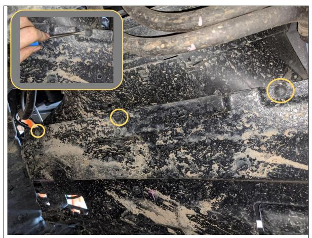
23. From underneath the car, remove the 3x Xmas Tree clips that secure the air guide from the radiator shroud using a trim tool.
