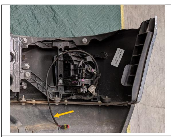
42. Remove the Parker light plug by cutting off close to factory parker location for re use on Offroad Animal Bar
