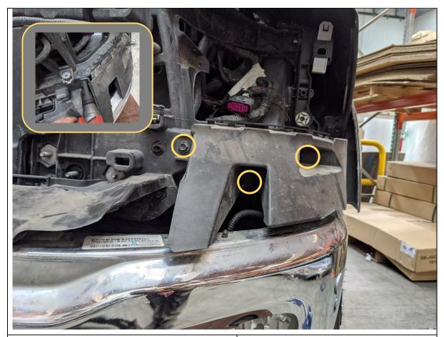
20. Remove the outer plastic bumper supports by removing the 3x 10mm head screws securing it to the crossmember.
