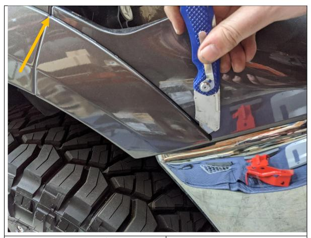
16. Using a Utility knife carefully cut the double-sided adhesive tape securing the wheel arch flare back to the bumper to guard joint in the body.
