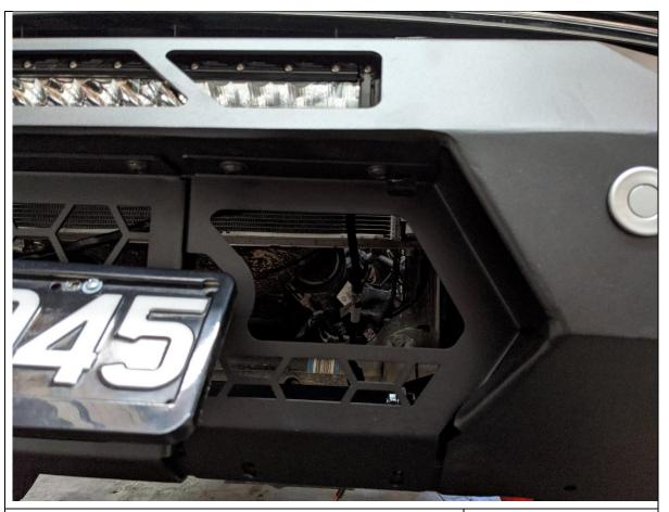
99. Fit Mesh Infill Panels. Use 2x M8x16 Button head bolt, M8 flat washer and M8 flange nut for top mount
