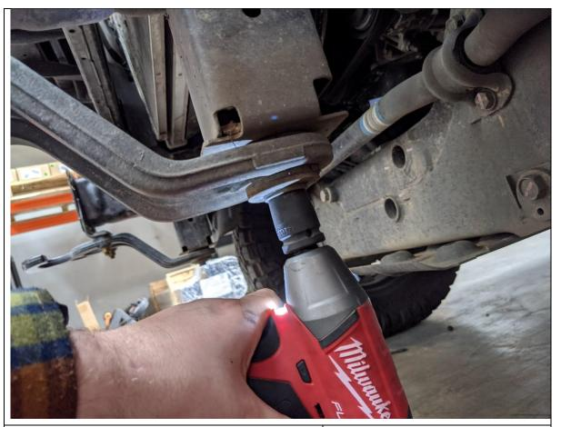
30. Remove the factory tow hooks, by removing the M12 Fine pitch bolt securing it to the chassis.
