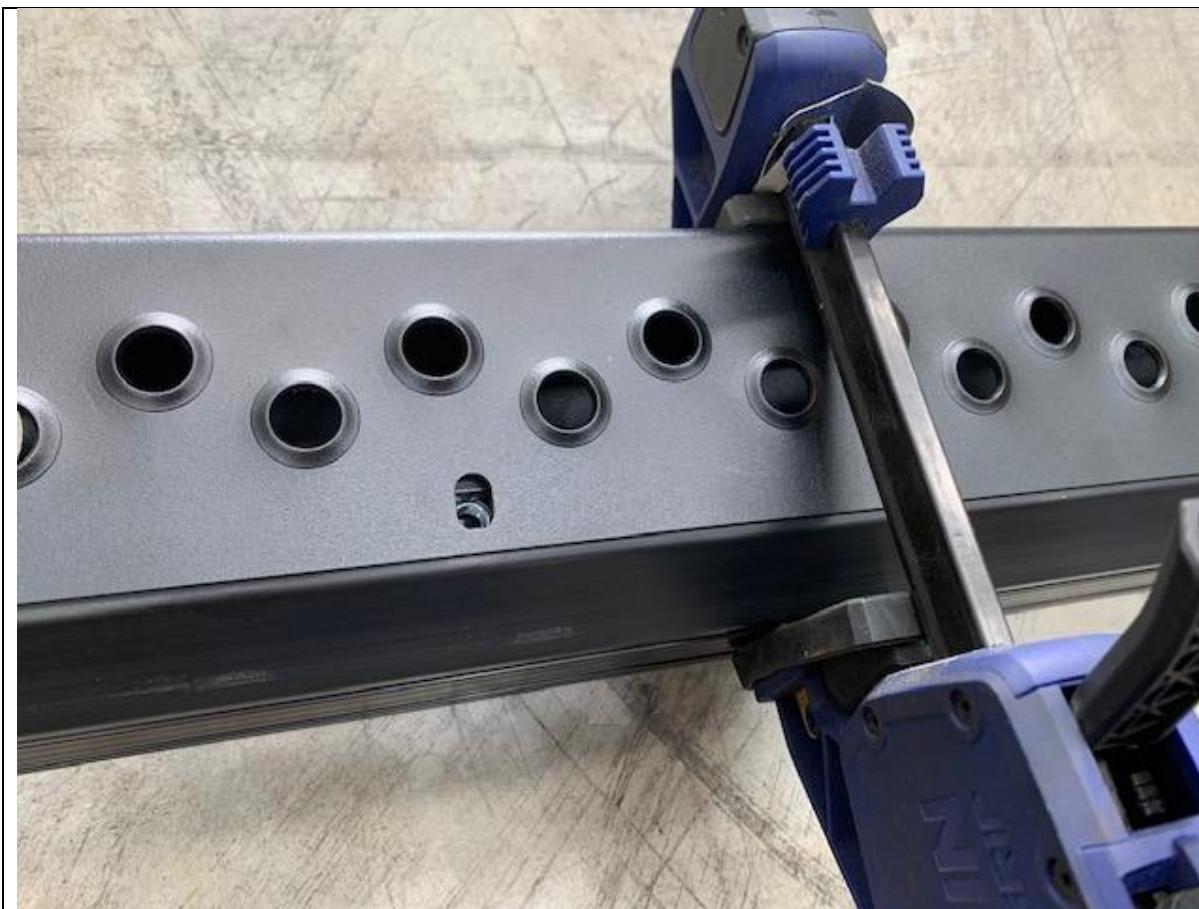
32. Using long tool feed nuts in to centre first and thread in with black M8 button head cap screws and washers.
