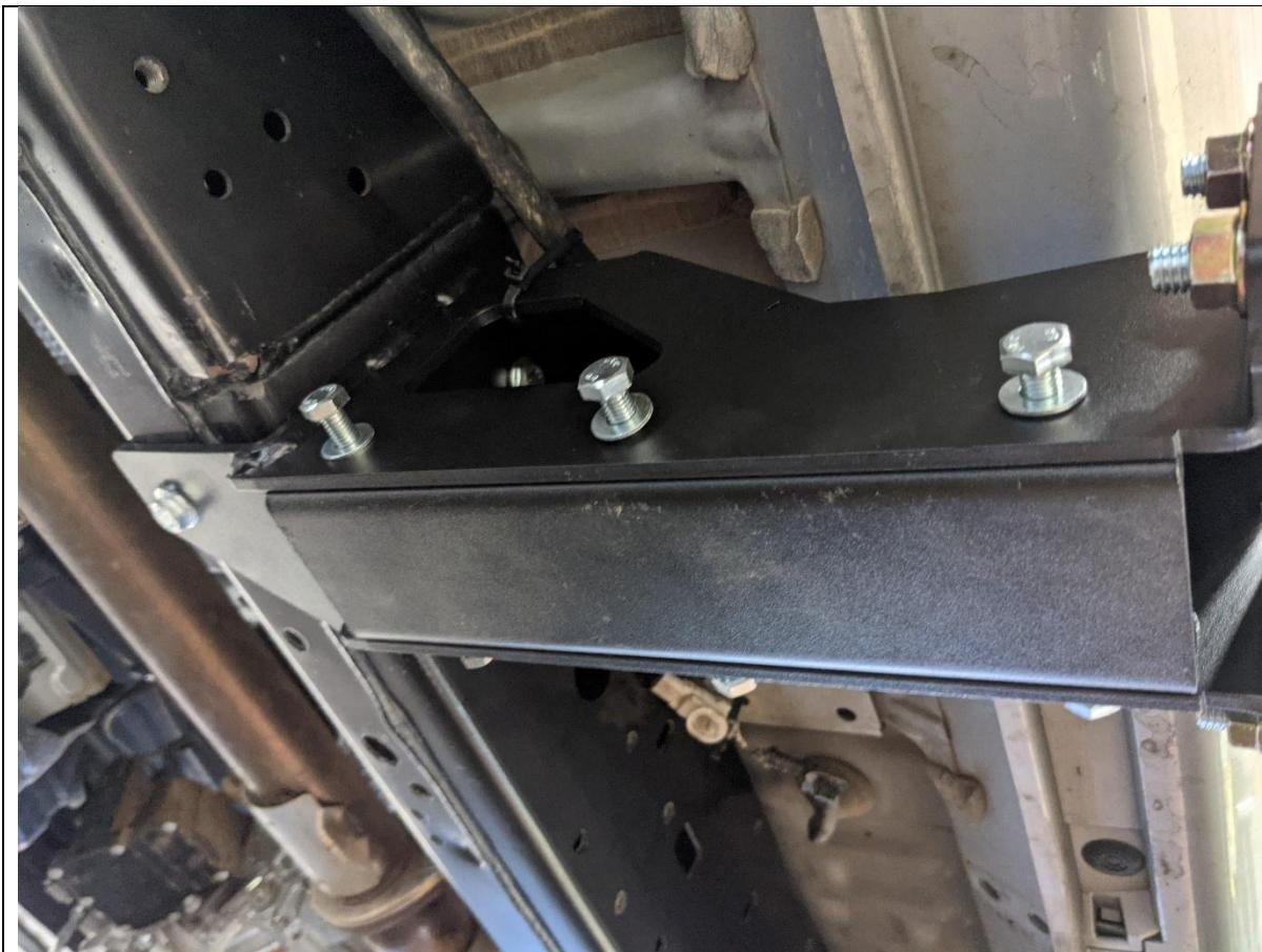
48. Check all fasteners Securing the mounts to the chassis rail are tight.
