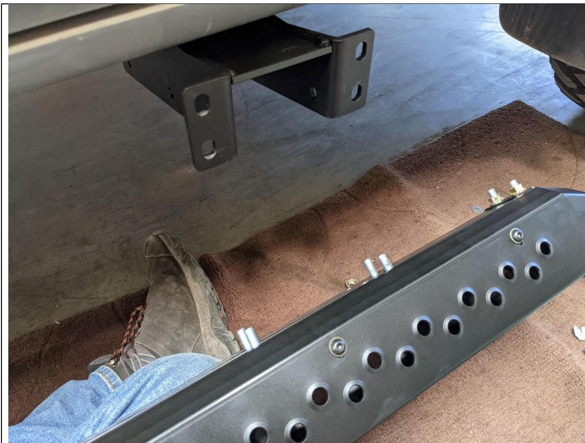
42. With Assistance from another person, or mechanical lifting aid such as a lift trolley, Lift the slider onto the mounts.
