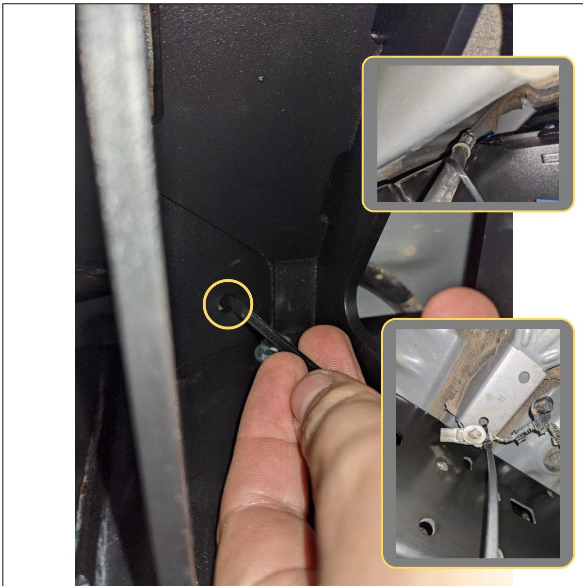
47. Secure Hand Brake cable and under step wiring harness with cable ties as shown in images.
