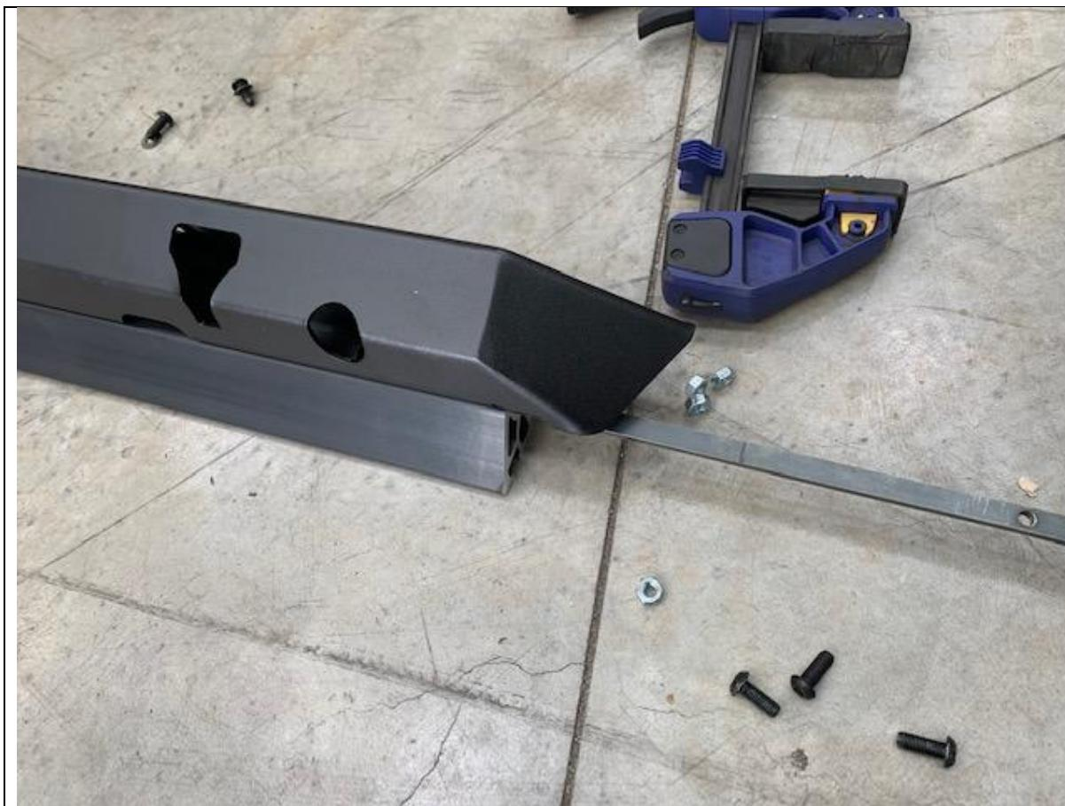
27. Lie extrusion down and place step on top.
