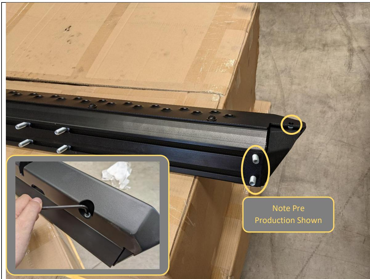
39. Fit mirrored end cap to remaining end of slider, using 2x M10x16 Button bolts and M6x20 Button head bolt with flat washer as per previous steps 34-36.
