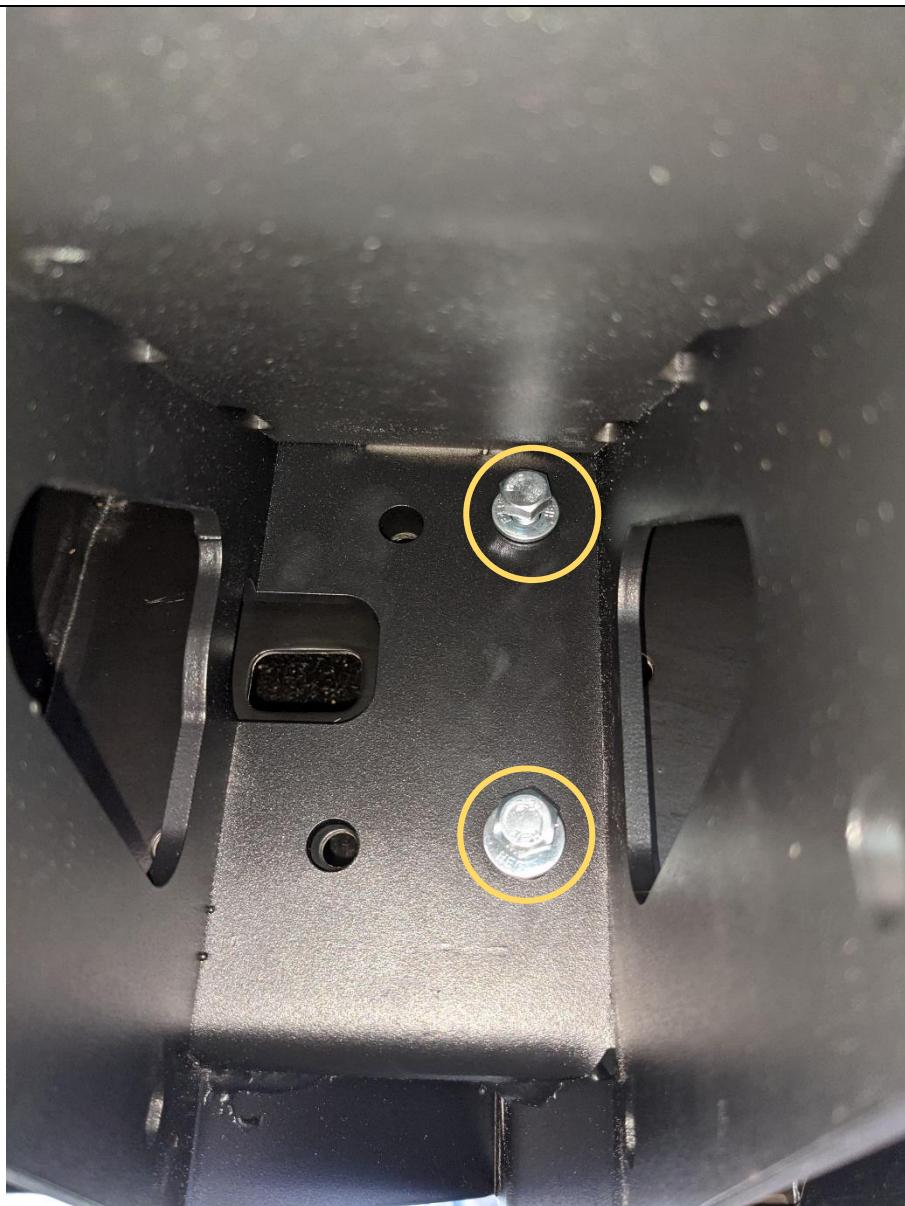
6. Fit the front mount, to the chassis using M8x20 bolts, HD flat washers, Secure finger tight only at this stage
