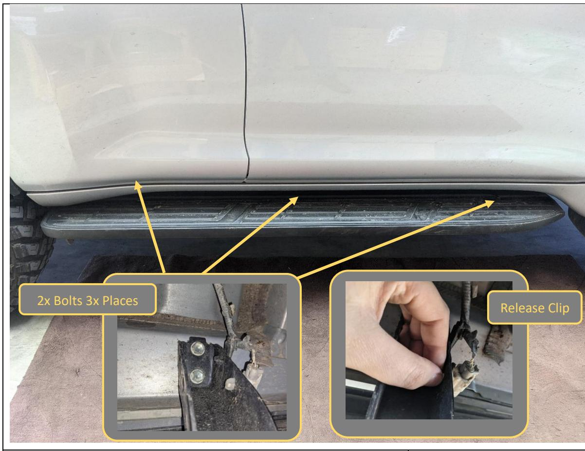
1. Remove Factory side steps if fitted by removing the 6x Bolts (2 Per mount) securing them to the body using a 12mm socket.
