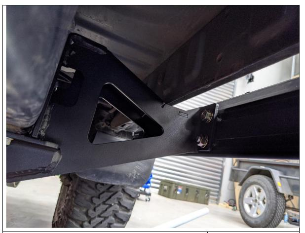
40. Tighten all mount to slider M10 flange nuts using 15mm spanner. A ratcheting spanner makes this process easier.
