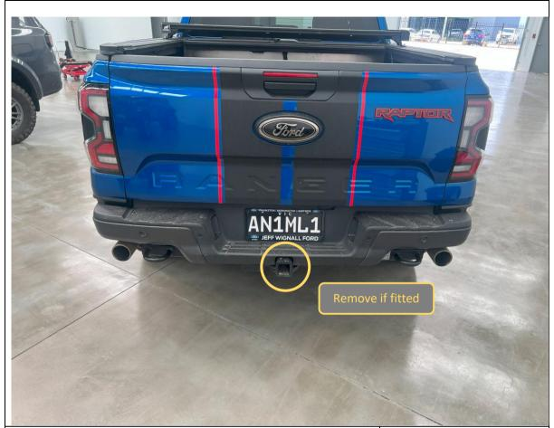
1. Before beginning work, remove factory tow ball mount if fitted for easier access. 17mm spanner may be required to loosen anti rattle bolt on bottom of hitch.
