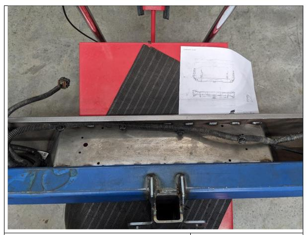
19. Fit the harness to the rear bar, routing the cables through the side arms so that the sensor wiring positions are in the correct locations. Ensure the correct orientation of the harness connectors in maintained.
