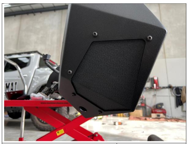
20. Fit plastic radar windows to the opening in the wing of the rear bar, using supplied M6x16 black bolts, Flat washers, and flange nuts.
