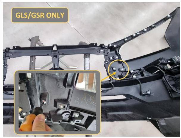
108. **GLS/GSR only.** Remove 2x Phillips pan head screws on the inside of the bumper, per side.
