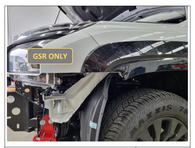
118. **GSR only.** Re-fit the trimmed flares and re-secure with fasteners/clips removed in Steps 17 and 18.
