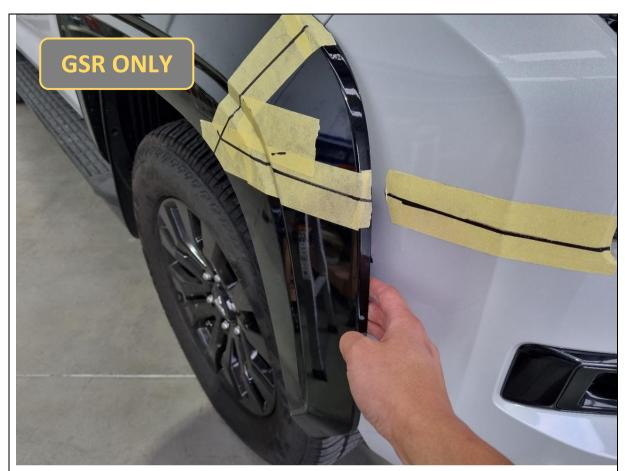
19. Gently pull outwards from the two ends to release the clips holding the flare. Set aside for later.
