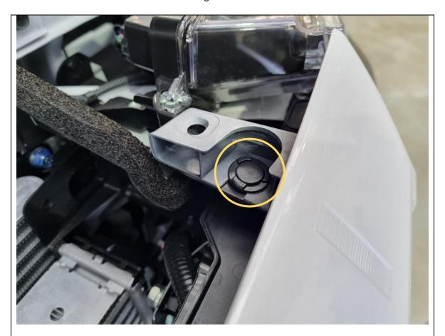
12. Remove 2x plastic push clips (1x either side) on the top of the grille.
