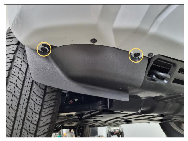
23. Remove the 2x plastic push clips securing the outside bumper (per side).
