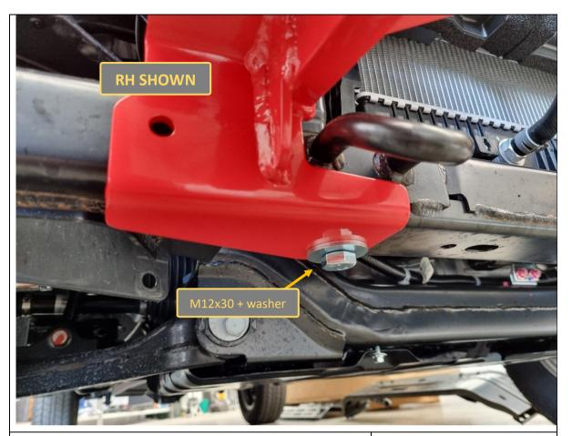
52. Loosely secure the bottom of the tow point with 1x M12x30 hex bolt and heavy duty washer to the M12 nutplate installed previously. Leave finger tight.
