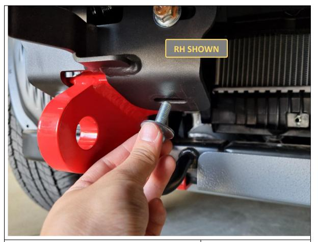
162. Loosen the lower inner M10x30 hex bolts on the impact assemblies in preparation for fitting main bash plate.
