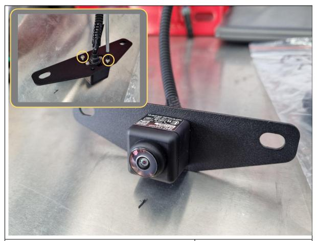
152. Use a precision (jewellery) Phillips head screwdriver to secure the 2x tiny screws holding the camera to the front of the camera mount plate.
