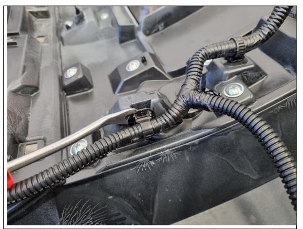
73. Unclip the complete harness from the bumper and set aside, with radars and parking sensors attached. Take care not to drop or impact any of the components. Take note of harness orientation.
