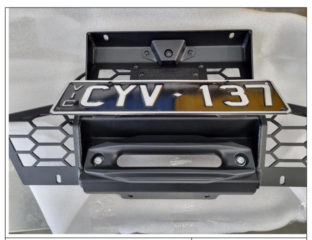
157. If required, fit the winch fairlead to the mesh fairlead mount using M10 or 3/8" fasteners supplied with the winch. This bar is only compatible with hawse type fairleads.
