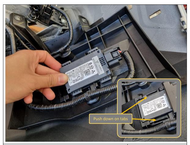
71. Push down on the plastic tabs, then slide the ICA radar outwards and off the bumper. Take note of the orientation of each radar unit and its plug direction before fully removing.
