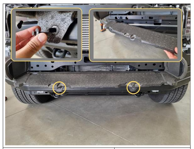
35. Remove 2x plastic scrivets securing impact foam with a Phillips head screwdriver, then remove impact foam.
