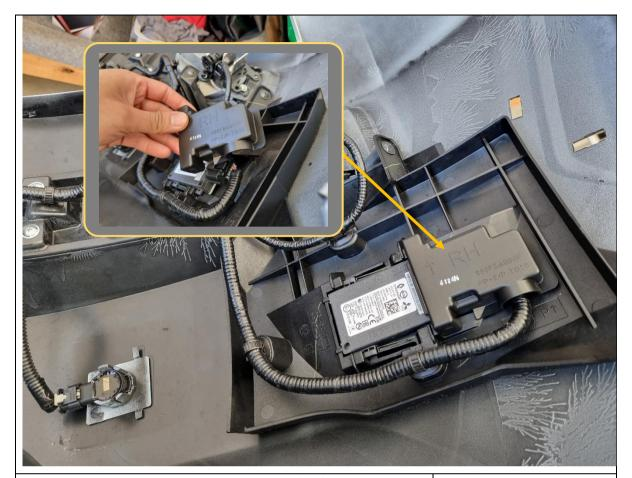
70. Unclip the intersection collision assist (ICA) radar plug plastic cover.
