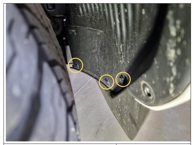
22. Remove the 3x plastic push clips securing bumper to the lower edge of the wheel arch liner (per side).
