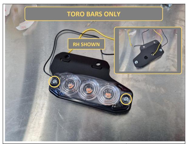
75. Fit the supplied indicator repeater lamps to the indicator brackets, using 2x M3 Phillips head screws and the adhesive backing included with the lamp module. Do this with both brackets.
