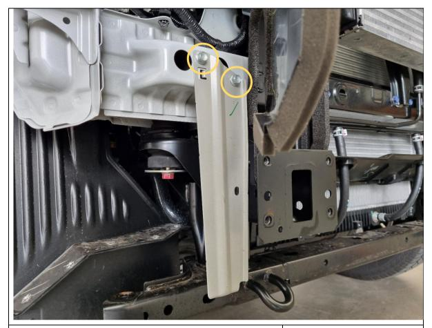
45. Remove 2x 12mm hex bolts securing the bumper support bracket to the chassis. Discard the bracket. Repeat for other side.
