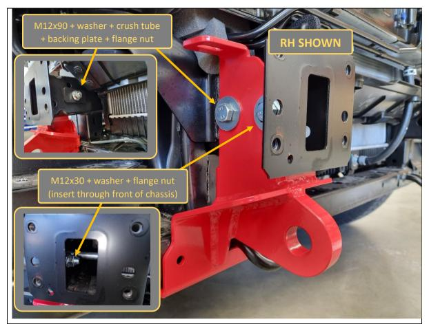
51. Fit the tow point onto the outside face of the chassis rail, then loosely secure with fasteners as shown above. Leave finger tight.
