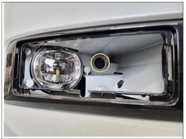
31. Remove 1x 10mm hex bolt securing the bumper to the body, next to the fog light. Do this on both sides.
