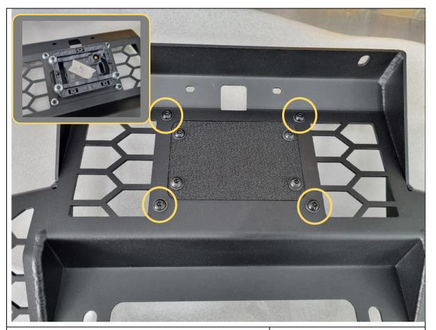
151. Fit the radar and mount through the open window in the mesh fairlead and secure with 4x M6x16 black button head bolts, black washers and flange nuts.
