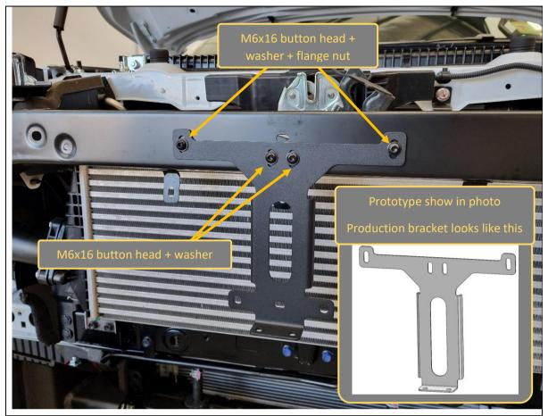
67. Fit the grille brace bracket to the upper body frame. Secure with 4x M6x16 black button head bolts, black washers and flange nuts.
