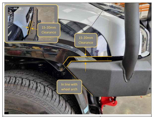
142. With assistance, from another person, align the bar with the edges of the vehicle. The bar should sit symmetric left/right on the vehicle.
