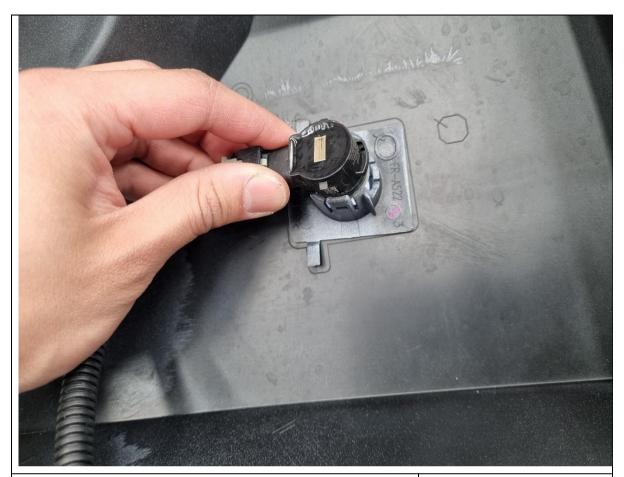
72. Unclip all 4x parking sensors from the bumper. Take note of the orientation of each parking sensor and its plug direction (i.e. in/out).
