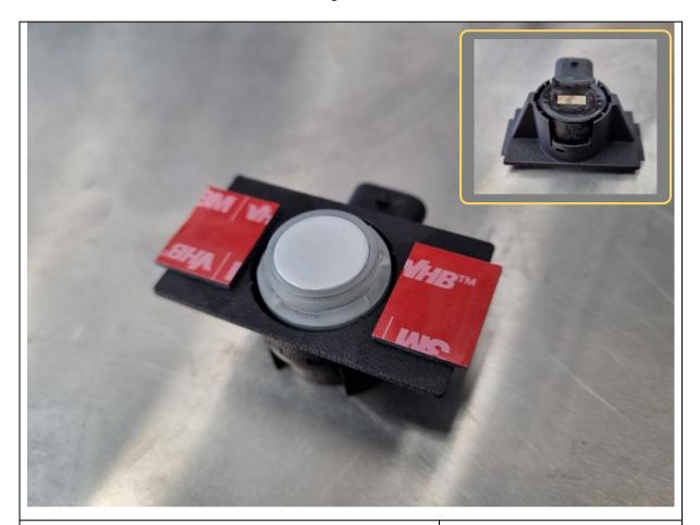
98. Fit parking sensors into plastic sensor housings.
