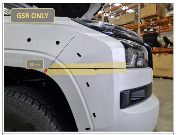
21. Finish marking the bumper cut line over the area previously hidden by the flare. Check with 30mm reference point from wheel arch liner and re-mark line if necessary.
