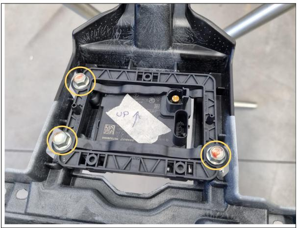
74. Remove 3x 10mm hex bolts securing the middle ACC radar on the bumper. Take note of the radar orientation before removing. Do not drop or impact the radar unit.
