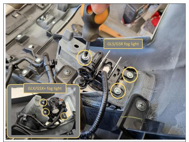
69. Remove the 3x screws holding each fog light to the stock plastic bumper with a Phillips head screwdriver.
