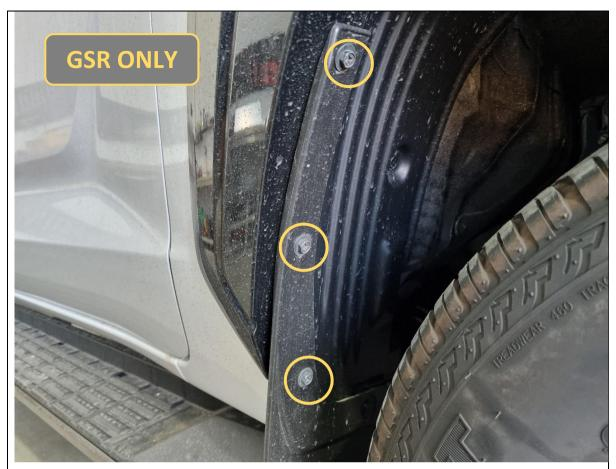
17. Remove 3x 10mm hex bolts holding the rear of the flare and mudflap.
