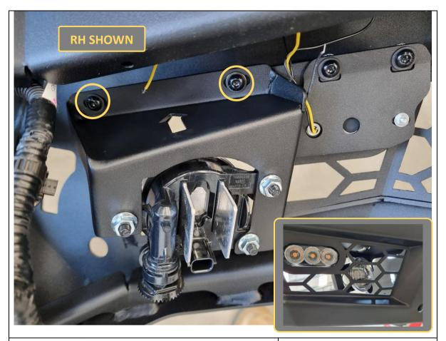
86. Fit the fog lights and brackets to the bullbar using 2x M16x16 black button head bolts, 2x black flat washers and 2x flange nuts each.
