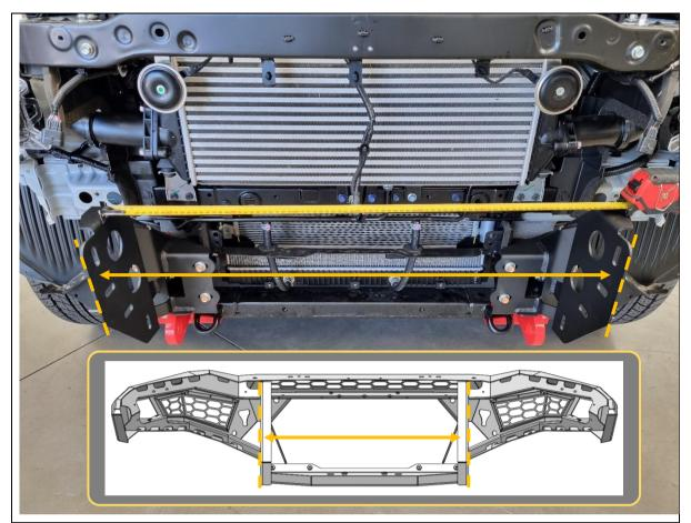
61. Measure the distance between the outside faces of uprights on bar using tape measure. Write distance below for reference if required.
