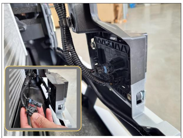
26. Unplug 2x connectors and unclip the wiring harness behind the adaptive cruise control (ACC) radar in the middle of the bumper.
