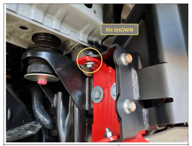
165. Loosen the upper rear M10x30 hex bolts on the impact assemblies in preparation for fitting side underpanels.
