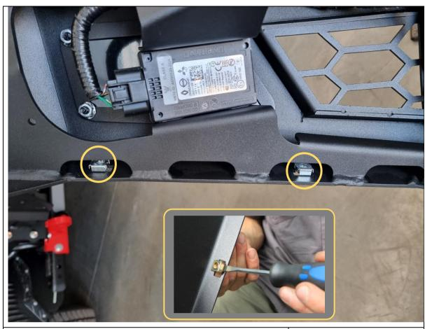
104. Fit 10x M6 cage nuts into the rectangular slots on the bottom of the bar wing (5x per side).
