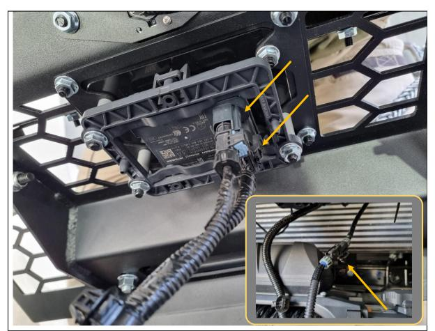
158. Hold the mesh fairlead mount up near the bar and reconnect the 2x radar harnesses and 1x camera harness.
