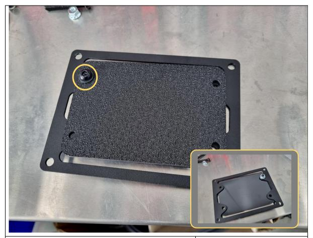
147. Fit the plastic ACC radar cover panel to the P-0381 radar mount plate and loosely secure with 1x M6x16 black button head bolt, black washer and flange nut in the top left corner.
