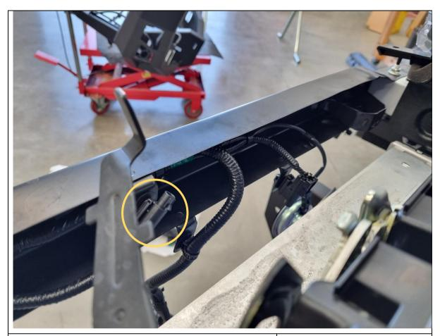
68. Unclip the camera harness from the upper body frame and let cable hang down.
