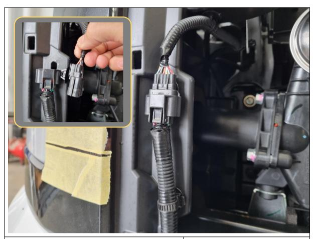
27. Unplug and unclip the 2x bumper harness connectors (left and right), located on the bumper near the inside face of the headlights.
