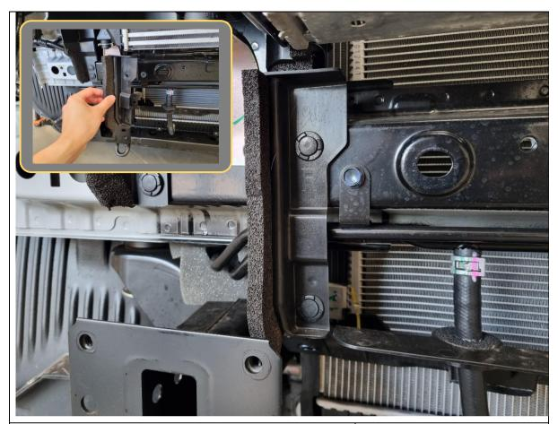
48. Remove 2x plastic push clips securing the mini air dam above the chassis rail. Remove and discard on both sides.
