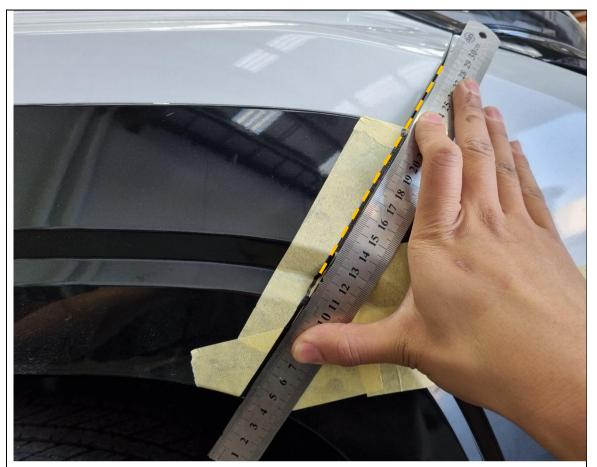
6. **GSR trim level only.** Mark out a straight line extending from the quarter panel edge onto the flare.
