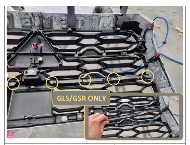
125. **GLS/GSR only.** Remove 8x Phillips pan head screws holding the 2x metal support brackets inside the grille and set aside. Do not discard.
