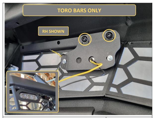
76. Fit the indicators and brackets to the inside of the bullbar wing mesh, using 2x M6x16 black button head bolts, black washers and flange nuts. The indicator should sit flush and central to the cutout in the mesh. Do this for both indicators.
