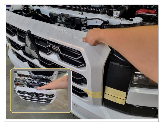
13. Pull outwards from the top and release the clips holding the grille. Set aside for later.
