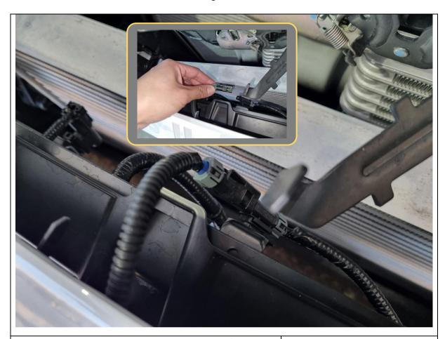
11. Disconnect the camera plug on the inside of the grille.
