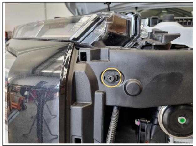
32. Remove 2x 10mm hex bolts on the front face of the bumper near the headlights. Do not discard fasteners.
