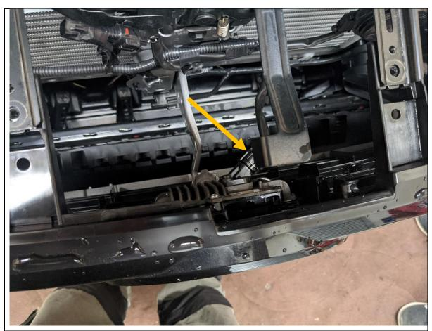
5. Unplug the radar sensor module wiring connector, located on the back of the Toyota Badge / sensor.
