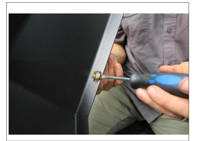
80. Insert cage nuts to square slots in bottom of wings. Seat cage nut against one edge of slot then push other edge in with flat bladed screwdriver.
