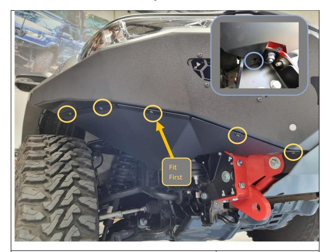
110. Fit side under panels to bar and secure with 4x M6x16 Button head bolts and M6 Flat washers, into M6 cage nuts fitted earlier.
