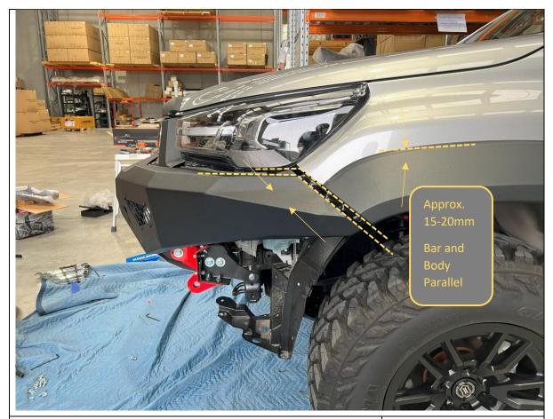
85. Align the bar with the body. Aim for 15-20mm clearance between the wing and body.
