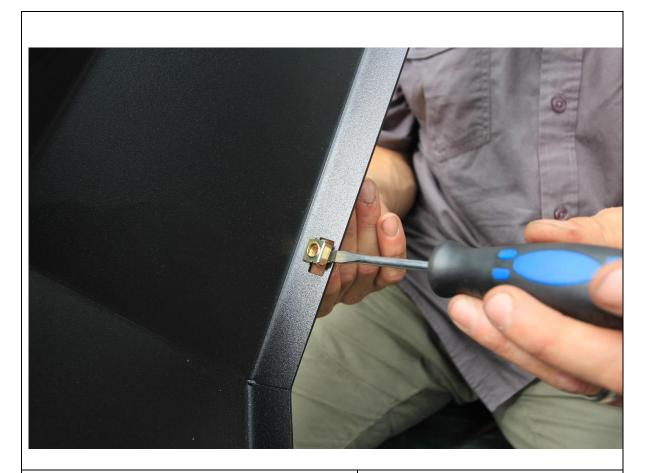
78. Insert cage nuts to square slots in bottom of wings. Seat cage nut against one edge of slot then push other edge in with flat bladed screwdriver.
