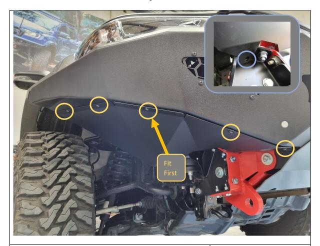
108. Fit side under panels to bar and secure with 4x M6x16 Button head bolts and M6 Flat washers, into M6 cage nuts fitted earlier.
