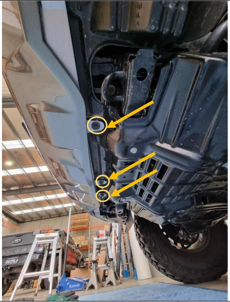
Remove the 3x Factory Screws securing bottom center section of bumper to inner wheel arch liner. Use 10mm socket / spanner.
