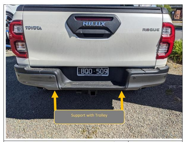
1. Before beginning work, support the factory rear bar / tow bar using lift trolley or jack.
