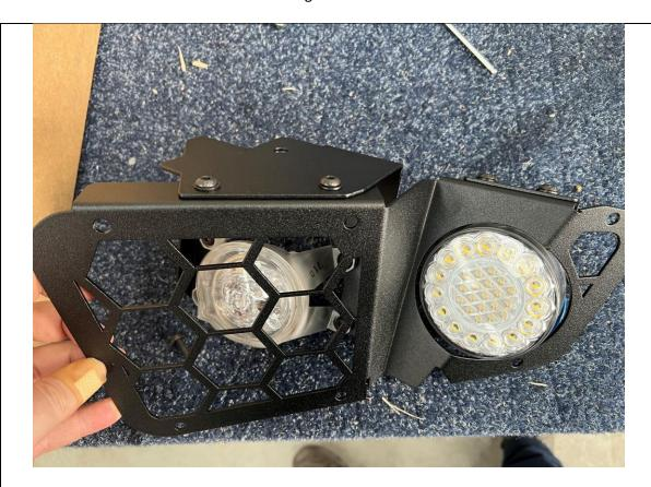
83. Fit the fog/indicator lamp brackets, to the light mesh panels using 4x M6x16 Button head bolts. The bracket should sit on TOP of the light mesh as shown.
