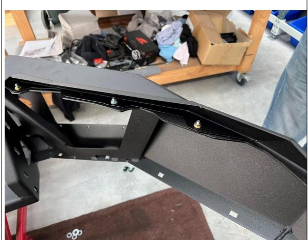
65. Fit the headlight infill panels to the top of the bar, using supplied M5 Hardware. Leave finger tight at this stage.
