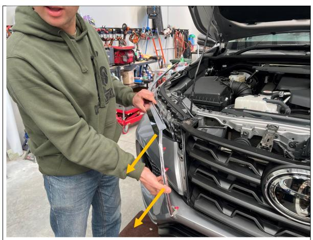
11. Remove the chrome headlight trim panels by carefully prying then pulling in a forward direction to release clips holding.
