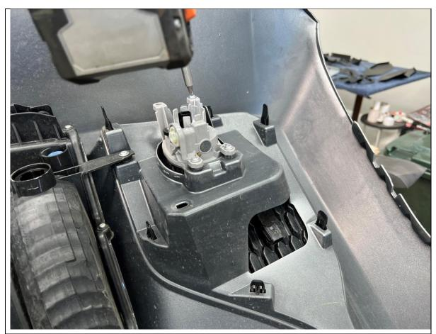
47. Remove the 3x Screws securing the fog lights to the bumper, then remove the fog light from the bumper
