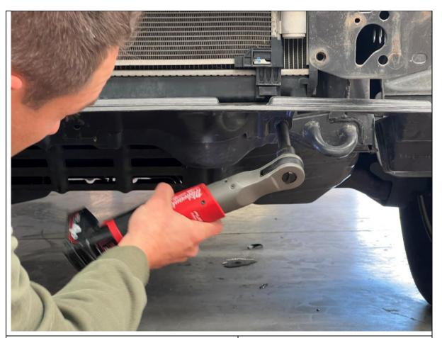
28. Remove the lower splashguard by removing the 10mm head bolts securing to vehicle
