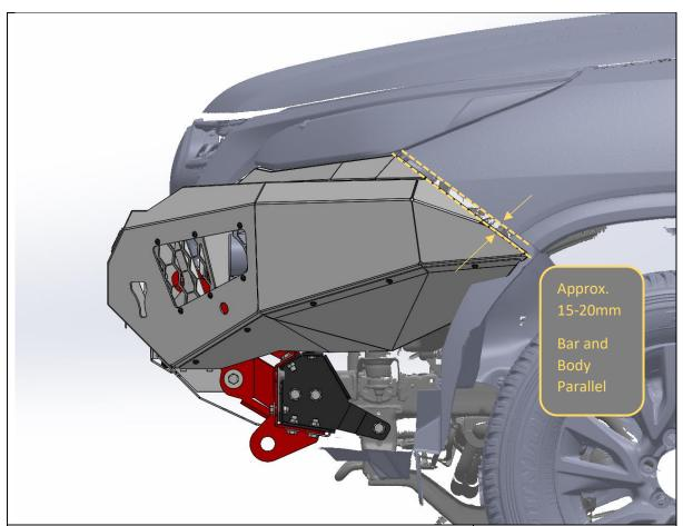
69. Align the bar with the body. Aim for 15-20mm clearance between the wing and body.
