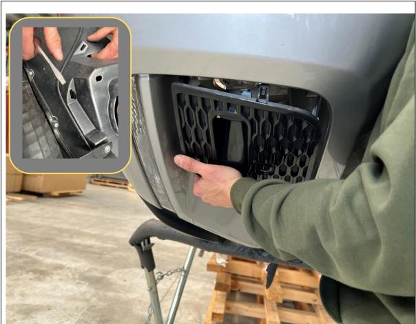
48. Remove the gloss plastic trim panel from the main bumper assembly by releasing clips securing, to gain better access to parking sensor housing.
