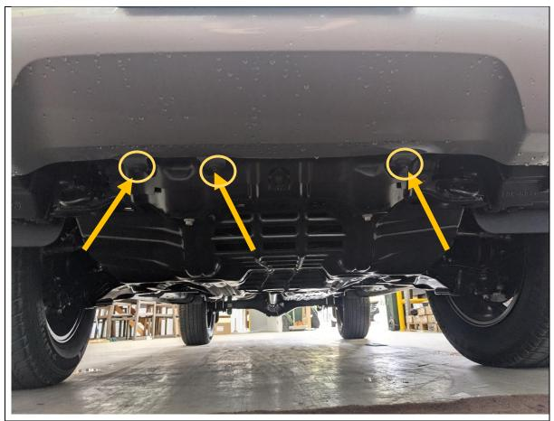
10. Remove the 3x 10mm head Screws securing bottom center section of bumper to inner wheel arch liner.
