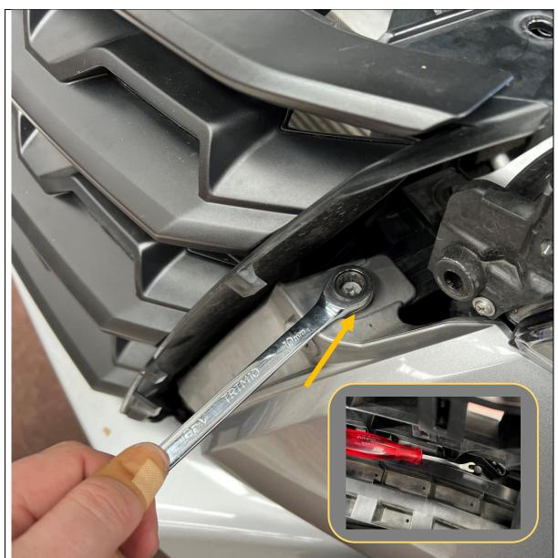
12. Remove the 2x 10mm Head/Phillips screws securing the bumper to crossmember.
