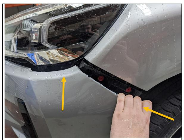
14. Remove the bumper. Start by pulling from the outside where the bumper meets the wheel arch and work towards the center from both sides.
