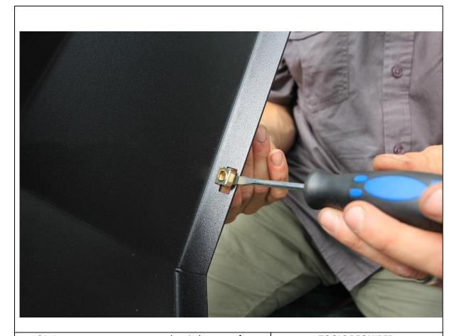
64. Insert cage nuts to square slots in bottom of wings. Seat cage nut against one edge of slot then push other edge in with flat bladed screwdriver.
