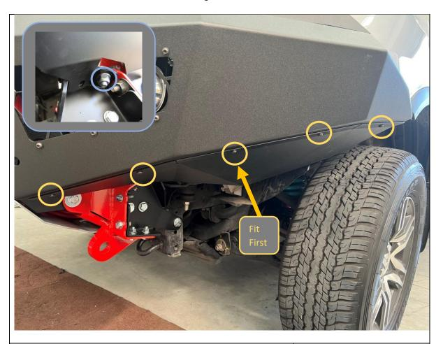
100. Fit side under panels to bar and secure with 4x M6x16 Button head bolts and M6 Flat washers, into M6 cage nuts fitted earlier.
