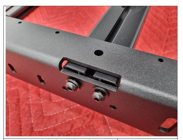
2. Bring the rack side in line with the cross bar extrusions and loosely secure each extrusion end with 2x M8x20 black button head bolts and black washers through the pre-threaded holes on the side.
