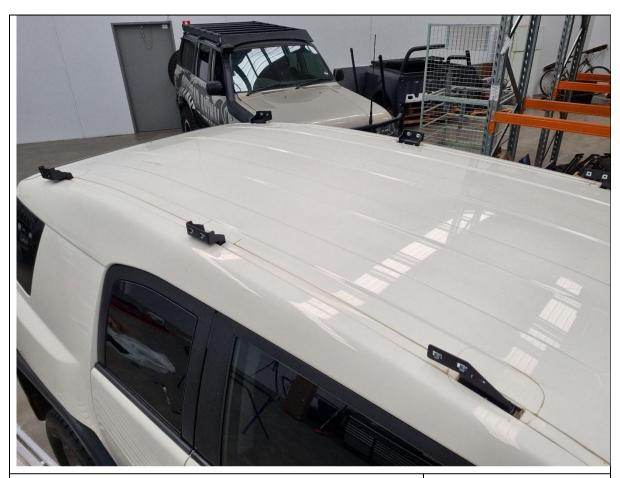
44. Image showing all 6x mounting brackets in position. Do not fully tighten bolts yet.
