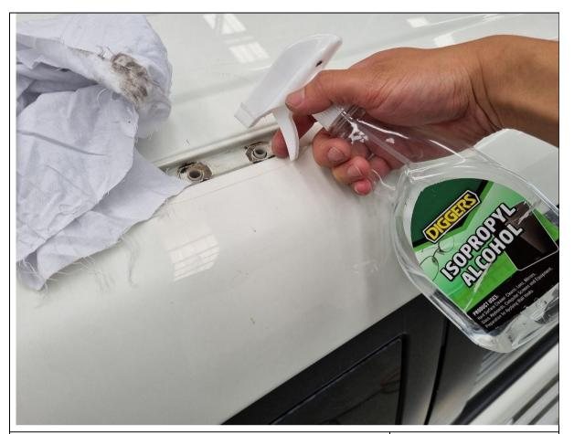
35. Using isopropyl alcohol and a clean workshop rag, clean away all the dirt from the roof gutters.
