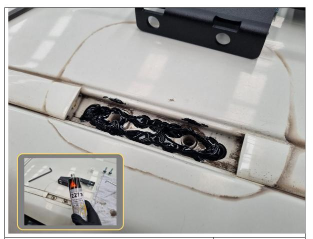
40. Apply a generous amount of automotive grade sealant (Offroad Animal recommends Sikaflex 227) around the 2x holes at each of the 6x mounting locations.
