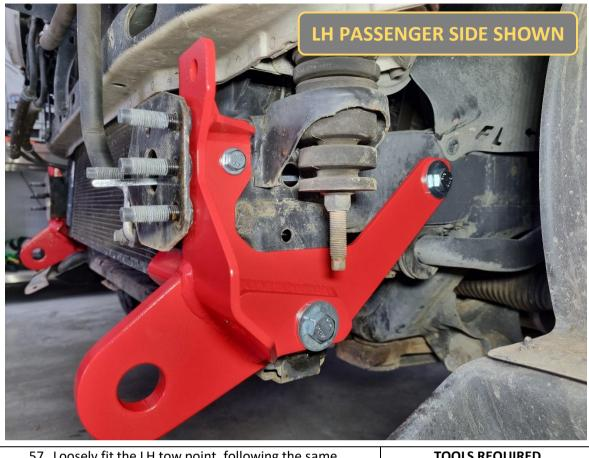
57. Loosely fit the LH tow point, following the same procedure as the RH tow point. This side is easier without the power steering lines and washer bottle getting in the way.
