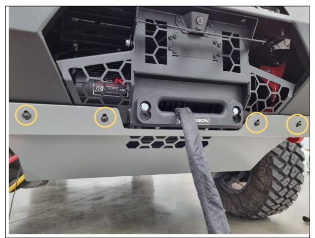
150. Fit the centre bash plate to the bar using 4x M8x20 black button bolts and flat washers.
