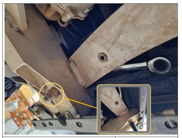
144. Additional reinforcement is required for the bash plate. Remove 2x 18mm hex nuts (1x per side) on the underside of the frame. Use an 18mm spanner to reach in access the bolt head on top of the frame member.
