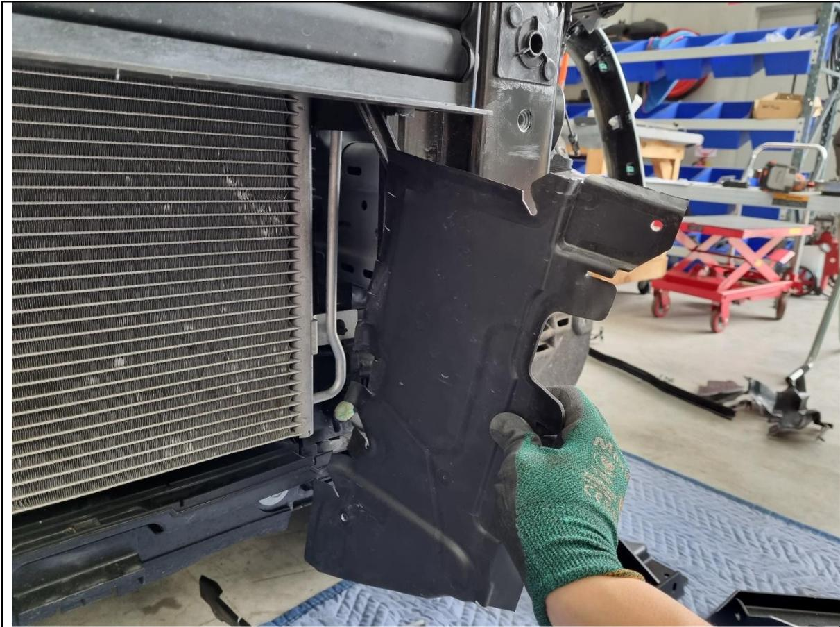
33. Unclip and remove the lower air dams with a flat head screwdriver or trim tool.
