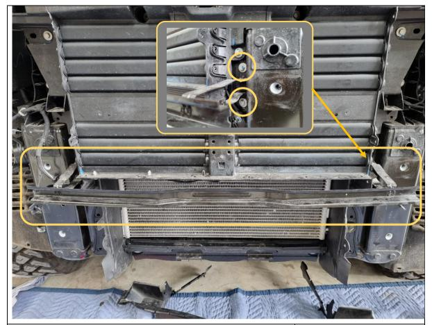
32. Remove the steel cross beam by removing the 4x 10mm hex head bolts securing it to the body (see inset).
