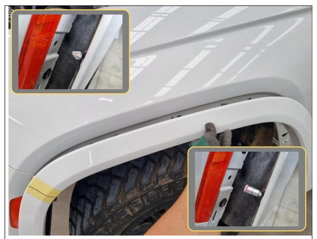
18. Pull and release the clips retaining the flare to the bumper + quarter panel.
