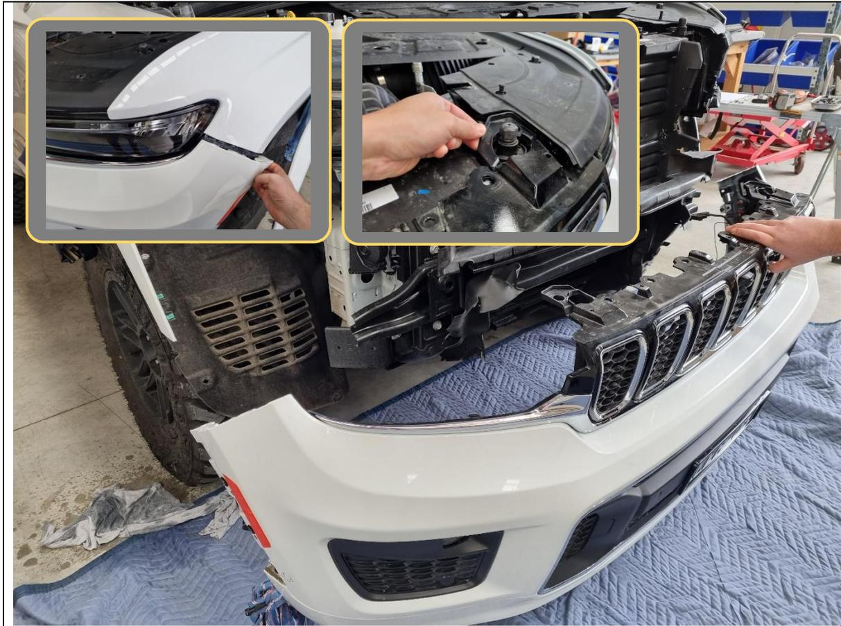
23. Remove the bumper by releasing the clips on either side and lifting the top flap of the grille over the bonnet rubber stops.
