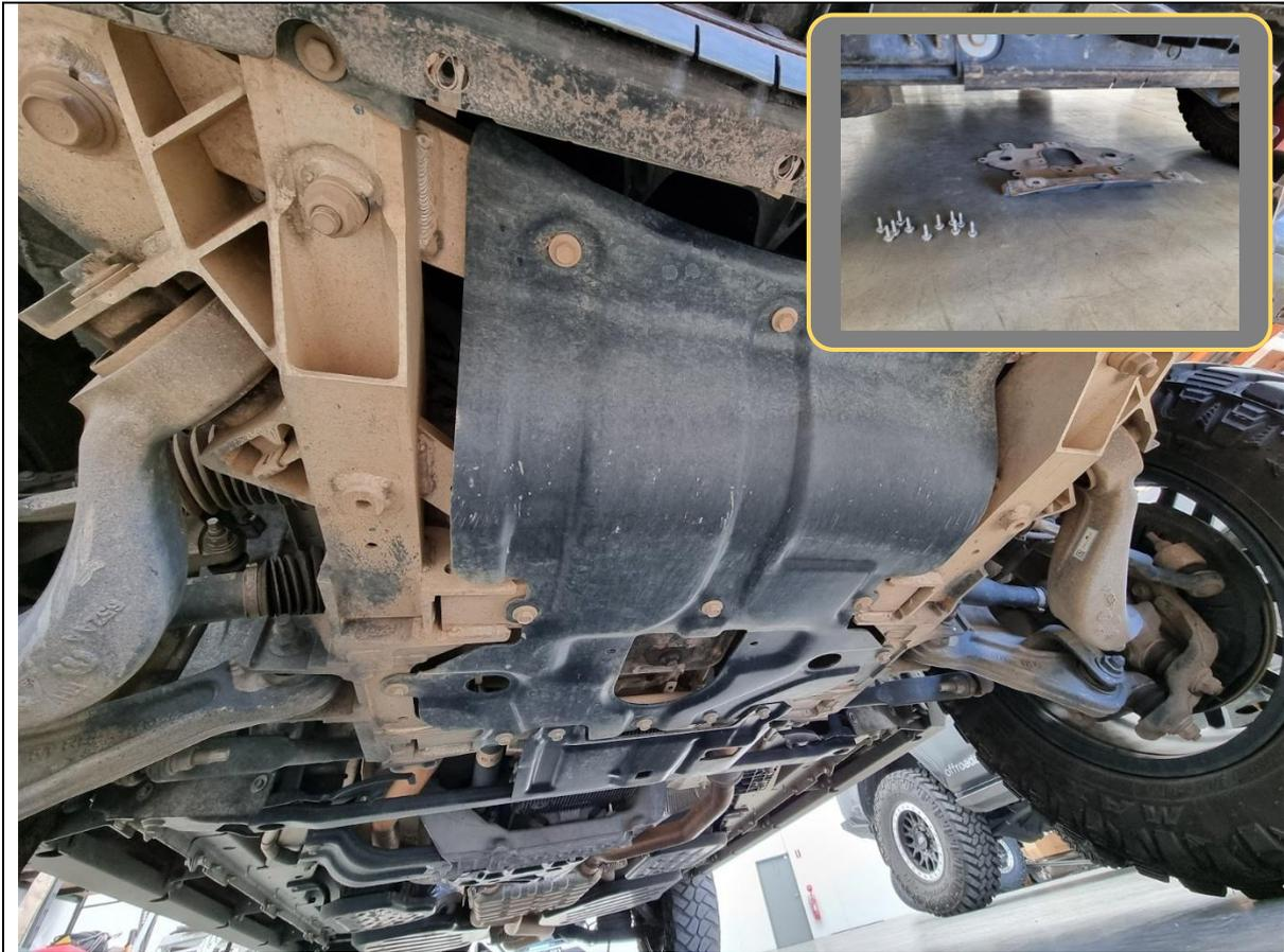
6. If equipped, remove 11x 13mm hex head bolts holding the metal skid plate underneath the vehicle and set aside.
