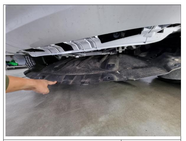
9. If equipped, remove 10mm hex bolts and plastic push rivets securing the felt undertray liner to the vehicle. Either fully remove it and set aside; or remove enough fasteners to get access to the front underside of vehicle.
