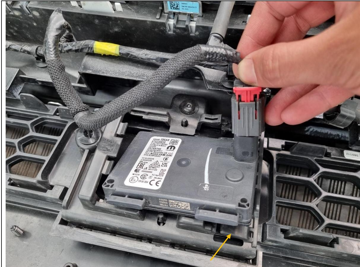
70. Next, note down the orientation of the adaptive cruise control (ACC) radar.
