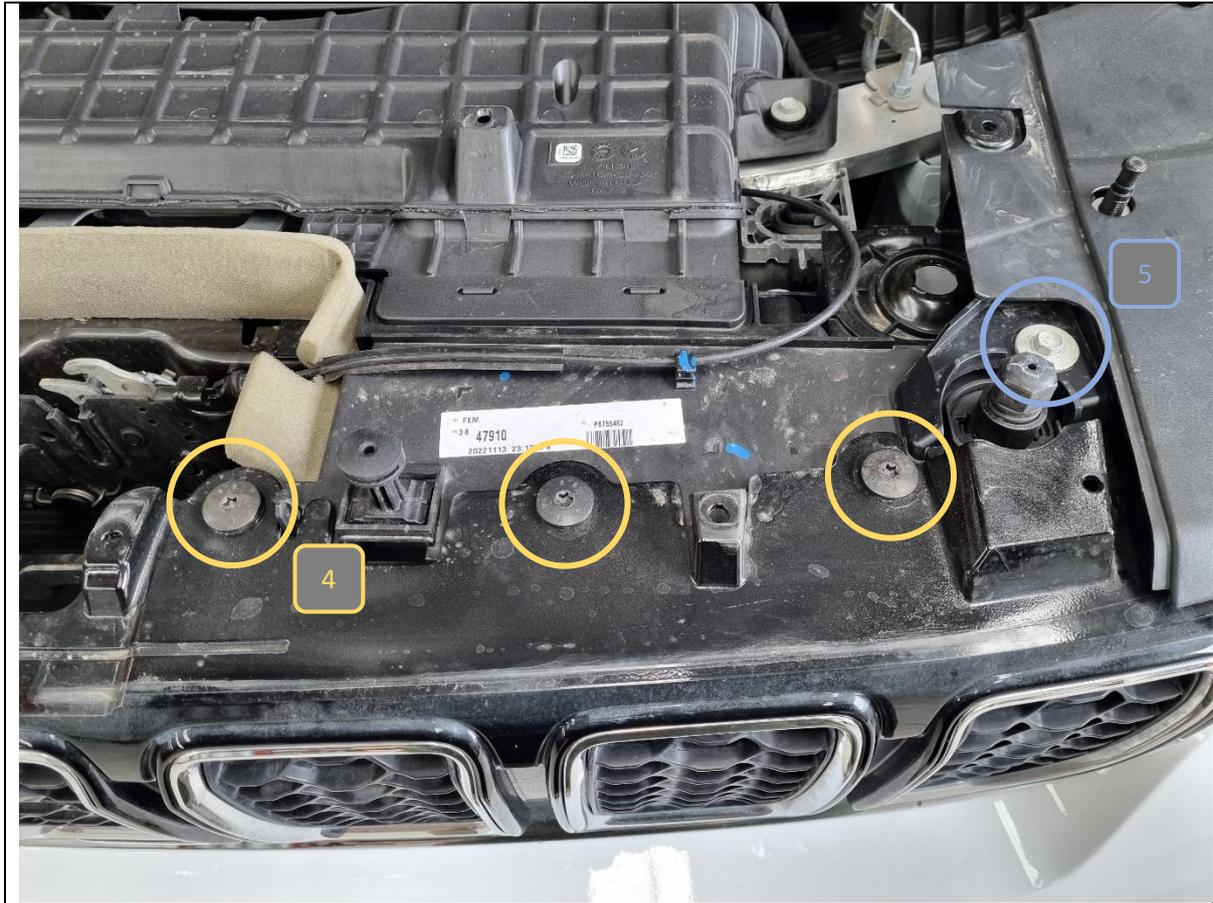
4. Remove 6x T40 Torx screws from the top of the grille.
