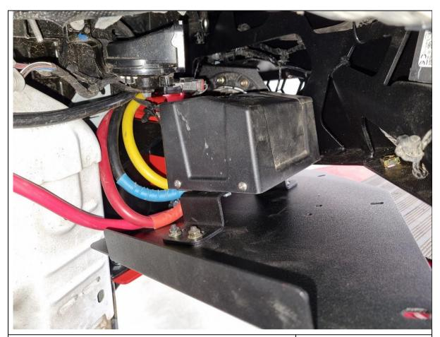
157. Secure the control box and relocation bracket to the inside of the side underpanel with 4x M6x16 black button head bolts, washers and flange nuts.
