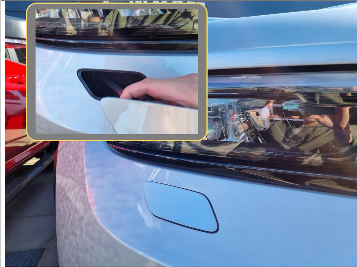
22. If headlight washers are equipped, pull out the plastic cover cap and unclip it from the plastic washer stem.
