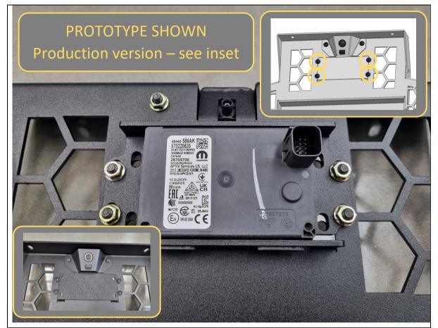
73. Fit the centre radar and bracket to the inside of the mesh fairlead.
