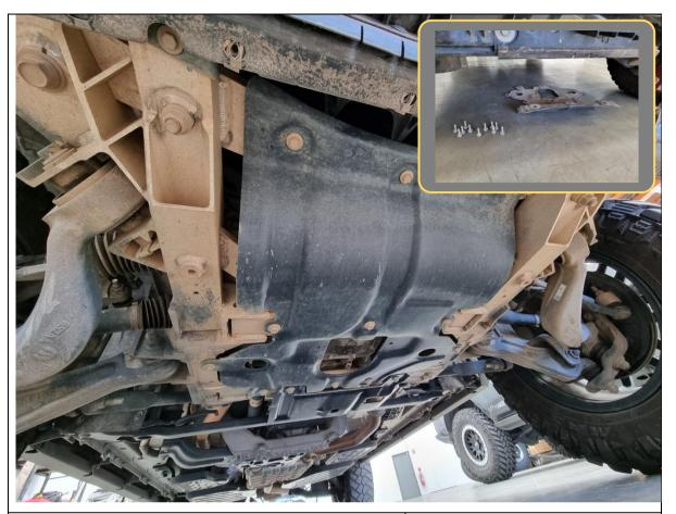
6. If equipped, remove 11x 13mm hex head bolts holding the metal skid plate underneath the vehicle and set aside.
