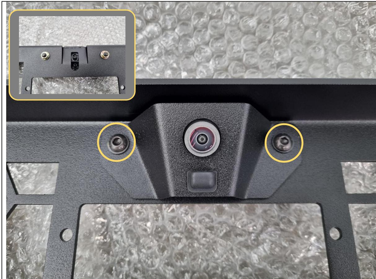
69. Bolt the relocation bracket (with camera clamped in between) to the mesh fairlead panel using 2x M6x16 black button head bolts, black washers and flange nuts.
