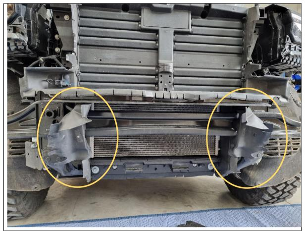
25. Unclip and remove the air dams with a flat head screwdriver or trim tool.
