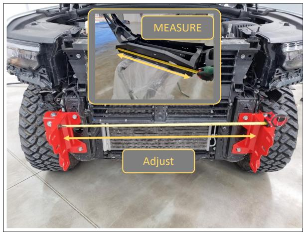
45. Measure the distance between the outside faces of the uprights inside the Predator bar using a tape measure. Write distance below for reference if required.
