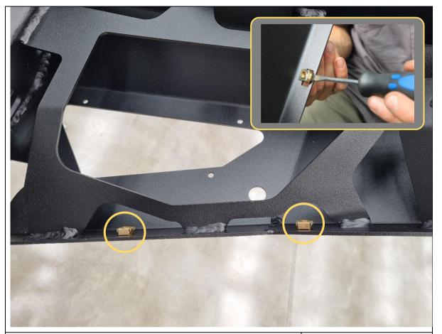
57. Fit 5x M6 cage nuts each side into the rectangular slots on the bottom of the bar wing.
