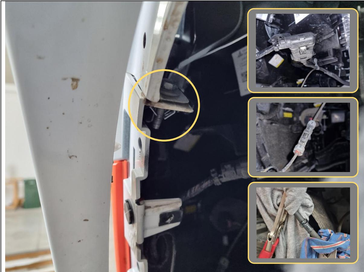
20. On both sides, remove the 10mm hex head bolt securing the bumper to the quarter panel (fender).
