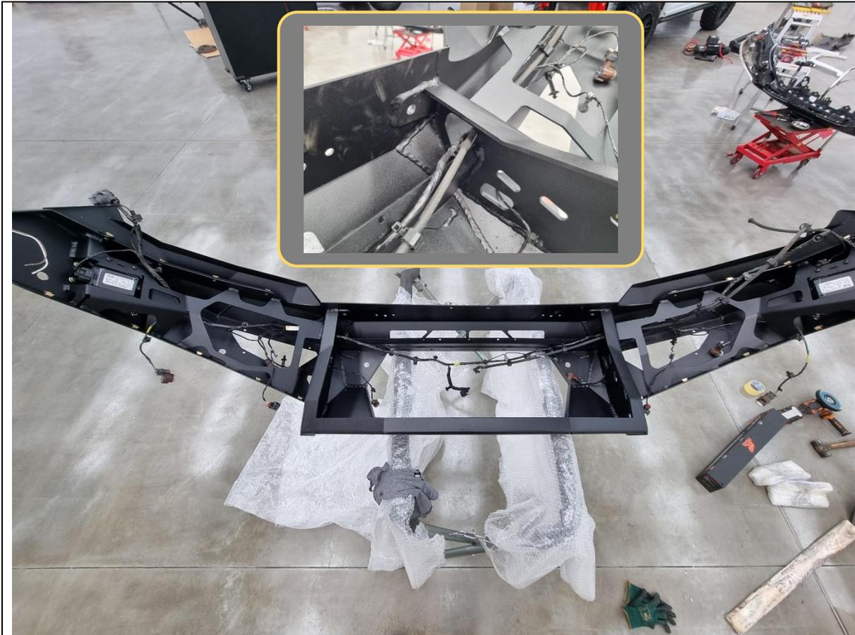
90. Transfer the entire harness and parking sensors across to the bar, in the same orientation as the original bumper.
