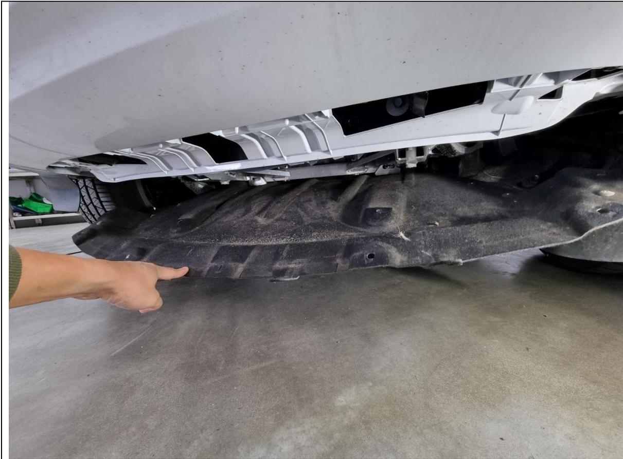
9. If equipped, remove 10mm hex bolts and plastic push rivets securing the felt undertray liner to the vehicle. Either fully remove it and set aside; or remove enough fasteners to get access to the front underside of vehicle.
