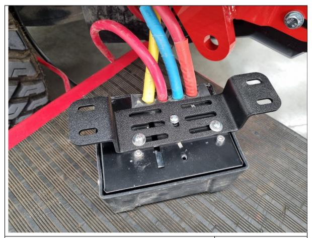
156. If relocating a winch control box, use the supplied relocation bracket and bolt the control box to it (fasteners not supplied).
