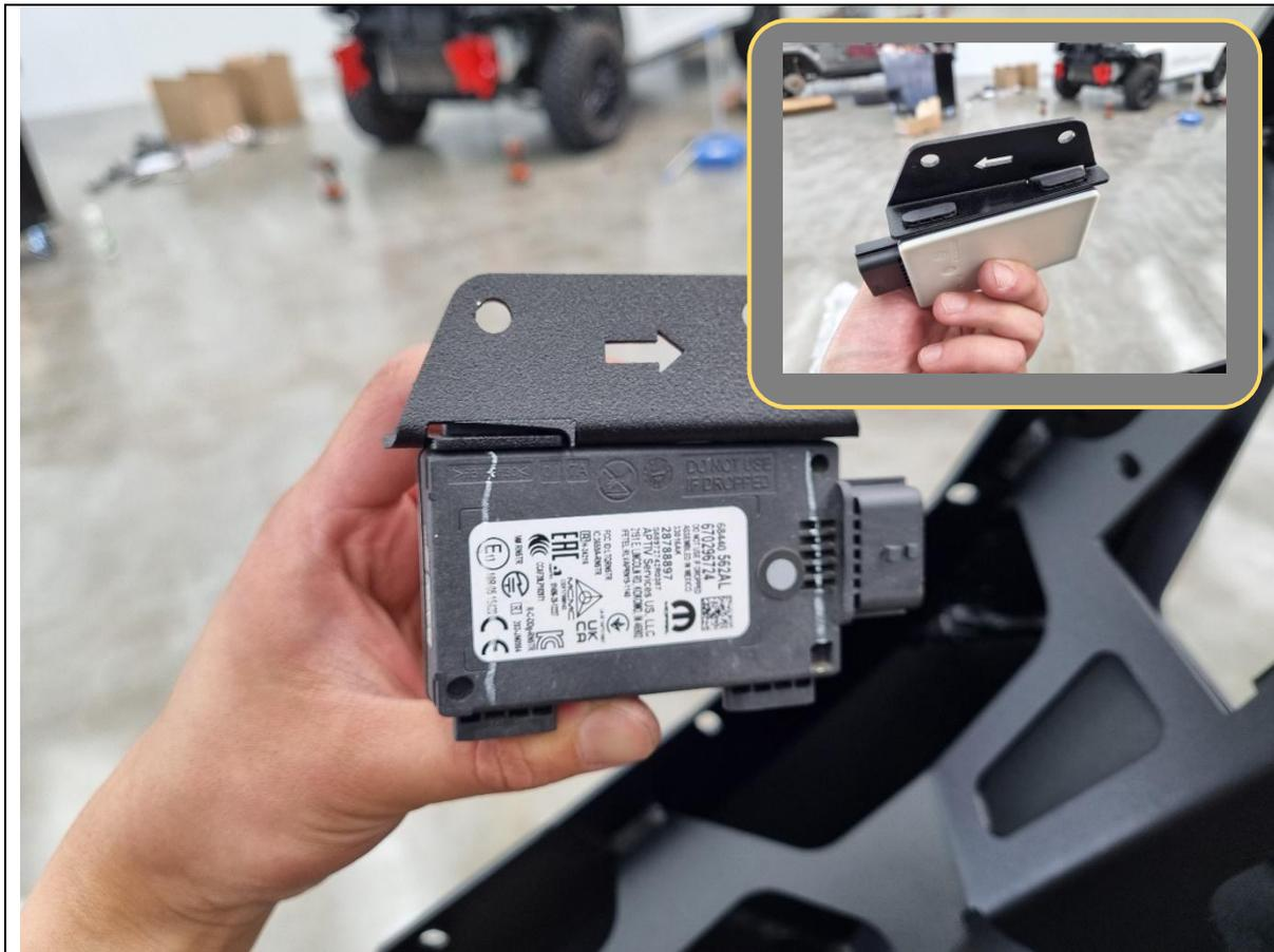
78. Clip the intersection collision assist radar into the side radar bracket with the plug pointing in the same direction as the arrow cutout in the bracket.
