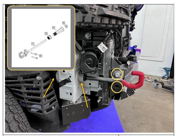
26. If factory tow hooks are equipped, remove them by undoing the 2x 16mm hex head bolts on each side, then remove the large nuts with a large adjustable wrench (see inset for Jeep parts breakdown).
