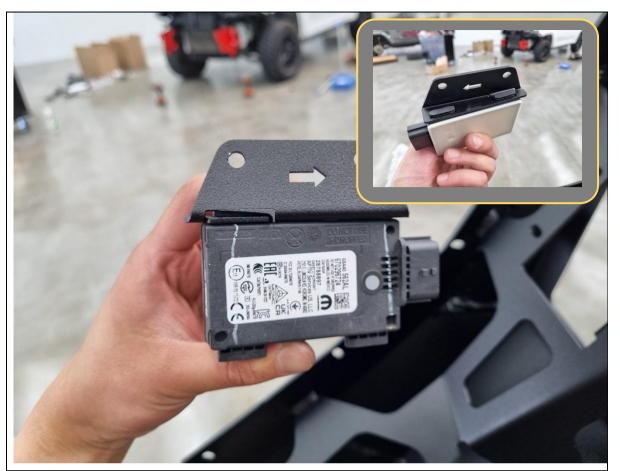
78. Clip the intersection collision assist radar into the side radar bracket with the plug pointing in the same direction as the arrow cutout in the bracket.
