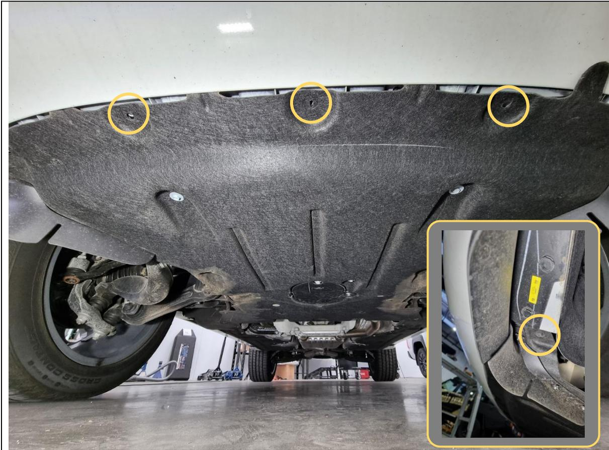
7. If equipped, remove 5x 8mm hex head bolts holding the front of the felt undertray liner to the bumper.
