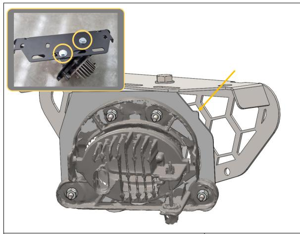
105. Secure the fog light and bracket to the light cover mesh panel, using 2x M8x12 hex head bolts, flat washers and flange nuts.
