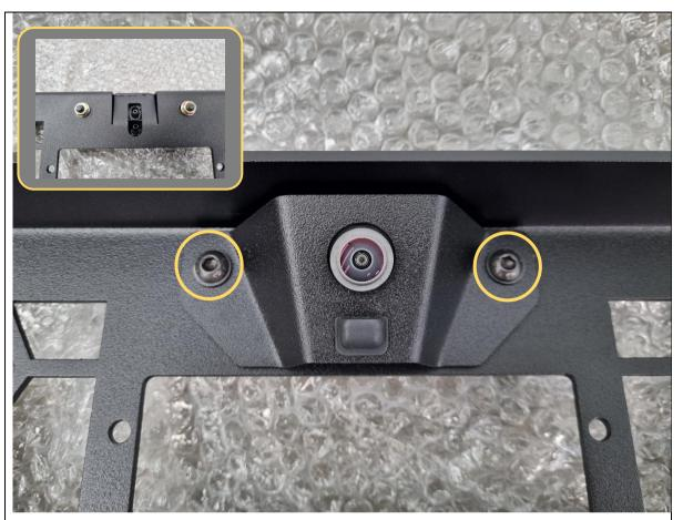
69. Bolt the relocation bracket (with camera clamped in between) to the mesh fairlead panel using 2x M6x16 black button head bolts, black washers and flange nuts.
