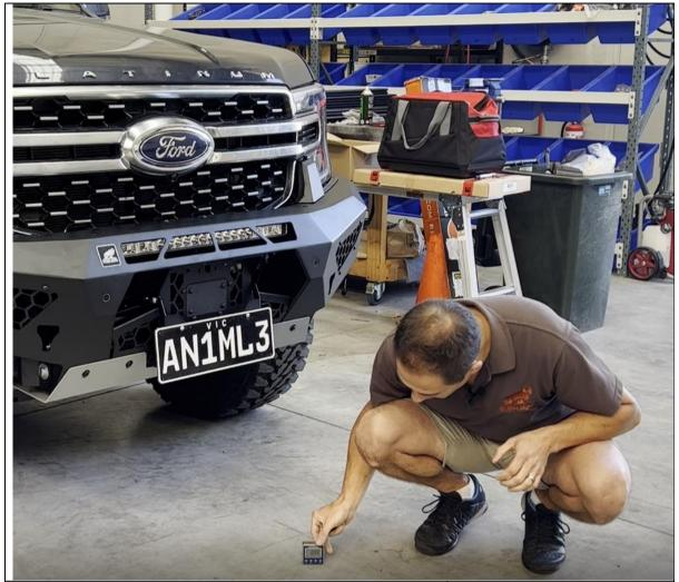
2. Zero the digital angle gauge on a flat reference surface
