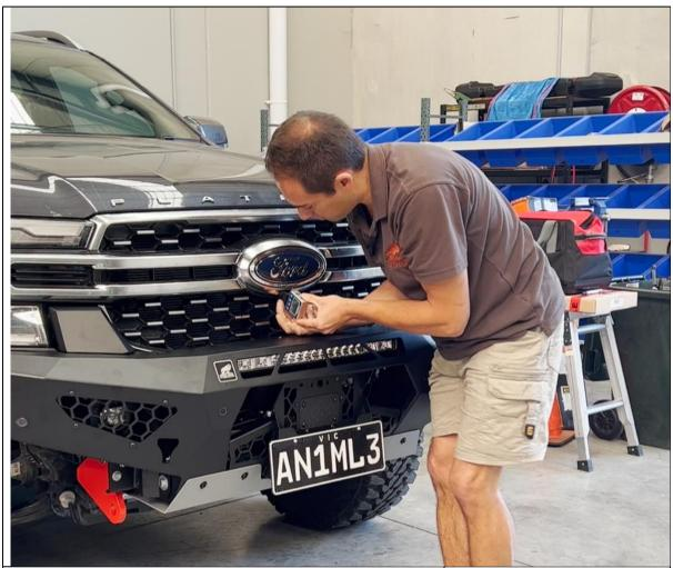
3. With the assistance of a straight edge tool, measure the angle of the front camera and record it below
