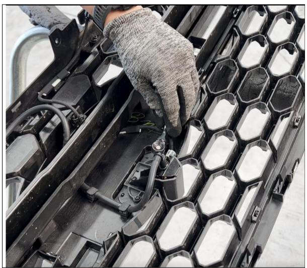
6. Remove the camera housing from the grille, by removing the 3x T20 Screws securing it.
