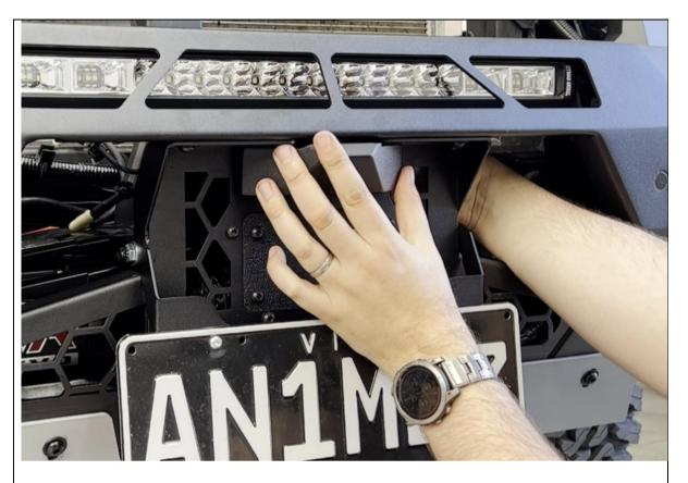
24. Fit the cover panel over the camera bracket assembly, securing with M5 Screws from behind, into the threaded inserts in the cover panel.
