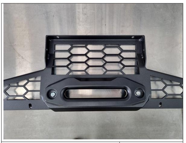
87. If required, fit the winch fairlead to the centre mesh fairlead mount using M10 or 3/8" fasteners supplied with the winch. This bar is only compatible with hawse type fairleads.
