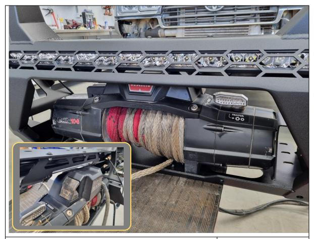
54. If fitting a winch with an integrated top mount control box and the vehicle is equipped with an aftermarket intercooler, fit the winch onto the cradle in the bar now.
