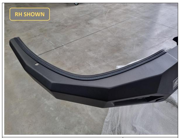
42. Fit the 2x supplied of top bulb pinch weld rubber to each wing on the bullbar, as shown.
