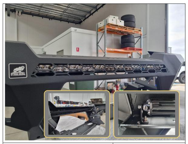
34. If fitting an integrated light bar, do so now from the back.
