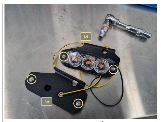
49. Fit the indicator repeater lamps to the indicator brackets, using M3x12 pan head screws, washers, nuts and the adhesive backing included with the lamp module.
