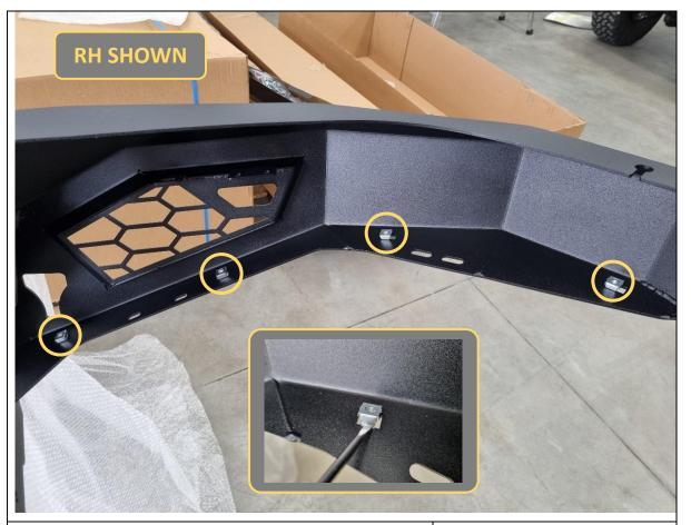
39. Fit 8x M6 cage nuts into the rectangular slots on the bottom of the bar wing (4x per side).
