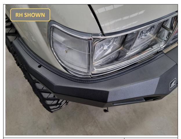
61. Shuffle the bar left/right on the vehicle so that the gapping to the fenders is even and symmetric.
