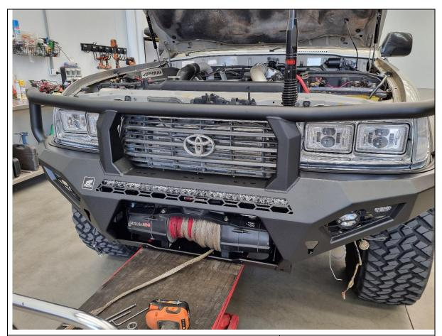
58. With assistance, either from another person, or a lifting trolley, lift and slide the bar onto the chassis.
