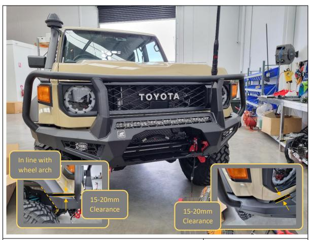
52. With assistance, from another person, align the bar with the edges of the vehicle. The bar should sit symmetric left/right on the vehicle.
