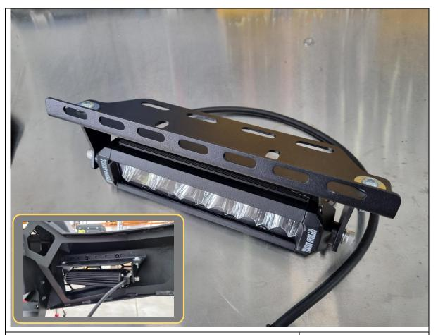
43. If not fitting factory fog lights, there is the option to fit Offroad Animal Halo Fog Lights (part no. ORA-ALO-M-2) with B-1185 mounting brackets (purchased separately), or fit 8" light bars or cube lights using the supplied B-1169 universal wing mesh light brackets (shown).
