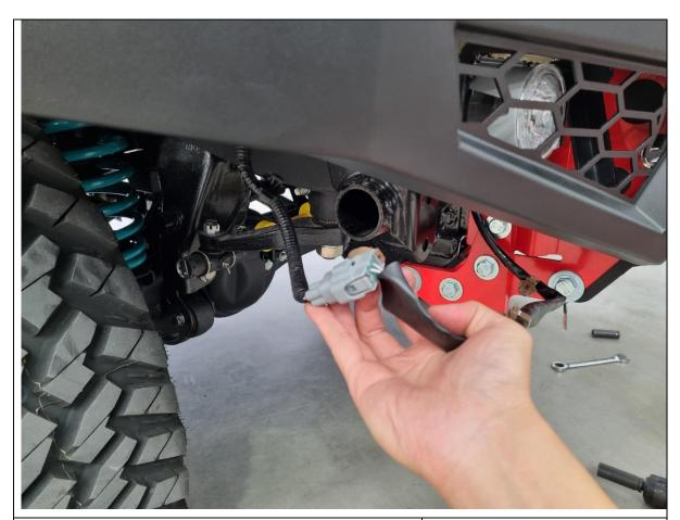
54. Reconnect the fog light and bumper loom to the vehicle.
