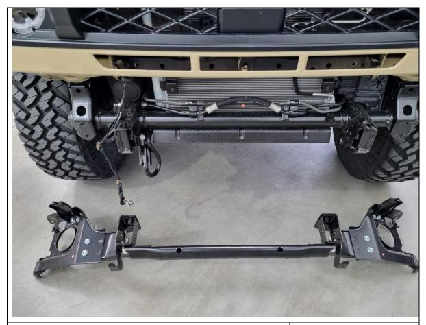
17. Remove the main impact bar from the vehicle. TOOLS REQUIRED
