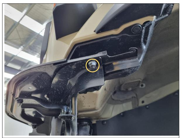
9. Remove 1x 12mm hex nut on the bottom of the metal top panel, per side.
