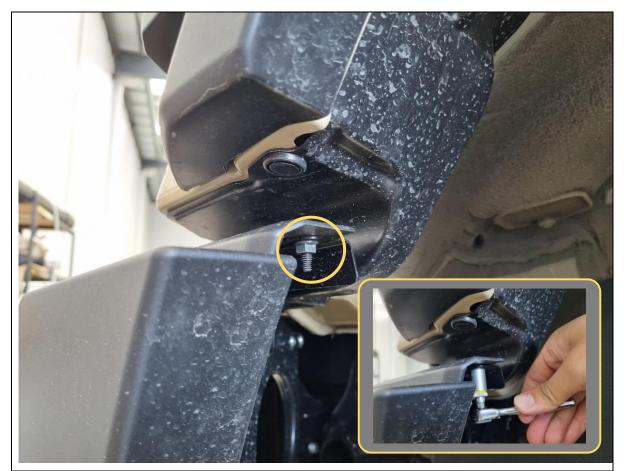
2. Remove 1x 10mm hex nut on the outer tip of the plastic bumper, per side.
