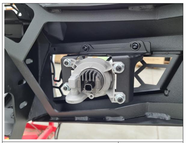
40. Fit the fog light and bracket to the inside of the bullbar and secure with 2x M6x16 black button head bolts and black flat washers, each.
