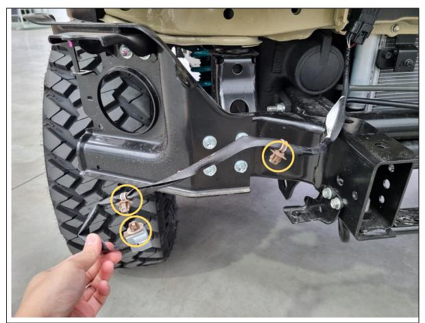
14. Unclip the bumper harness from the main impact bar.
