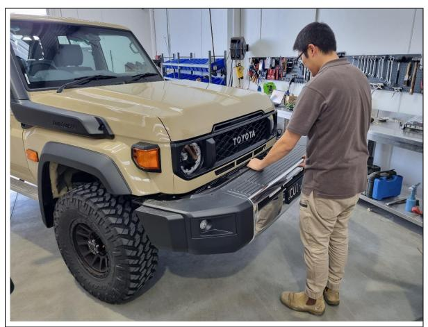
7. The bumper is now fully loose. Pull outwards and remove from vehicle.
