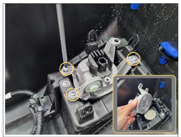
36. Remove 3x Phillips head screws holding each fog light and set aside.
