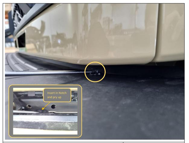
3. Remove 5x plastic push clips along the top of the plastic bumper. 3x of them are found through the opening in the grille fascia.
