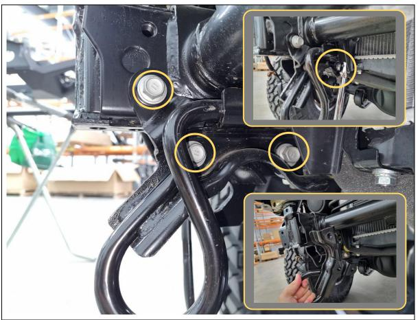
20. Remove the 3x 14mm hex bolts holding the factory tow
