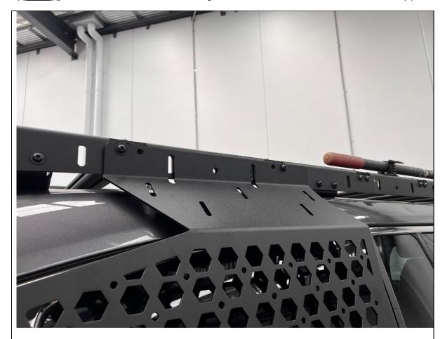
3. Loosely re-fit two screws through the window panel then into the roof rack holding the panel up.
