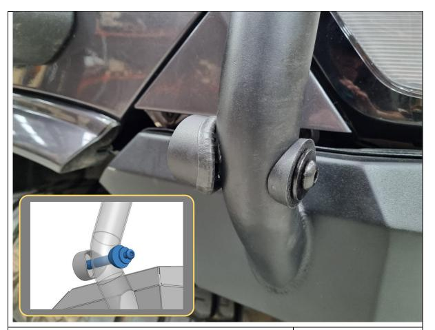
17. Loosely position the spigot with the Toro bar and hold in place with 1x M10x100 black button head, flat washer, nylon saddle washer and crush tube, through the 18mm drilled hole in the bar.
