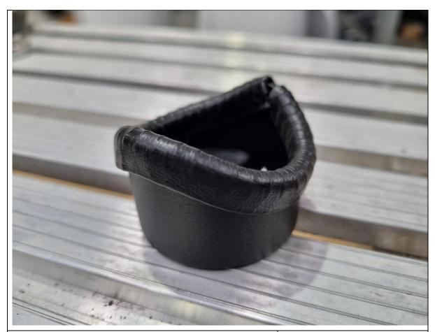
16. Fit supplied pinch weld around the curved edge of the spigot. Trim with side cutters if oversized.
