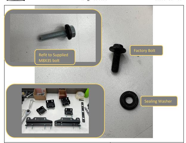
33. Remove the rubber sealing washers and rings from the factory fasteners for re-fitment to supplied bolts.
