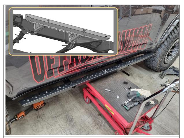
6. Using either another person or a lifting trolley, present the rock slider up against the vehicle. The U-shape brackets will wrap around the chassis rail.
