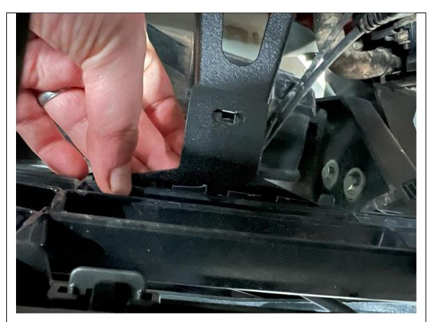
84. Fit the secondary grille support brackets to the underside of the grille, using the tape pads, such that the bracket aligns with the slotted end of the primary support bracket.
